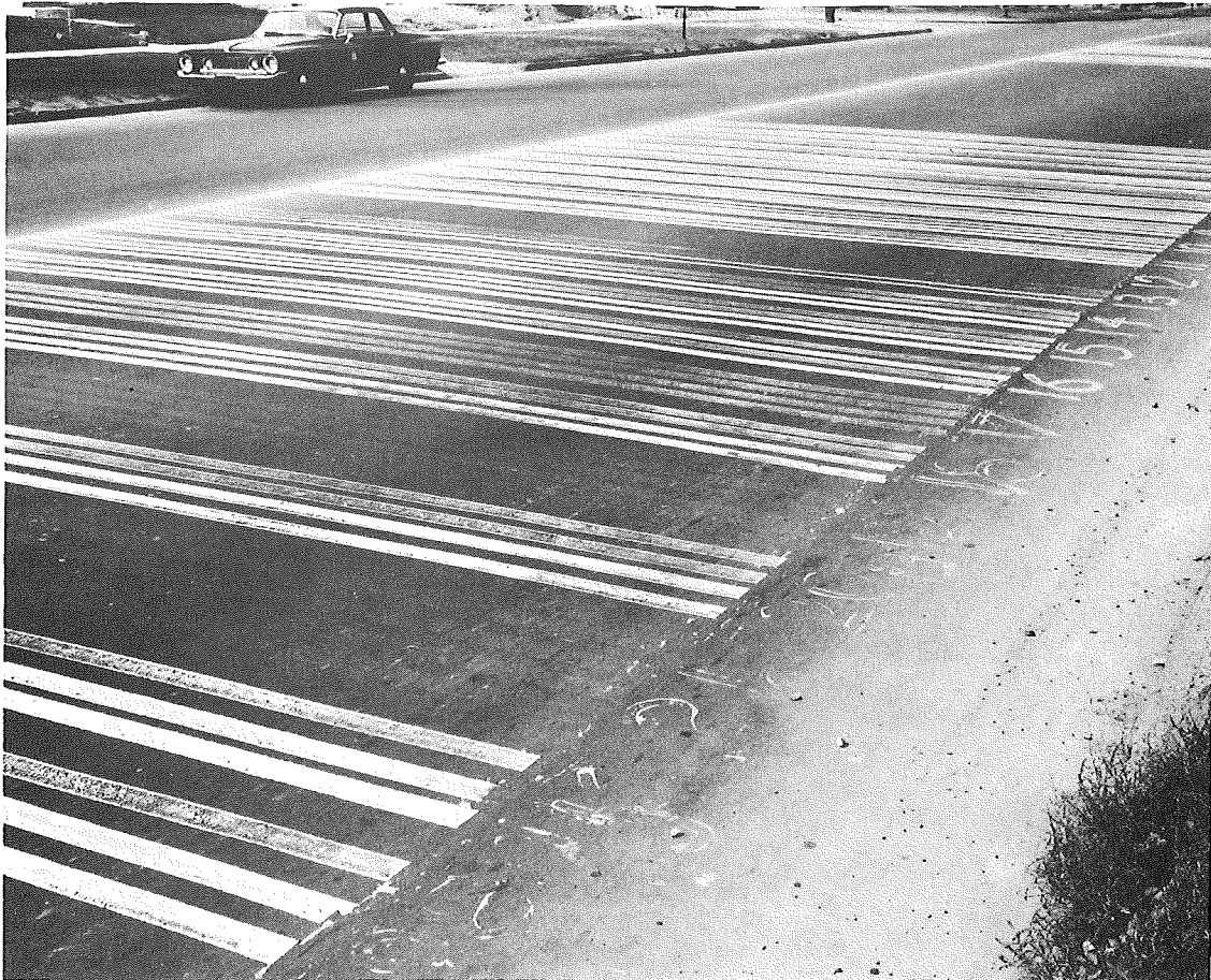
Figure 3. Terminal appearance of white stripes after eight months of service in Detroit; MSHD control stripes in triplicate in foreground, Detroit's quadruplicate stripes in background.
