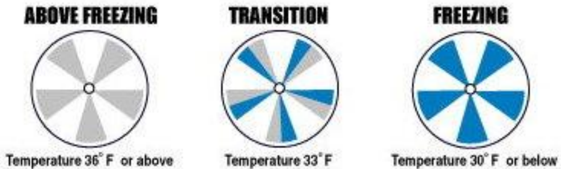
Figure 12. Change in the BlueStar System display as temperature falls below freezing.
