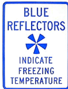
Figure 17. Sample road sign with instructions on how to read the Bluestar System display.
