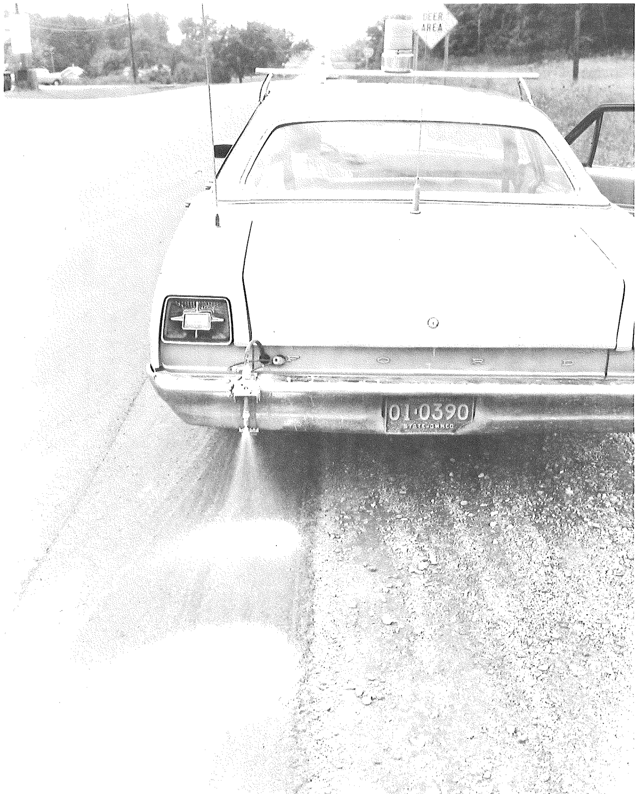
Photograph 3 - Middle vehicle operator applying two paint marks to designate a zone ending.
