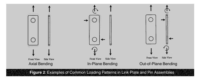
The variables that affect the stress magnitudes in a link plate are truck weights, impact factor, lateral distribution of the truck loads, length of the span, redundancy of beams, angle of crossing, and corrosion in the link plate. Additional variables that affect the fatigue life of the link plate are average daily truck traffic (ADTT), number of traffic lanes, percentage of trucks in a given lane, and number of stress occurrences per truck passage.
