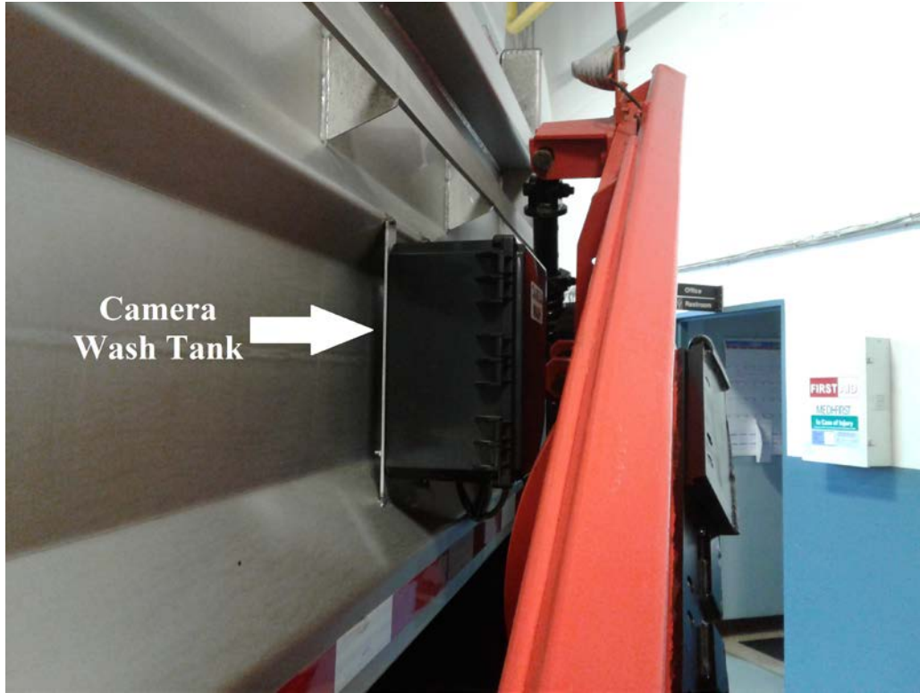
Figure 7-1 Camera Wash Tank
