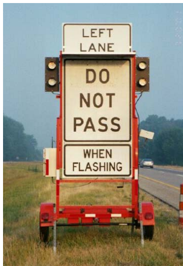
Figure 3. Dynamic LMTCS Sign and Trailer Used in Michigan
