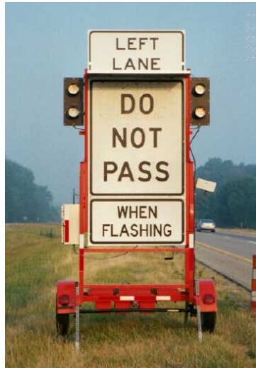
Figure ES-1. Dynamic LMTCS Sign and Trailer Used in Michigan
