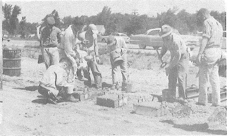
Figure 14. Concrete Consistency Was Measured by the Ball Penetration Method and the Same Concrete Used for a Unit Weight Determination.
