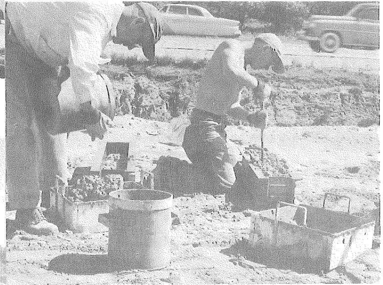
Figure 15. Following the Unit Weight Determination, the Concrete Was Used to Mold One Flexural Test Beam From Each Pan.
