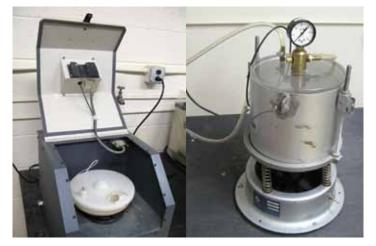
Researchers tested two approaches to measuring specific gravity. The automated SSDetect method (left) uses infrared technology to test fine aggregates; the vacuum saturation apparatus (right) for testing coarse aggregates removes trapped air and replaces any air voids with water.
