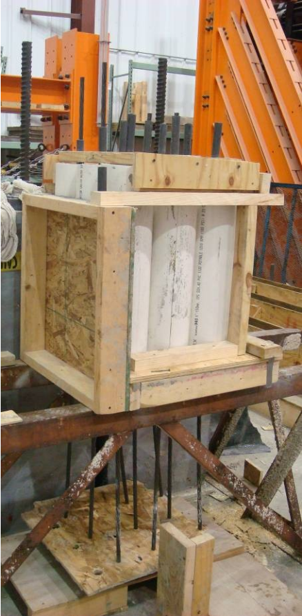
Figure 16 Form Work of Pull-out Cylinders
