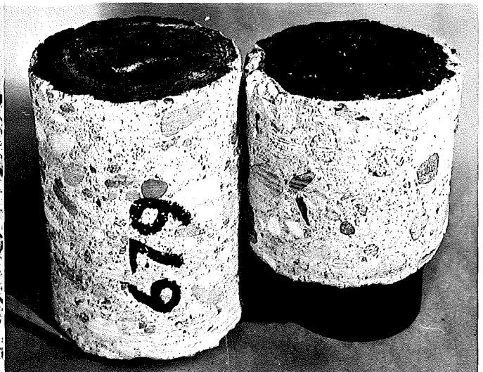
FIGURE 19. ANOTHER VIEW OF SAME CORE SPECIMEN, BASE ON LEFT, CAP ON RIGHT. NOTE THAT BITUMINOUS MATERIAL STICKS TO BOTH OLD AND NEW CONCRETE.
