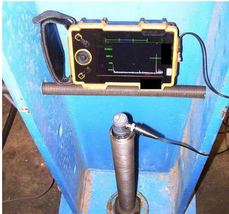
Figure 1.18 - An anchor bolt being inspected with a straight-beam ultrasonic transducer. https://fhwaapps.fhwa.dot.gov/ndep/DisplayTechnology.aspx?tech_id=6
