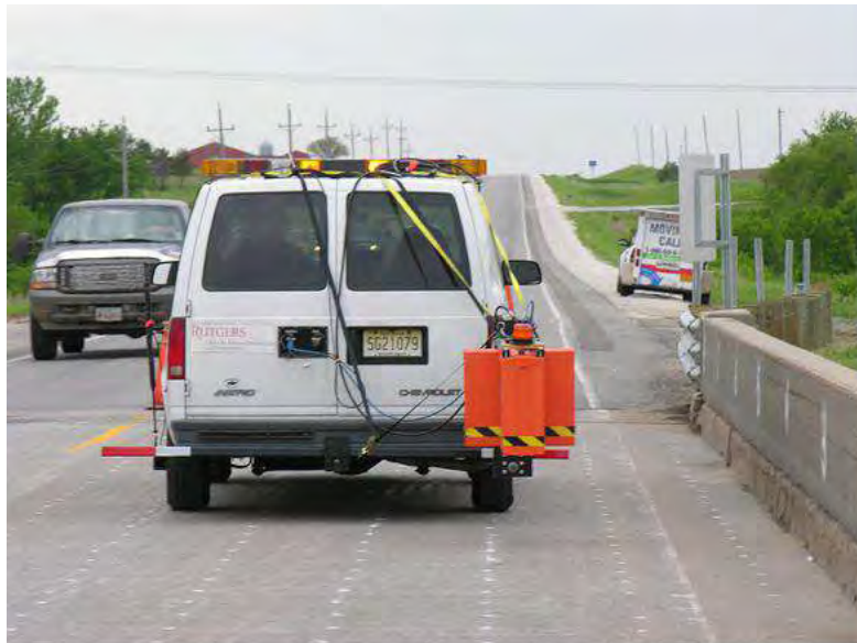
Figure 1.19 - Air coupled vehicle mounted GPR being collected data to examine a bridge deck. https://fhwaapps.fhwa.dot.gov/ndep/DisplayTechnology.aspx?tech_id=9
