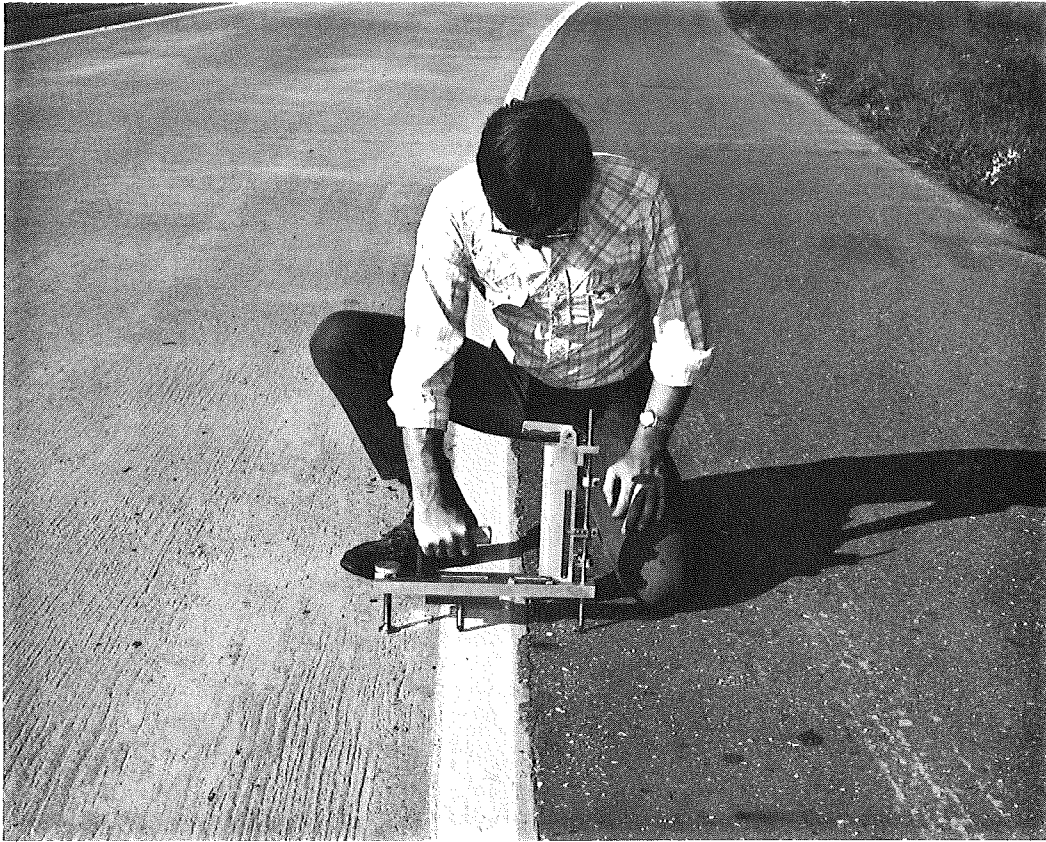
Figure 5. Device used to measure differential shoulder heave.
