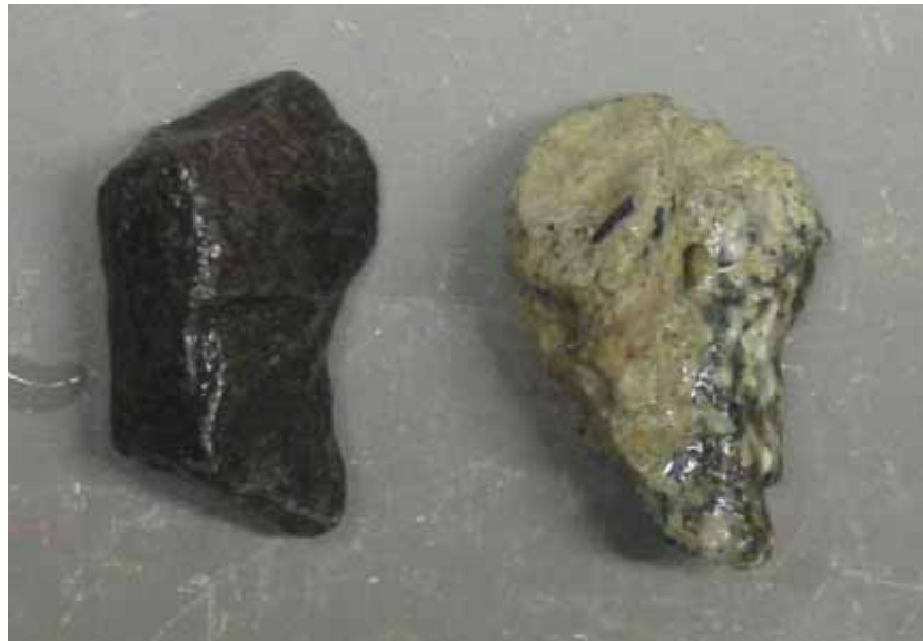
Figure 2-5. Virgin aggregate (left) and recycled concrete aggregate (right) in a moist condition after (Sturtevant 2007).
