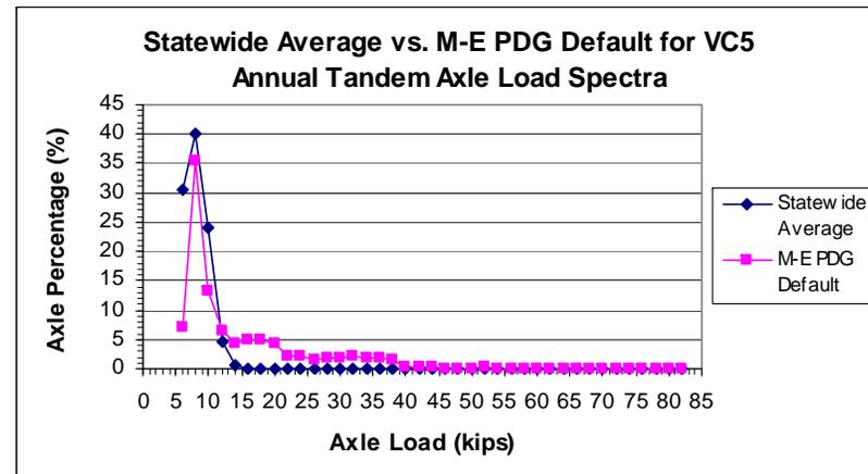
Figure G11.State Avg. vs. M-E PDG Default for Tandem VC4 LS    Figure G12.State Avg. vs. M-E PDG Default for Tandem VC5 LS
