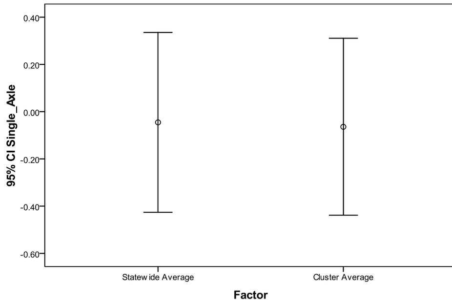
**Figure 4.29 Error Bar Chart for Differences in Flexible Performance Life Based on Fatigue Cracking Due to Single Axle Load Spectra Characterization**
