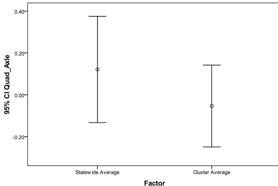
**Figure 4.35 Error Bar Chart for Differences in Flexible Performance Life Based on Fatigue Cracking Due to Quad Axle Load Spectra Characterization**
