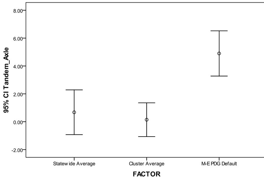
**Figure 4.19 Error Bar Chart for Differences in Rigid Performance Life Based on Tandem Axle Load Traffic Inputs**
