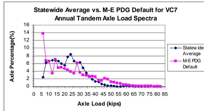
Figure G13.State Avg. vs. M-E PDG Default for Tandem VC6 LS    Figure G14.State Avg. vs. M-E PDG Default for Tandem VC7 LS
