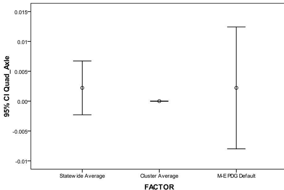
**Figure 4.21 Error Bar Chart for Differences in Rigid Performance Life Based on Quad Axle Load Traffic Inputs**
