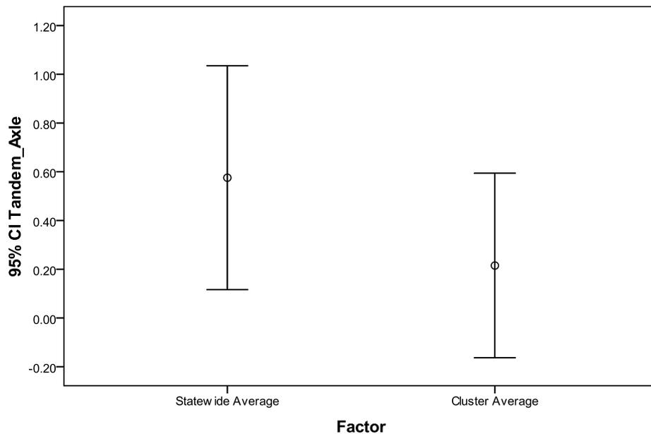
**Figure 4.31 Error Bar Chart for Differences in Flexible Performance Life Based on Fatigue Cracking Due to Tandem Axle Load Spectra Characterization**
