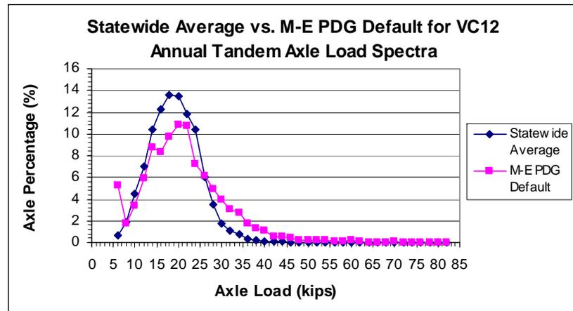
Figure G17.State Avg. vs. M-E PDG Default for TandemVC10 LS Figure G18.State Avg. vs. M-E PDG Default for TandemVC12 LS
