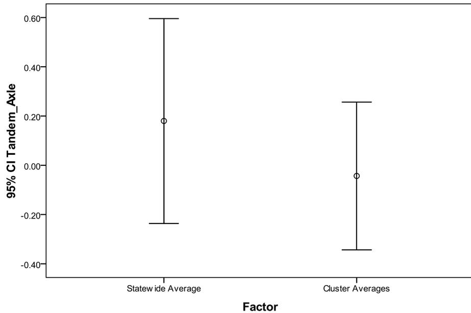
**Figure 4.30 Error Bar Chart for Differences in Flexible Performance Life Based on Rutting Due to Tandem Axle Load Spectra Characterization**
