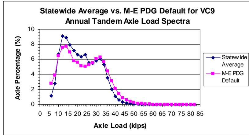
Figure G15.State Avg. vs. M-E PDG Default for Tandem VC8 LS Figure G16.State Avg. vs. M-E PDG Default for TandemVC9 LS
