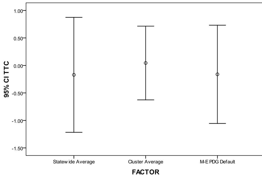
**Figure 4.14 Error Bar Chart for Differences in Rigid Performance Life Based on TTC Traffic Inputs**
