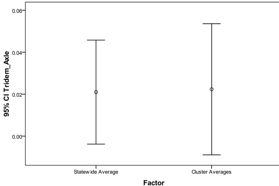
**Figure 4.32 Error Bar Chart for Differences in Flexible Performance Life Based on Rutting Due to Tridem Axle Load Spectra Characterization**
