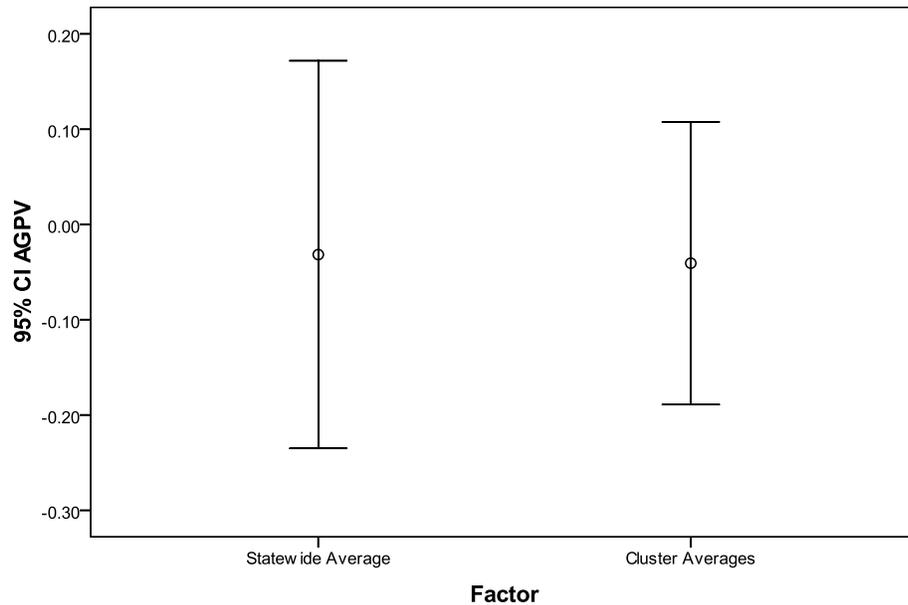
**Figure 4.26 Error Bar Chart for Differences in Flexible Performance Life Based on Rutting Due to AGPV Characterization**
