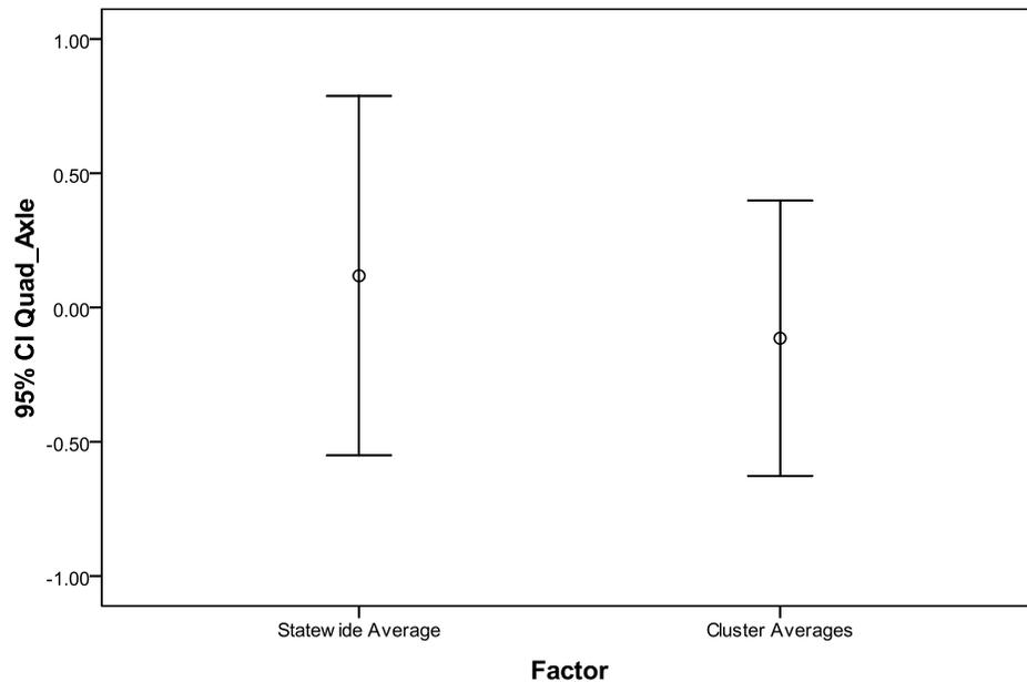
**Figure 4.34 Error Bar Chart for Differences in Flexible Performance Life Based on Rutting Due to Quad Axle Load Spectra Characterization**
