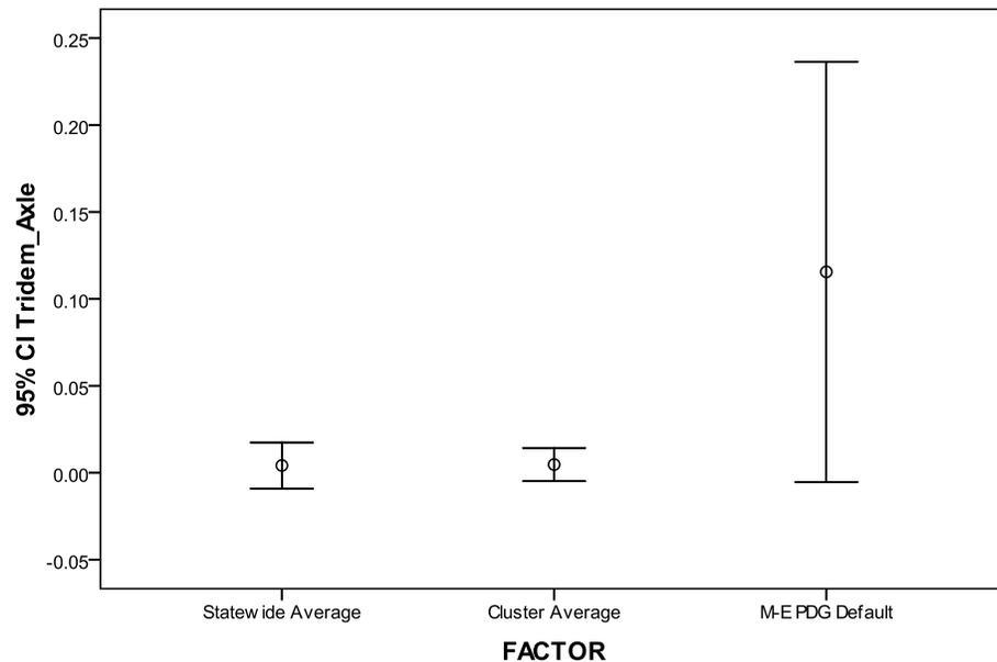
**Figure 4.20 Error Bar Chart For Differences in Rigid Performance Life Based on Tridem Axle Load Traffic Inputs**
