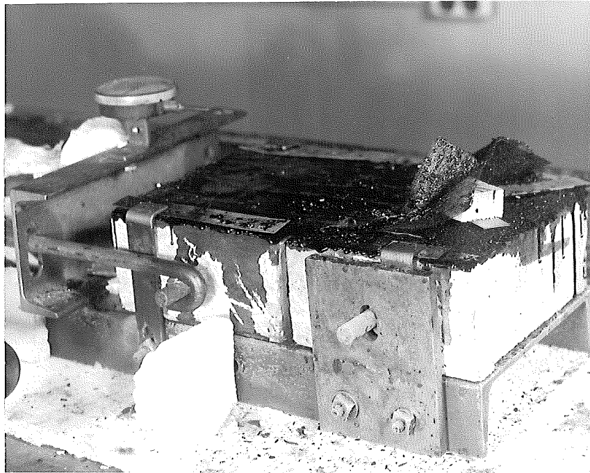
Figure 4. Note how fabric layers have separated.
