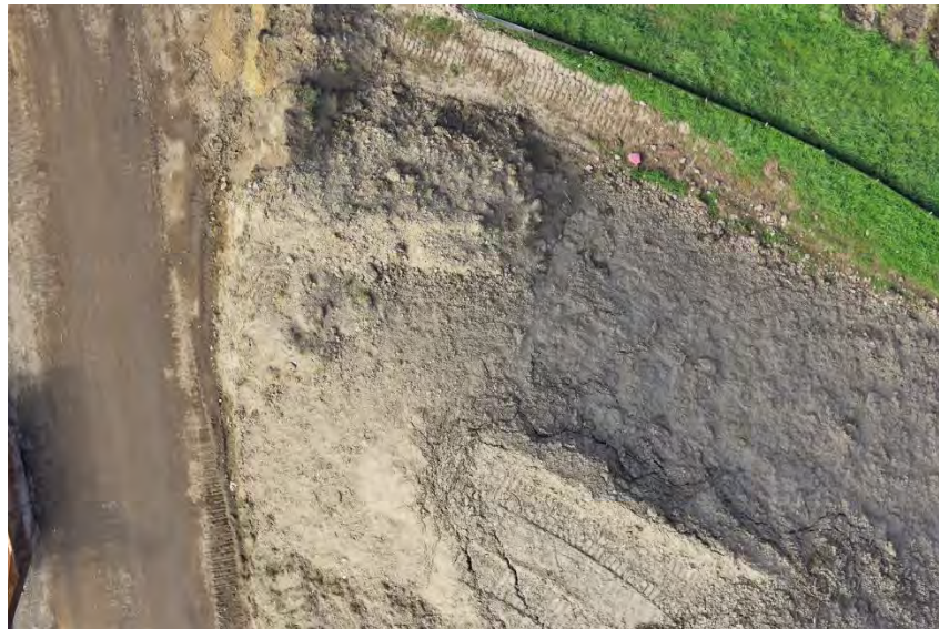
Figure 7: Nikon D810 36 MP image of one of the construction aggregate mounds as collected with the Bergen Hexacopter; it was used to create an orthophoto and DEM of the construction site area.
