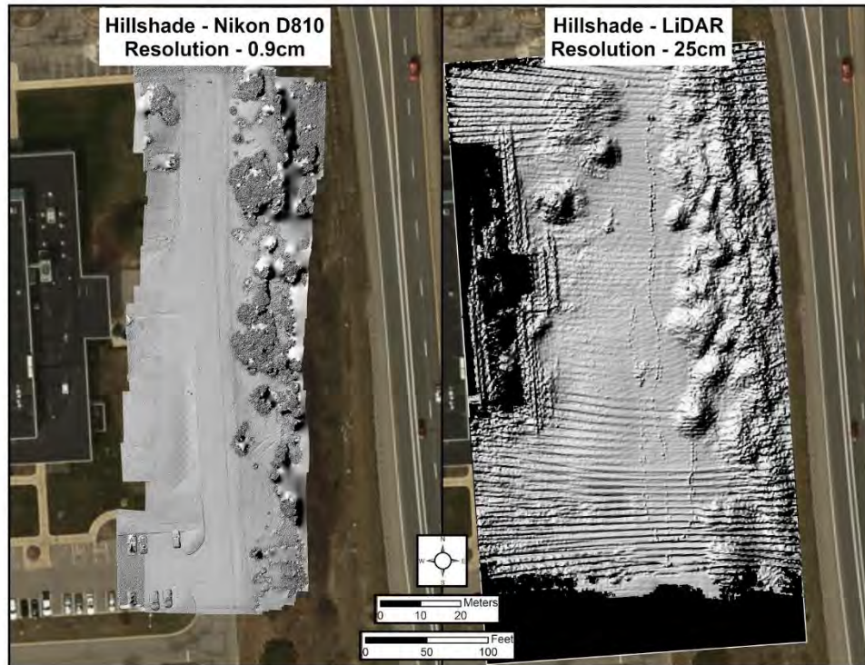
Figure 34: Comparison of a hillshade product for the same area using photogrammetric data collected using a Nikon D810 camera vs. the November, 2017 version of the lidar setup flown aboard the same Bergen Quad-8 UAV.
