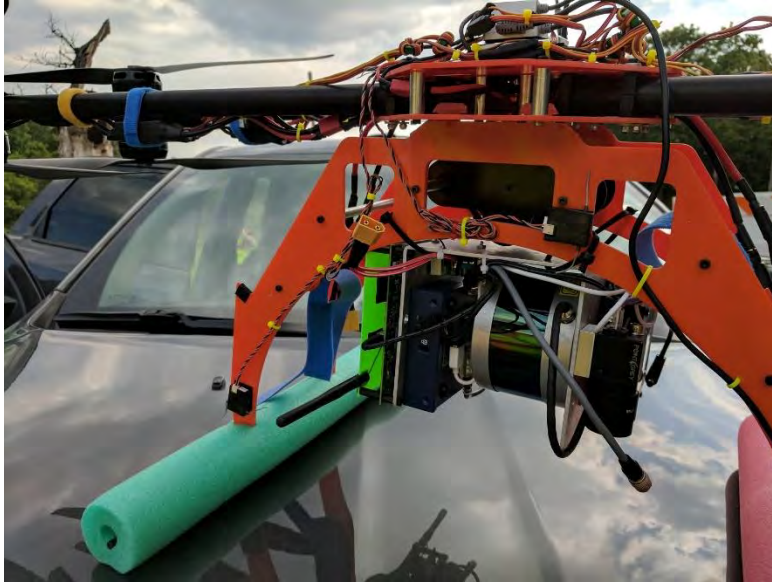
Figure 55: The Velodyne lidar puck on the Bergen Quad-8 with the original June, 2017 setup.
