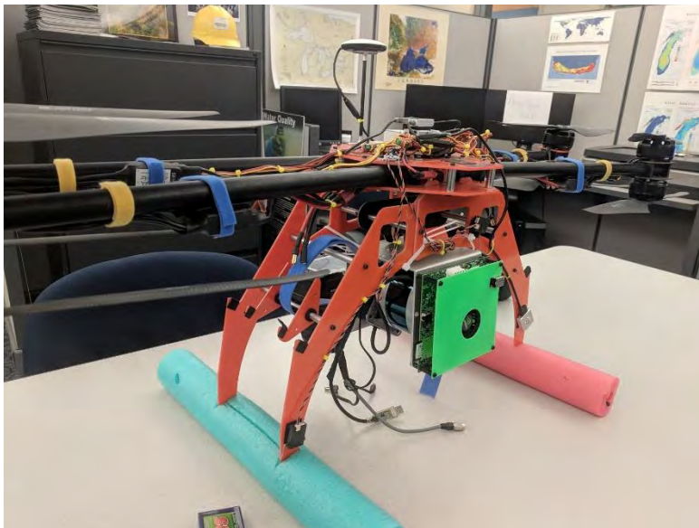
Figure 56: The Velodyne lidar puck on the Bergen Quad-8 in the revised November, 2017 setup. The Jetson TK1 control board is underneath the green protective panel.
