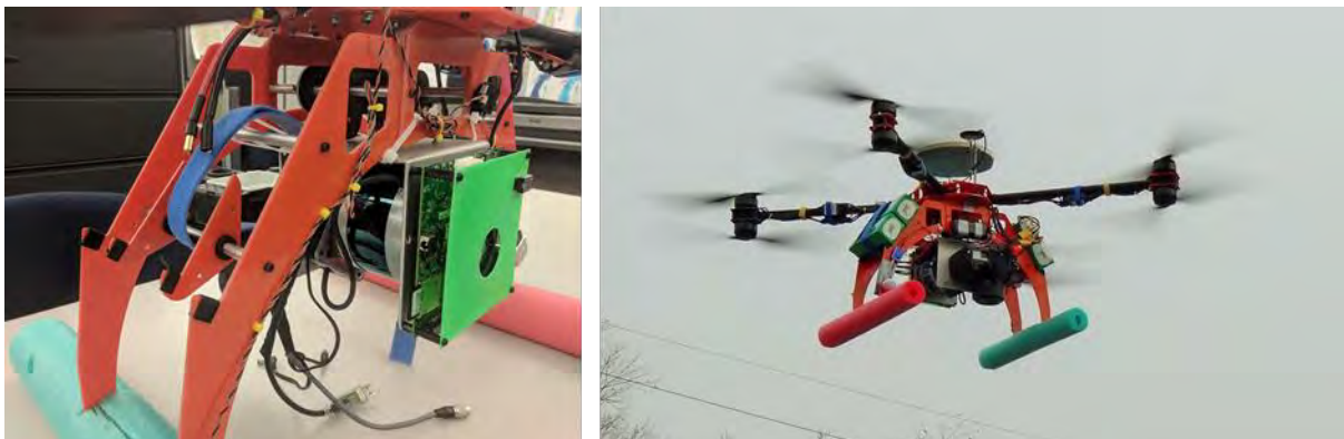
Figure 36: Quad-8 UAV with mounted lidar system (left) and deployed over the MTRI roadway site, collecting lidar data (right).
