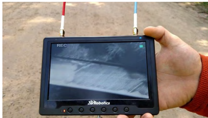
Figure 46: Thermal imagery of a bridge deck being shown live via FPV to the operator and nearby project staff.
