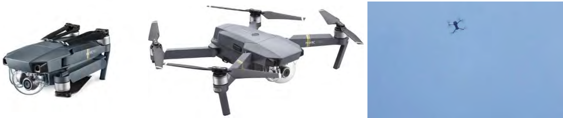
Figure 38: The DJI Mavic Pro, in folded mode for easy transport (left), in ready-to-fly mode (center), and flying over the US-31 corridor site (right).
