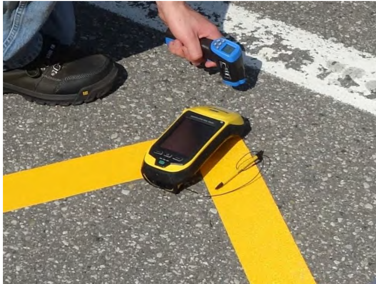
Figure 57: The Trimble GeoExplorer GPS unit being used to collect the location of a ground control point. In the background, a hand-held digital thermometer is being used to collect ground-reference data to compare to thermal imaging results.
