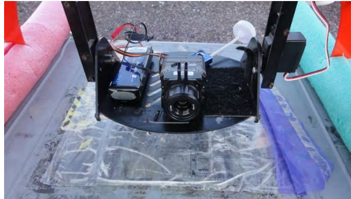
Figure 45: The FLIR Vue Pro onboard of the Bergen Hexacopter.
