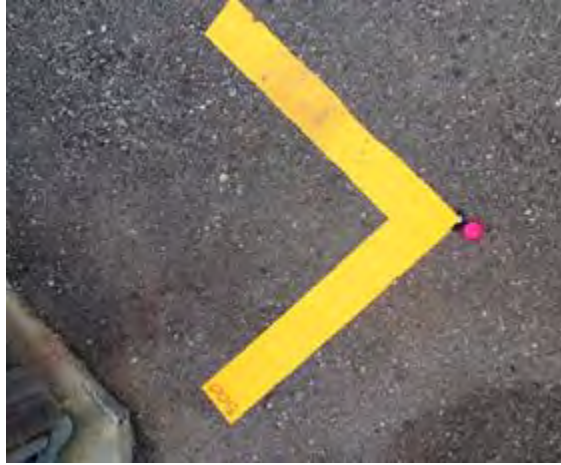
Figure 59: A chevron used to mark where GPS measurements were collected.
