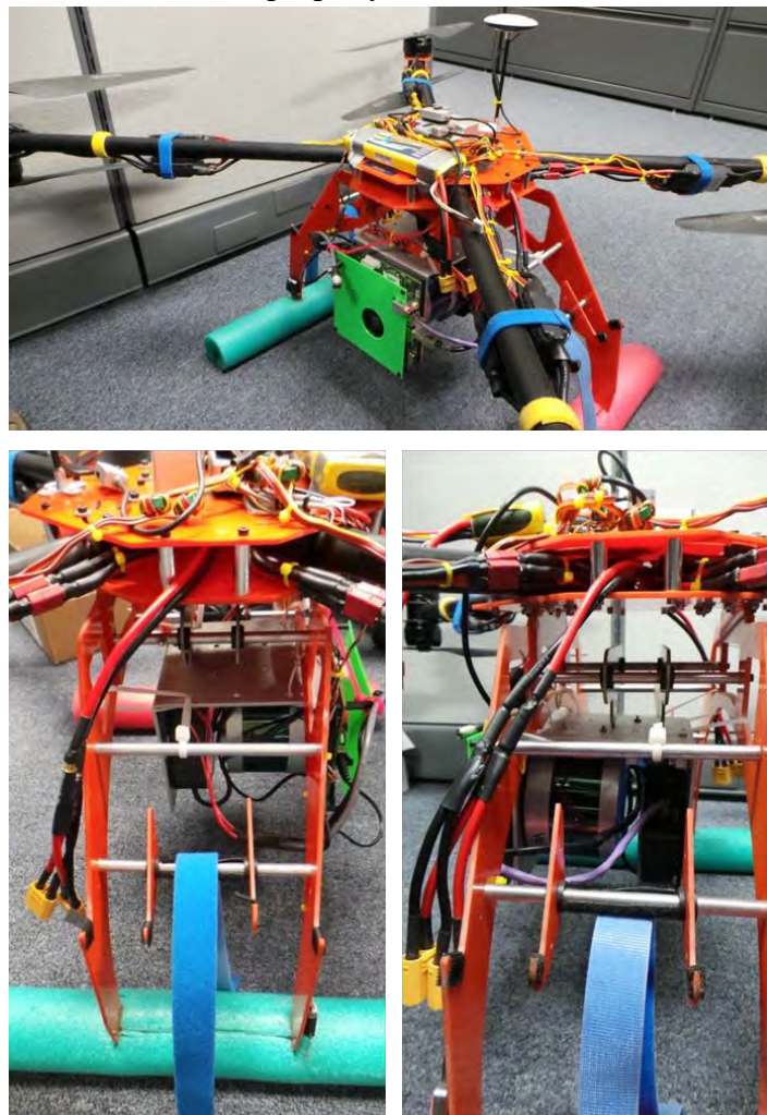
Figure A14: Bergen Q-8 with lidar attachment.
