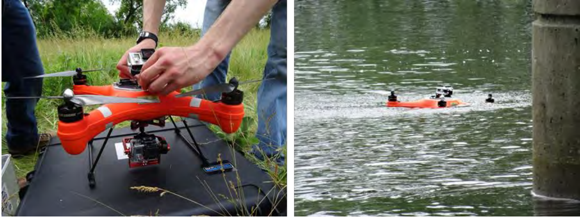
Figure 39: Waterproof Mariner 2 Splash being prepared for flight (left) and while collecting data after having landed on the water to image the underneath of the US-31 / White River bridge using GoPro cameras (right).
