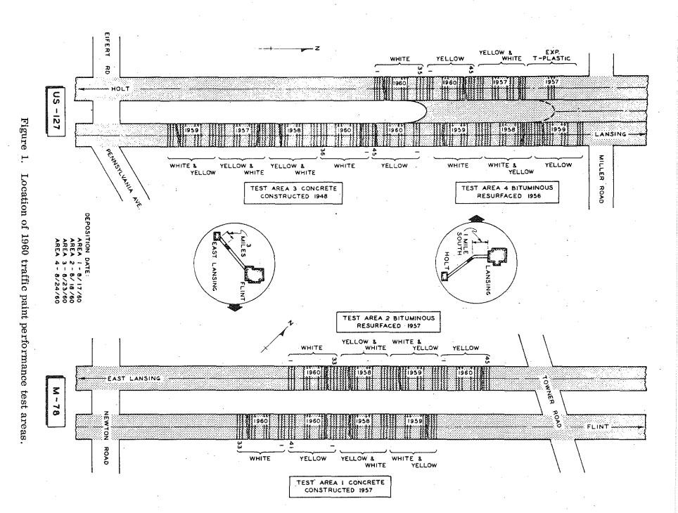
Each test paint was deposited as a series of three transverse stripes; the standard paints in all four areas, the experimental paints usually in fewer areas.
