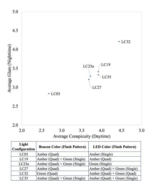
Figure 5-17 Dynamic experiment under clear weather conditions – comparing average conspicuity (daytime) and average glare (nighttime) for six light configurations
