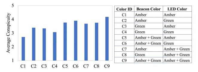
Figure 5-19 Static experiment under snowy conditions: Conspicuity test results for nine color groups in the daytime contrast
