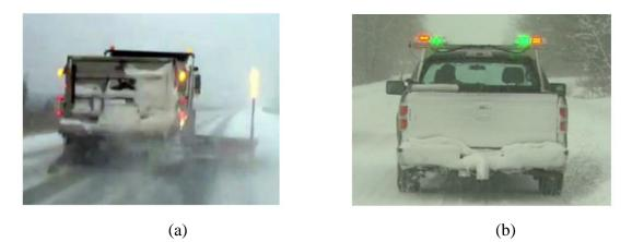
Figure 2-3 Winter maintenance vehicle warning lights: (a) MDOT vehicle warning lights (Source: Weingarten, 2016) and (b) new proposed green warning lights (Source: Walker, 2014)
