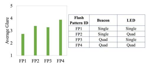
Figure 5-23 Static experiment under snowy conditions: Glare rating test results for four flash pattern groups in the nighttime contrast
