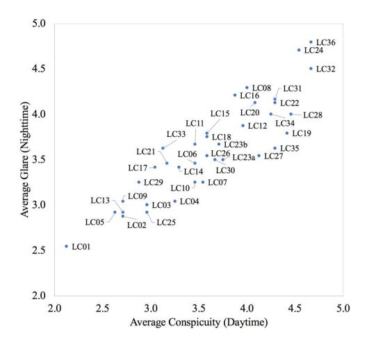
Figure 5-8 Static experiment under clear weather conditions: Relationship between conspicuity (daytime) and glare (nighttime)
