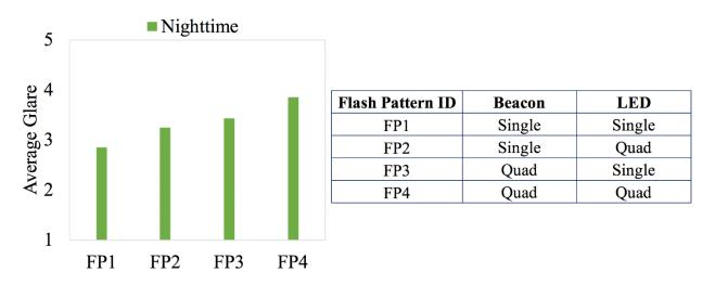
Figure 5-7 Static experiment under clear weather conditions: Glare rating test results for four flash pattern groups in nighttime contrast
