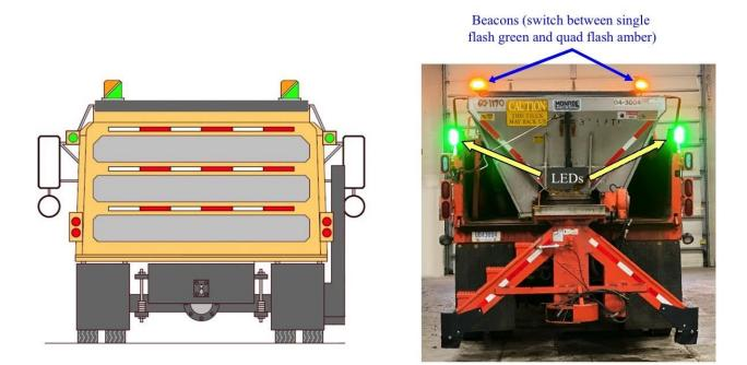
Figure 4-11 MDOT current configuration for warning lights
