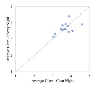
Figure 5-24 Static experiment under snowy conditions: Comparison of glare average values over various warning light configurations for each participant in clear and snowy weather conditions
