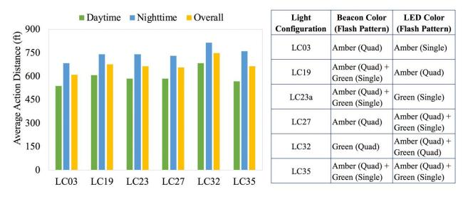
Figure 5-11 Dynamic experiment under clear weather conditions: Action-taking distance test results for six light configurations in daytime and nighttime contrasts
