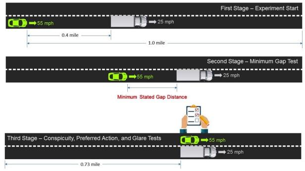
Figure 4-7 Different stages of the dynamic experiment
