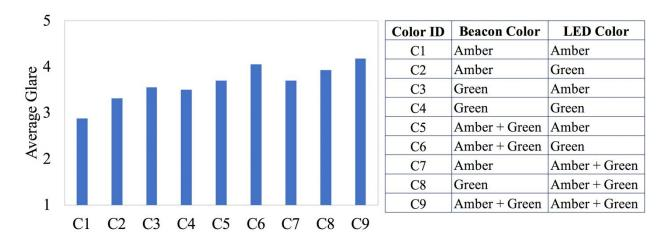
Figure 5-22 Static experiment under snowy conditions: Conspicuity test results for nine color groups in the nighttime contrast
