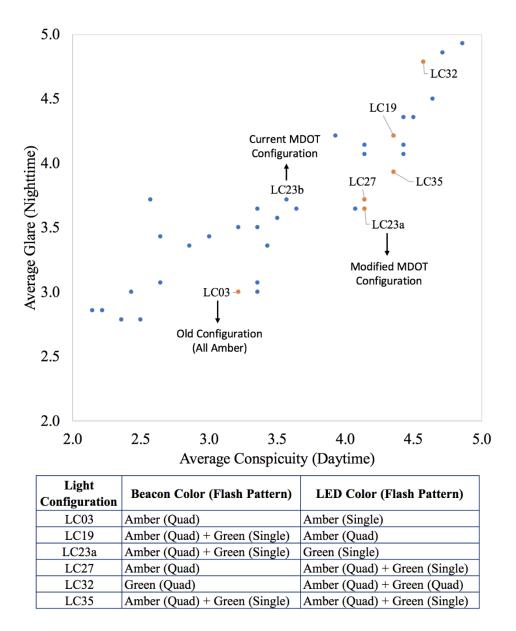
Figure 5-26 Static experiment under snowy conditions: Relationship between conspicuity (daytime) and glare (nighttime) averaged over all participants for six highlighted warning light configurations (used in the dynamic experiment)
