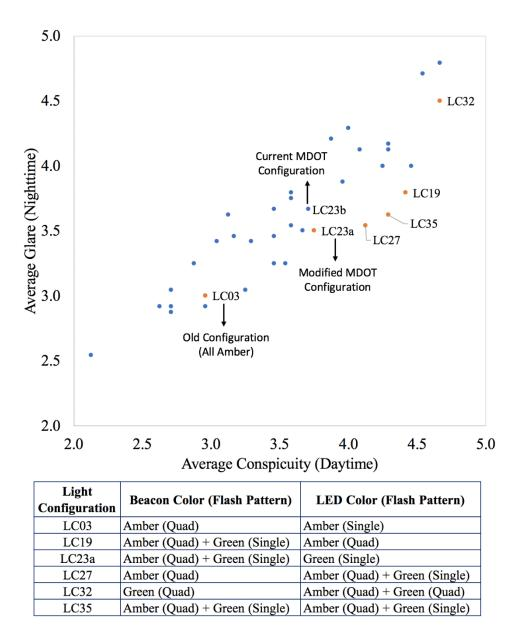
Figure 5-9 Candidate light configurations for further assessments in the dynamic experiment (orange dots are selected configurations for the dynamic experiment and the blue dots are configurations used only in the static experiment)
