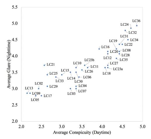
Figure 5-25 Static experiment under snowy conditions: Relationship between conspicuity (daytime) and glare (nighttime) averaged over all participants for each warning light configuration
