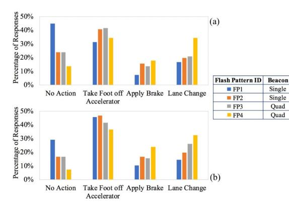
Figure 5-4 Static experiment under clear weather conditions: Appropriate driving action test results for four flash pattern groups: (a) daytime and (b) nighttime
