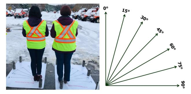
Figure 4-3 Maximum peripheral detection angle test configuration
