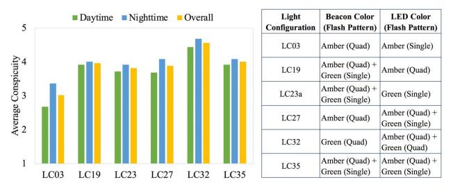
Figure 5-13 Dynamic experiment under clear weather conditions: Conspicuity test results for six light configurations in daytime and nighttime contrasts
