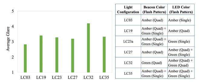
Figure 5-16 Dynamic experiment under clear weather conditions: Glare test results for six light configurations in nighttime contrast
