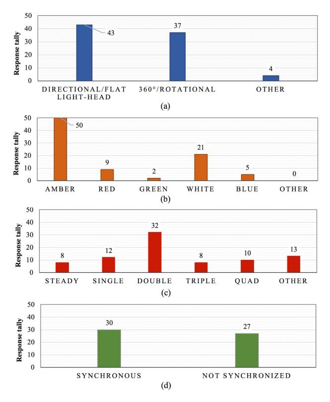
Figure 3-2 Types, colors and flash patterns of auxiliary warning lights on general maintenance trucks: (a) types of auxiliary warning lights, (b) colors of auxiliary warning lights, (c) flash patterns and (d) synchronization types
