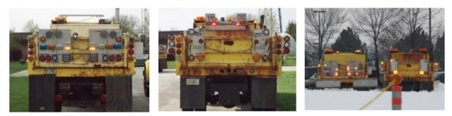
Figure 2-1 Examples of warning lights layout (Source: McCullouch and Stevens, 2008)
