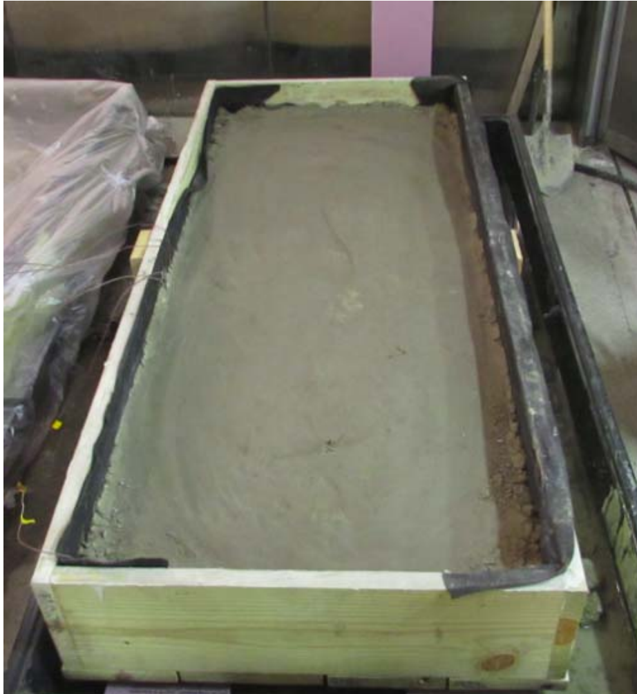
Figure 3.54: Full Scale Freeze/Thaw Test Sample
