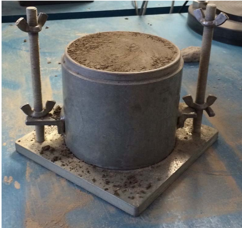
Figure 3.6: Sample Prepared for Standard Proctor Test
