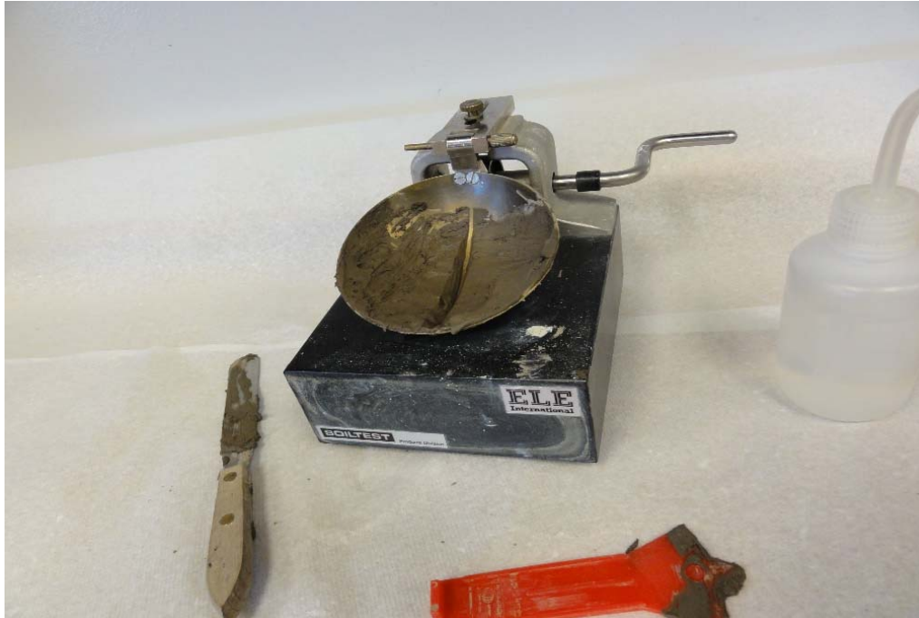
Figure 3.3: Cassagrande Apparatus for Liquid Limit Testing
