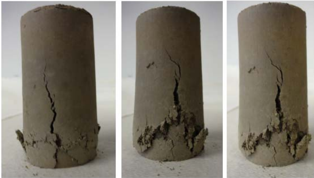
Figure 3.12: Soil Specimen after Failure
