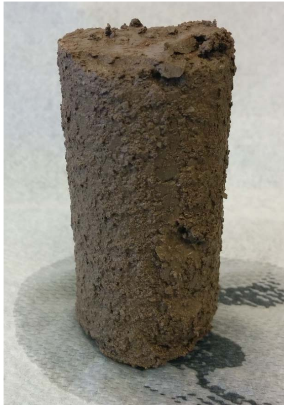
Figure 3.51: Condition of Specimen after Seven Freeze/Thaw Cycles and 24 Hours of Capillary Soaking (Soil-1 stabilized with 8% CKD)
