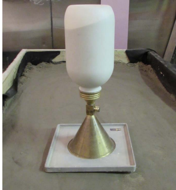
Figure 3.56: In situ Density Test Using Sand Cone Method
