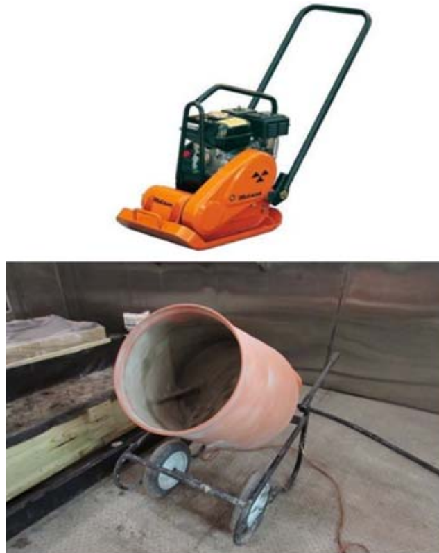
Figure 3.55: Mixing Soil-Recycled Materials (Down) and Compactor (Up)
