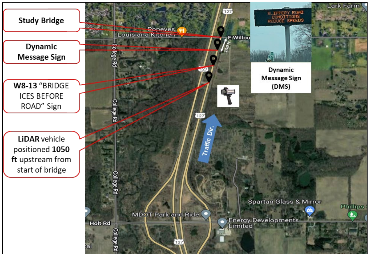
Figure 18. Field Evaluation Layout and for DMS Evaluation at NB US-127 Lansing Site
