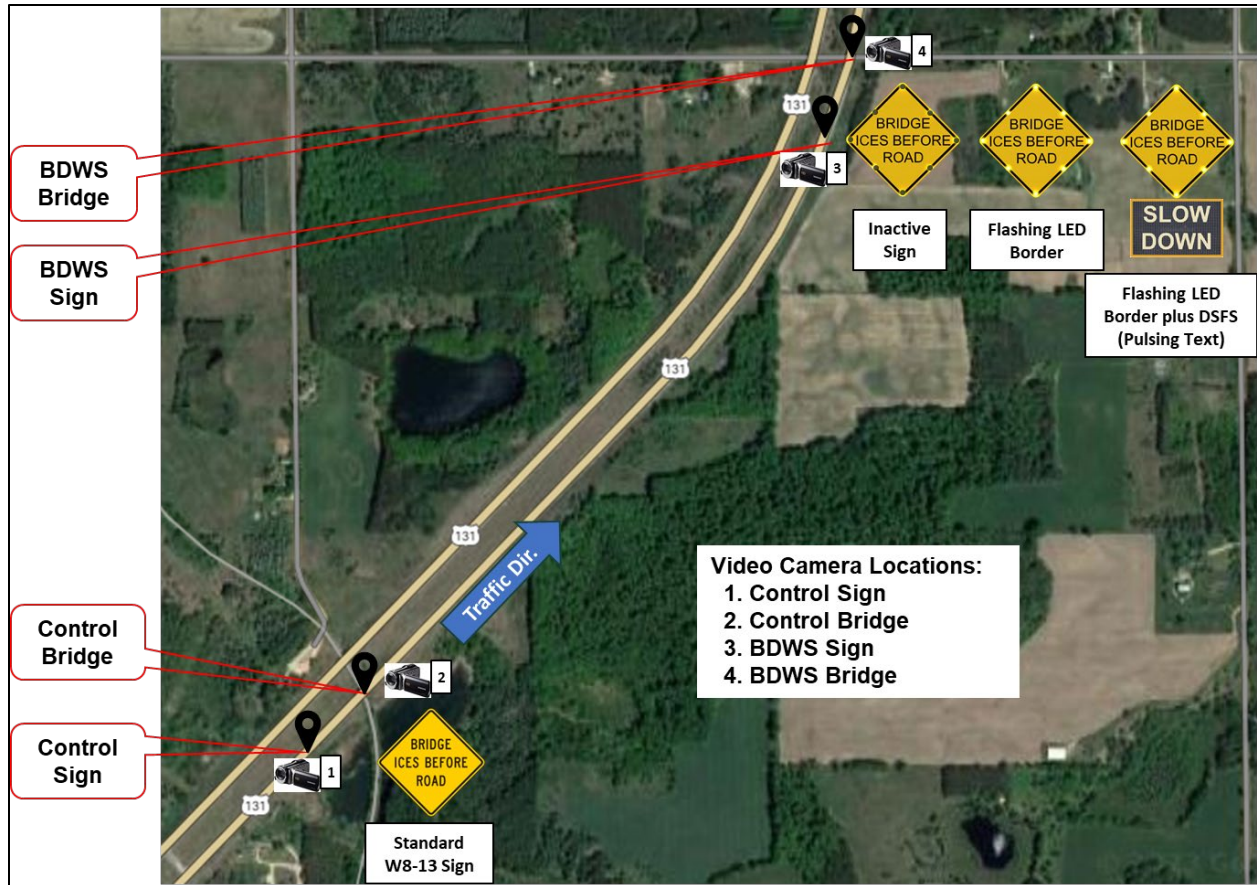
Figure 12. Field Evaluation Layout and Sign Test Conditions at NB US-131 Cadillac Site
