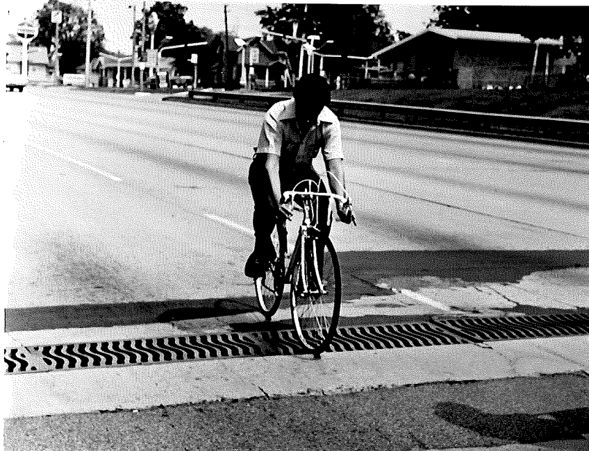
Figure 4. Bicycle test runs at various speeds and angles over sinusoidal grating.
