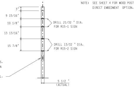
4" X 9" NATIONAL INVENTORY NUMBER TAG (SALVAGED OR FURNISHED BY THE RAILROAD) SHALL BE INSTALLED USING EITHER NAILS OR LONG STAPLES. THE INSTALLATION SHALL BE ON SIDE OF POST FACING THE ROADWAY JUST ABOVE EYE LEVEL.
