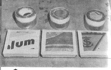
Figure 6. Containers of calcium chloride covered with flat bag sections, prepared for exposure tests.
