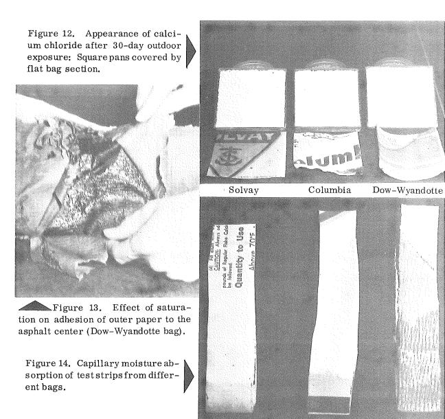
strips, but the Dow-Wyandotte bag shows a considerable rise. The high rate of absorption by the Dow-Wyandotte bag might be due to the treatment used to blot the excess asphalt. It is a serious defect and one that accentuates the damage caused by any contact of the bag with moisture.
