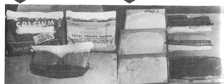
Figure 6 shows other forms of samples used. Each circular can was partially filled with calcium chloride and the top covered with a flat bag section containing no joints, bent sections, or seams. The sample was so prepared that any moisture increase to the calcium chloride would have to come through the bag section. The calcium chloride was not in contact with the bag section during this test. These samples were placed in the 100 percent relative humidity room.
