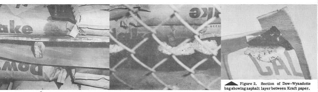
Figure 1. Typical deterioration of calcium chloride bags during storage.
