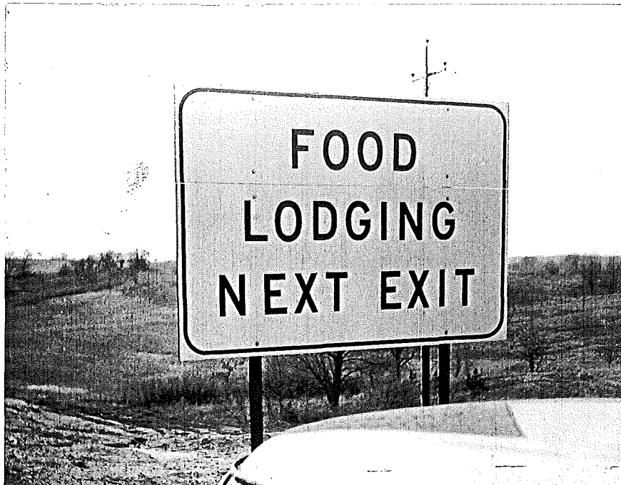
Figure 2. Non-reflectorized green tape and white reflectorized background on plywood.
