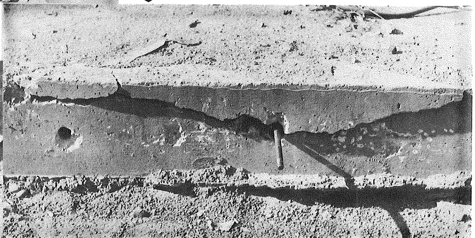
Figure 11. Typical condition of concrete slab after failure using 5/8-in. diameter or 3/4-in. diameter Bethlehem steel expansion sleeve devices.
