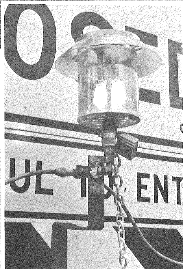
▲ Figure 2. Propane light (center mounted) showing attachment bracket and security lock.
