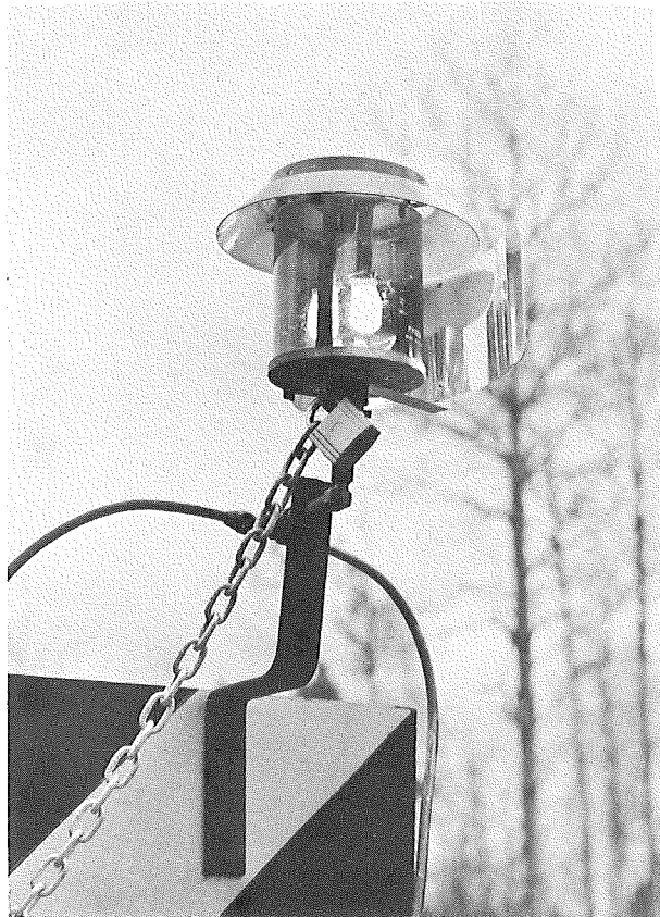
▲ Figure 2. Propane light (center mounted) showing attachment bracket and security lock.
