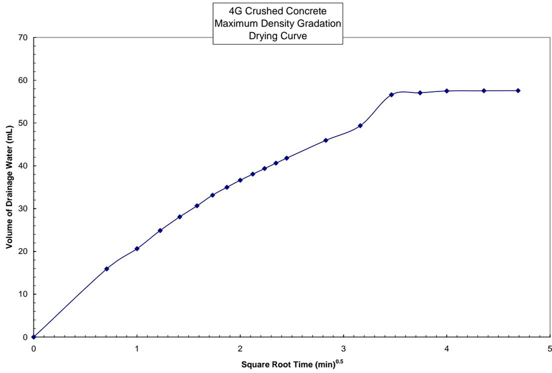
Figure 3.1-13 Drying Curve, Maximum Density Gradation, Crushed Concrete
