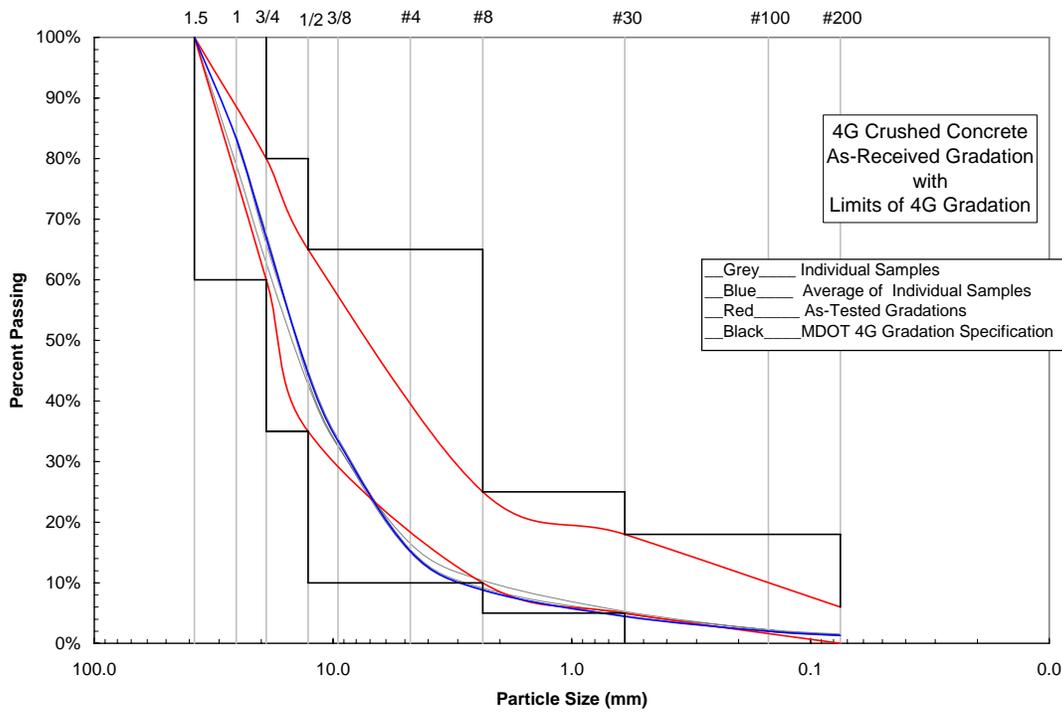
Figure 2.2-4 As-Received and As-Tested Gradations; 4G Crushed Concrete
