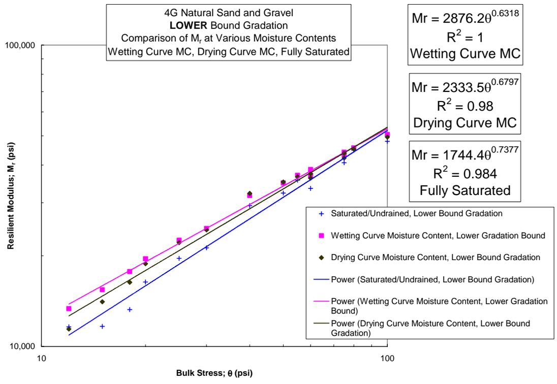
Figure 3.3-4 Natural Gravel, Lower Bound Gradations, Wetting and Drying Curve MC, Fully Saturated MC
