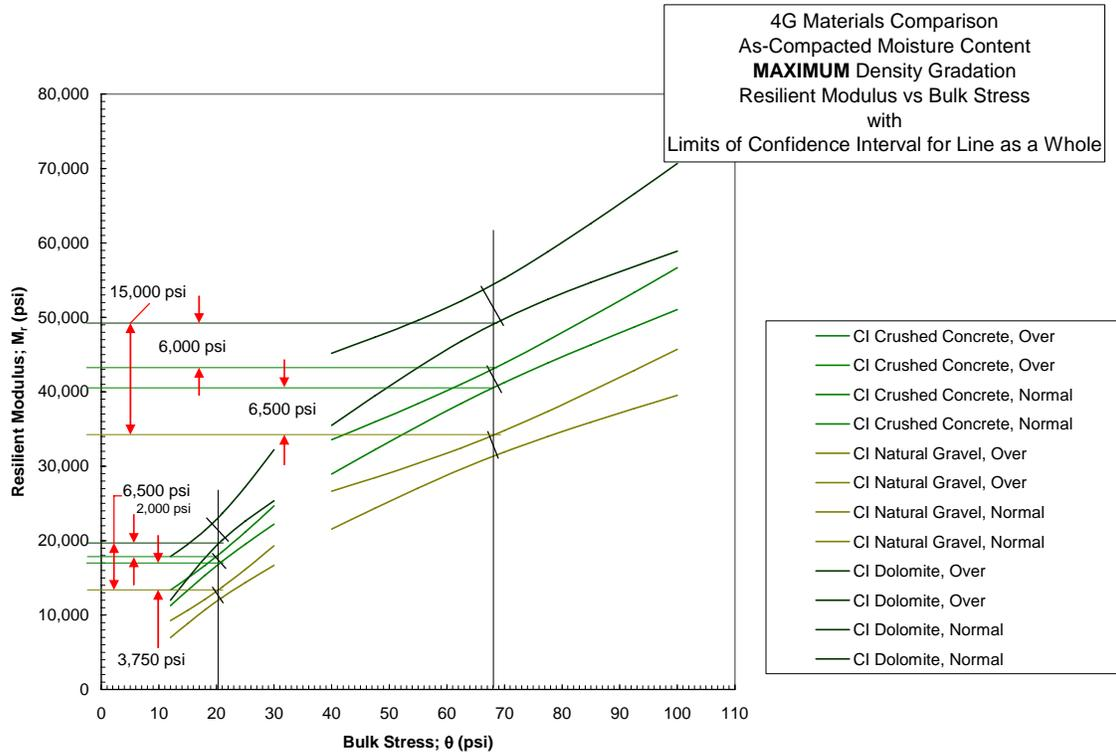
Figure 4.3-5 Maximum Density Gradation Comparing Dolomite, Crushed Concrete, and Natural Gravel
