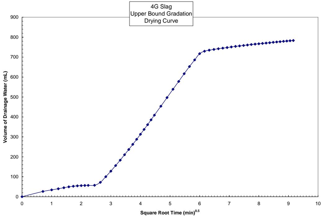
Figure 3.1-9 Drying Curve, Upper Bound Gradation, Slag
