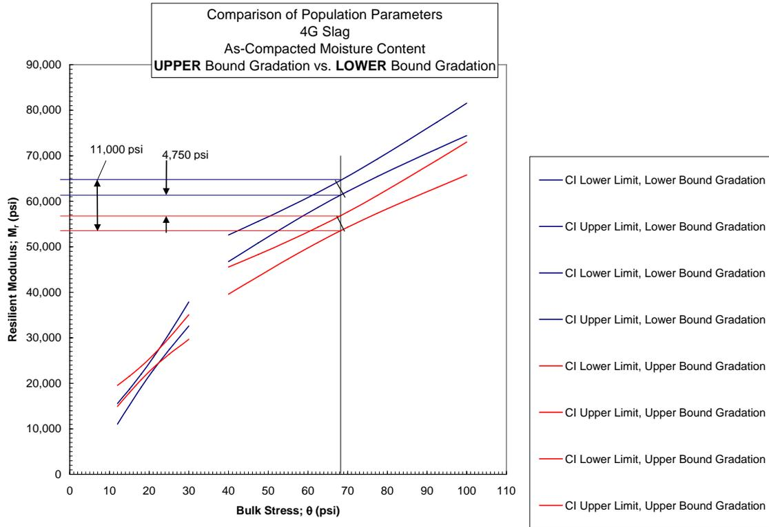
Figure 4.1-20 Stiffness Difference between Upper and Lower Bound Gradations; Slag
