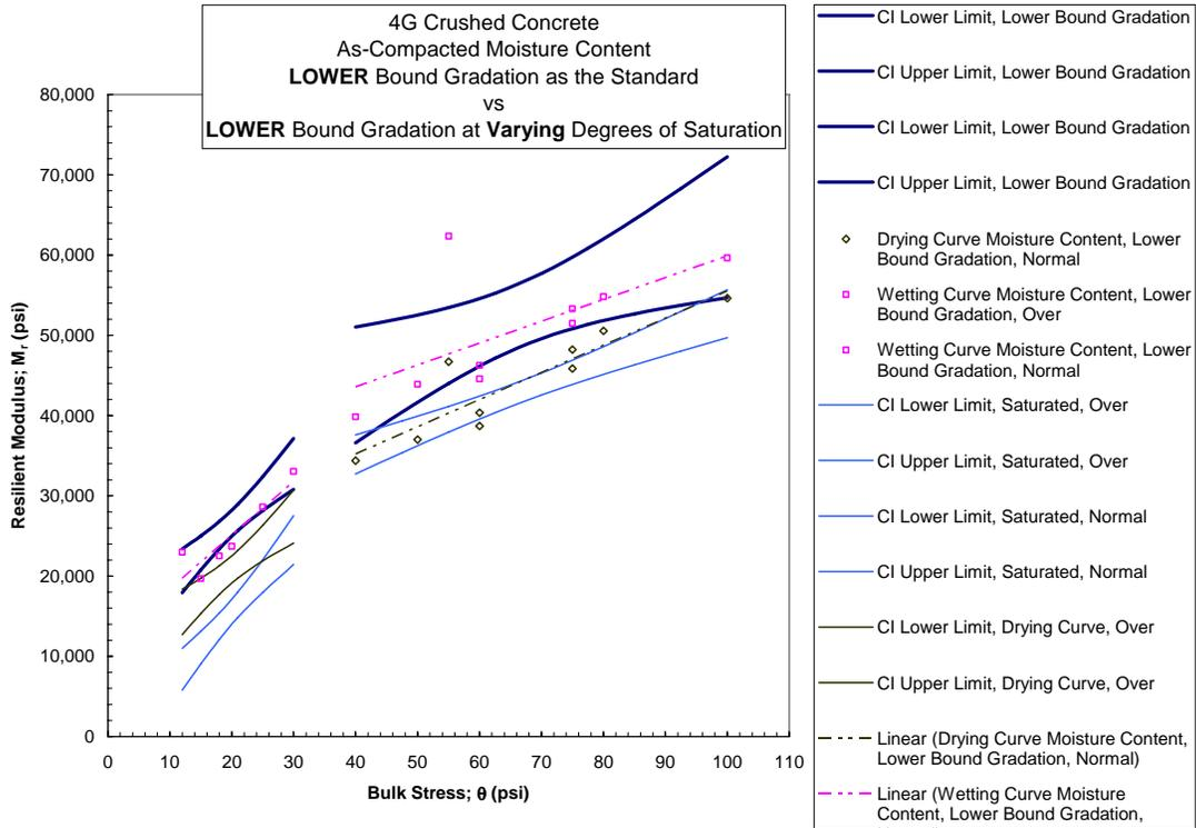
Figure 4.2-23 Crushed Concrete Lower Bound Gradation Comparing Effect of MC with Drying Curve MC and Fully Saturated Curve MC CI Bands
