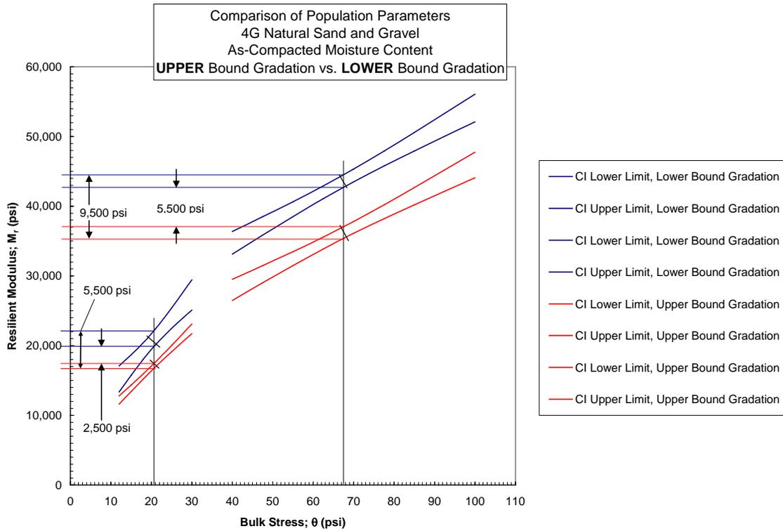
Figure 4.1-14 Stiffness Difference between Upper and Lower Bound Gradations; Natural Gravel
