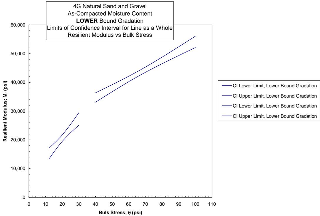
Figure 4.2-2 95% CI Band sans measured data - Natural Gravel Lower Bound Gradation as-compacted MC; Linear-Linear Space
