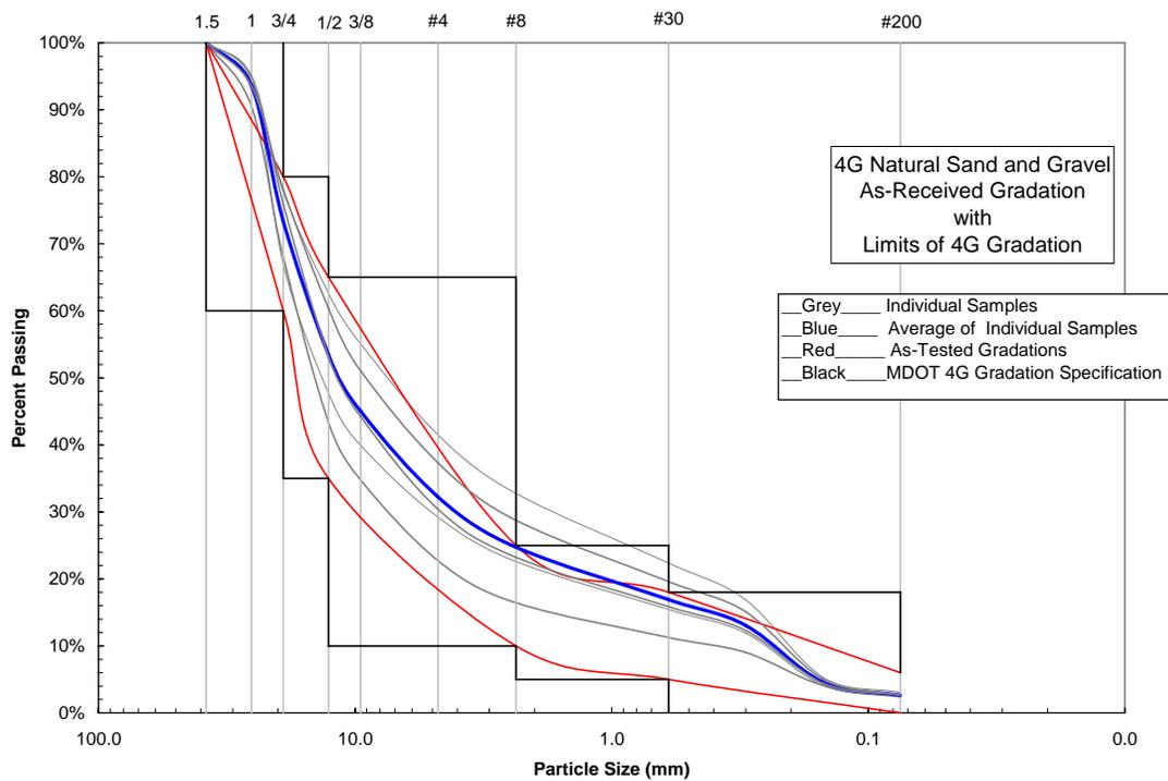
Figure 2.2-1 As-Received and As-Tested Gradations; 4G Natural Gravel
