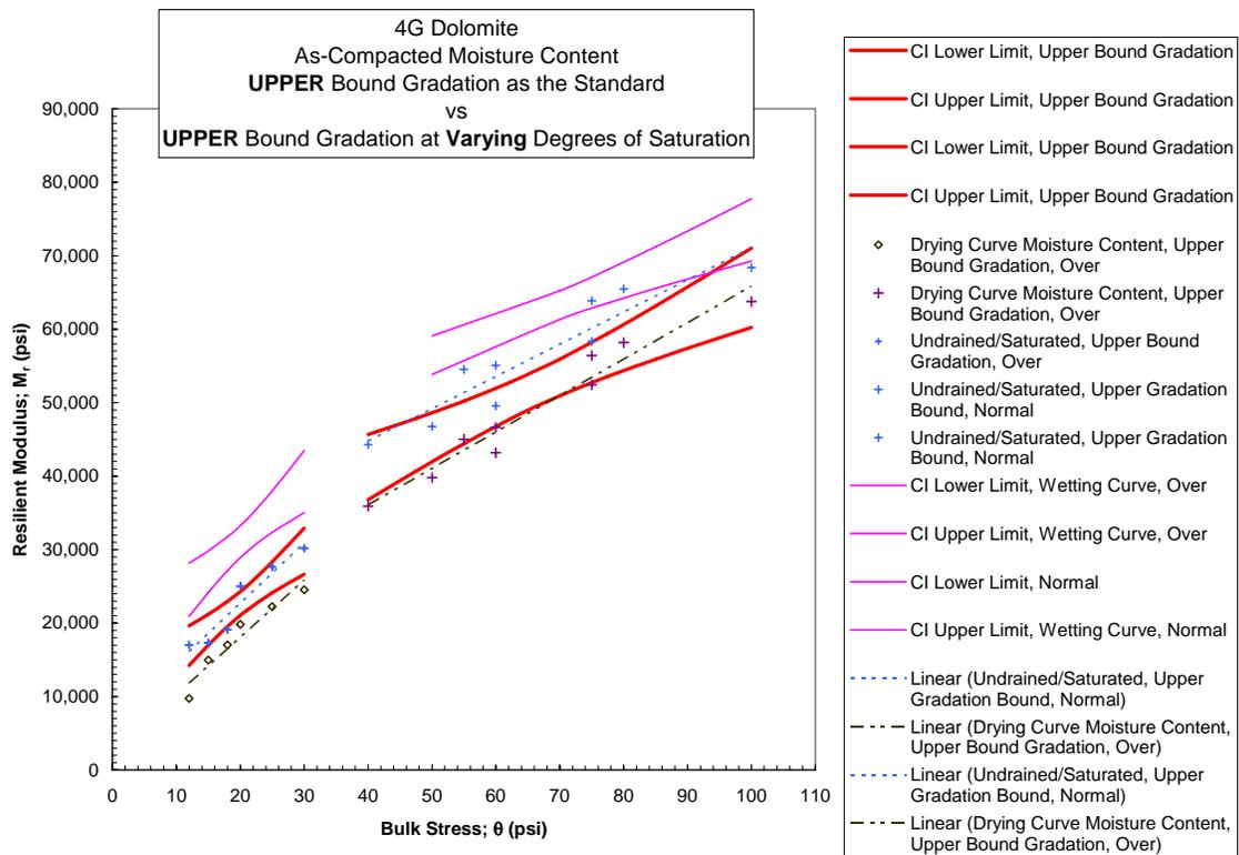
Figure 4.2-13 Dolomite Upper Bound Gradation Comparing Effect of MC with Wetting Curve MC CI Band
