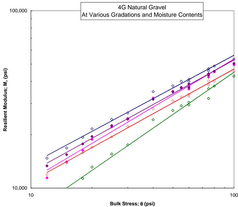
Figure 4.1-3 Resilient Modulus vs Bulk Stress for Natural Gravel at Various Gradations and Moisture Contents
