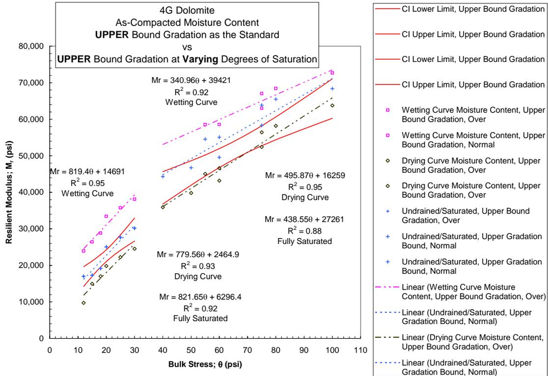
Figure 4.2-12 Dolomite Upper Bound Gradation Comparing Effect of MC
