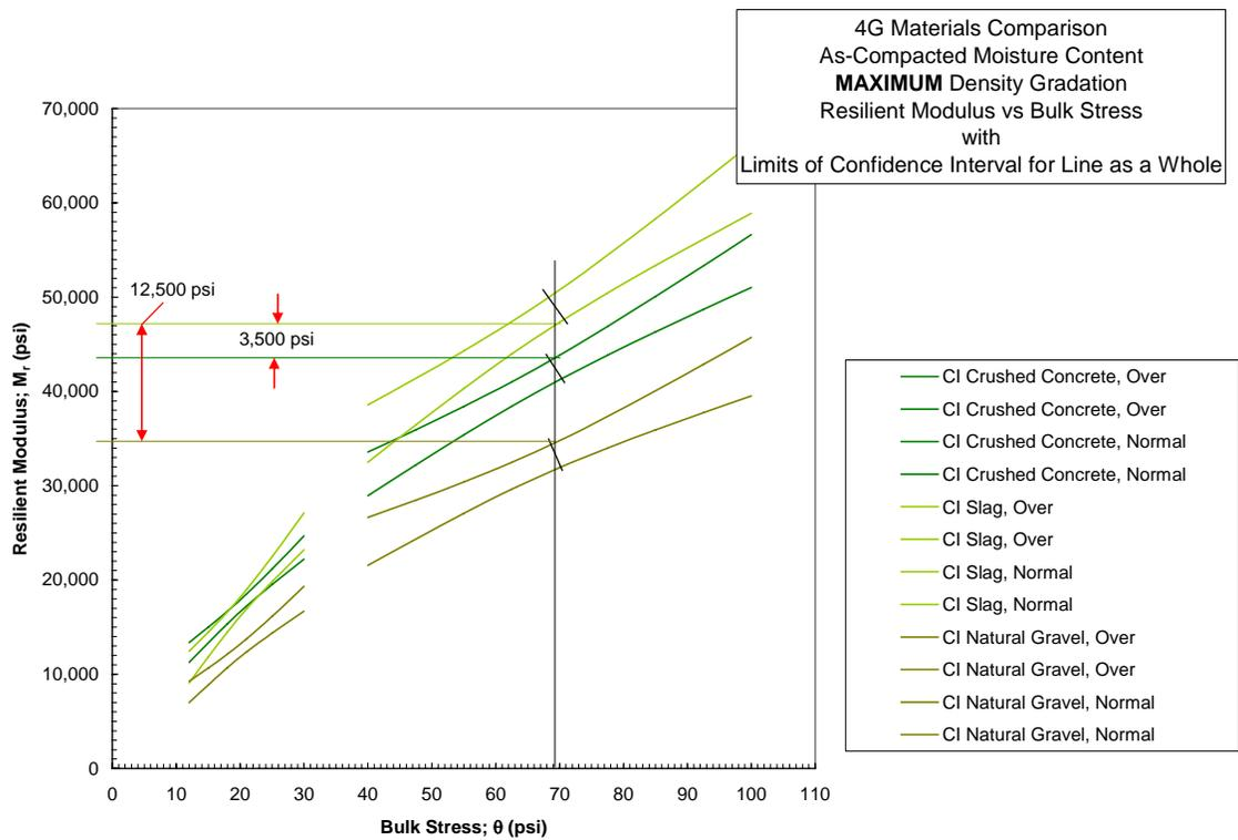
Figure 4.3-6 Maximum Density Gradation Comparing Slag, Crushed Concrete, and Natural Gravel
