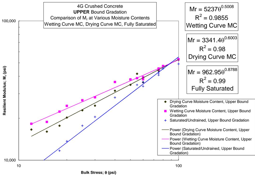
Figure 3.3-23 Crushed Concrete, Upper Bound Gradations, Wetting and Drying Curve MC, Fully Saturated MC
