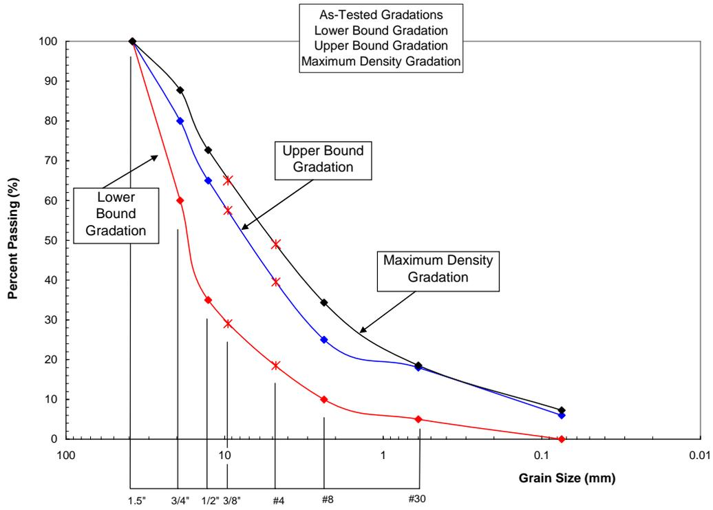
Figure 2.2-5 *As-Tested Gradations; Lower Bound Gradation, Upper Bound Gradation, Maximum Density Gradation*
