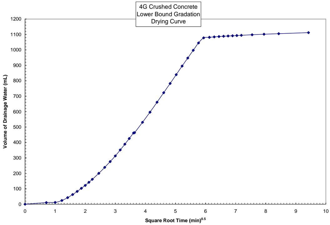
Figure 3.1-11 Drying Curve, Lower Bound Gradation, Crushed Concrete
