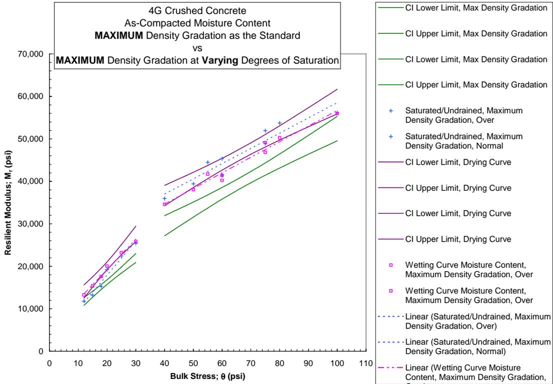
Figure 4.2-26 Crushed Concrete Maximum Density Gradation Comparing Effect of MC
