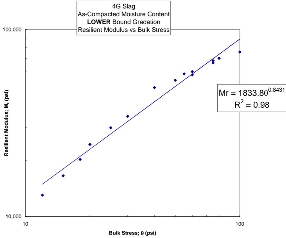
Figure 3.3-13 Slag, Lower Bound Gradation
