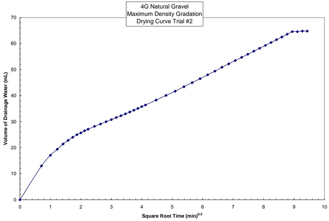
Figure 3.1-4 Drying Curve, Maximum Density Gradation, Natural Gravel Trial no. 2
