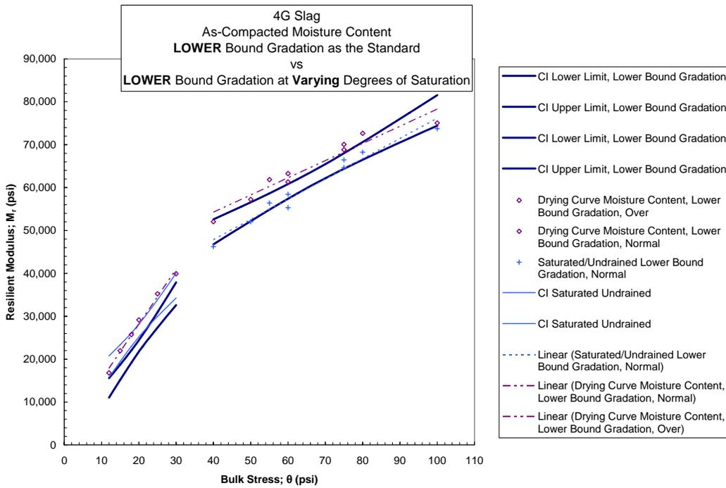
Figure 4.2-16 Slag Lower Bound Gradation Comparing Effect of MC with Saturated MC CI Band
