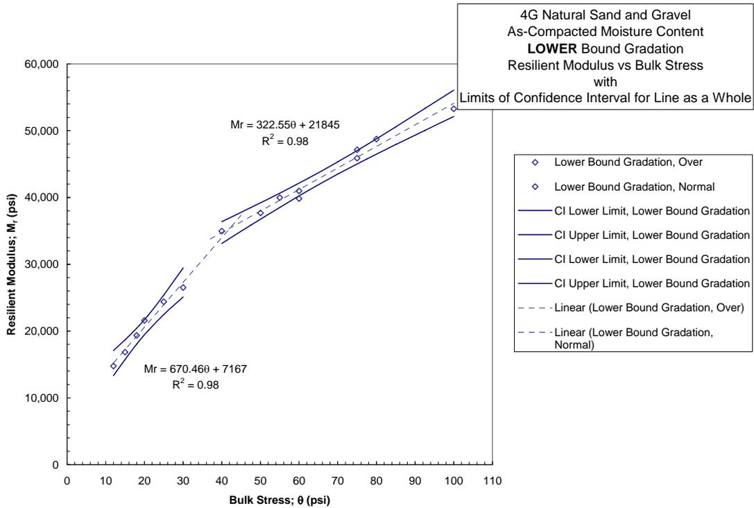
Figure 4.1-11 Resilient Modulus vs Bulk Stress with Limits of 95% Confidence Interval; Linear-Linear Space
