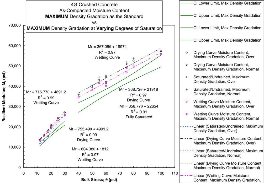
Figure 4.2-25 Crushed Concrete Maximum Density Gradation Comparing Effect of MC
