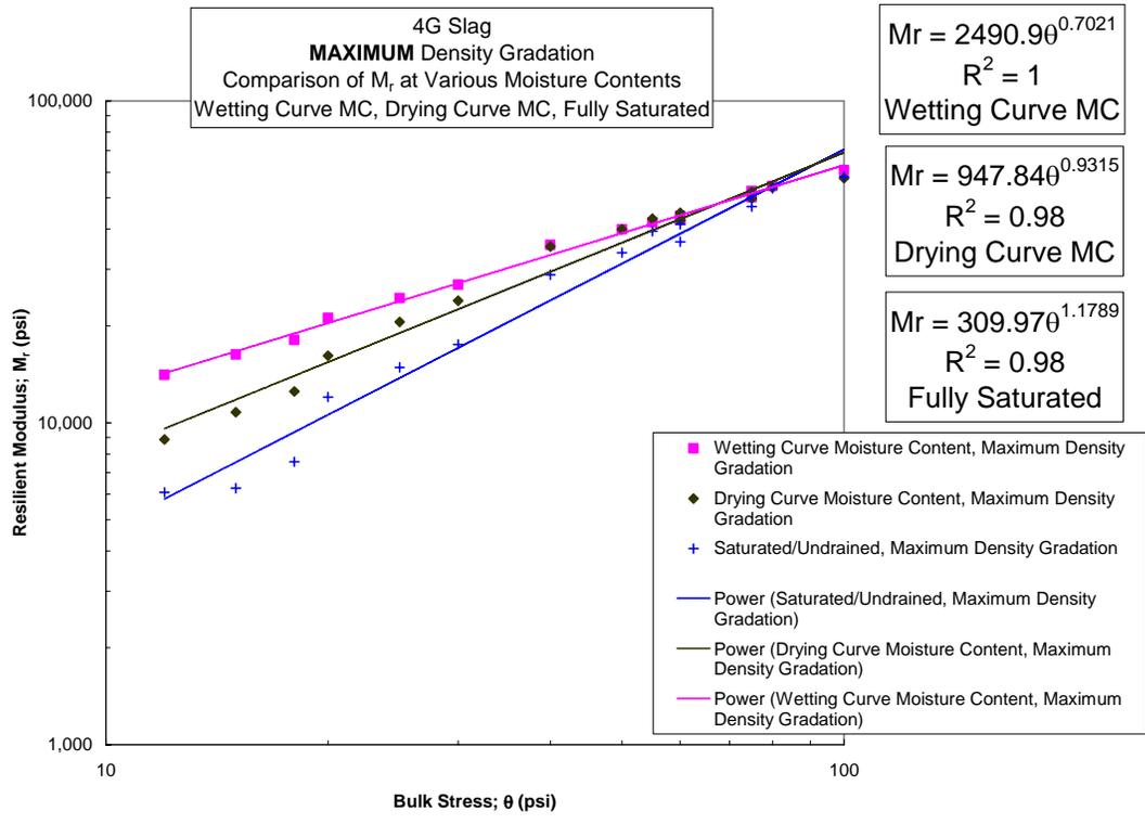
Figure 3.3-18 Slag, Maximum Density Gradations, Wetting and Drying Curve MC, Fully Saturated MC
