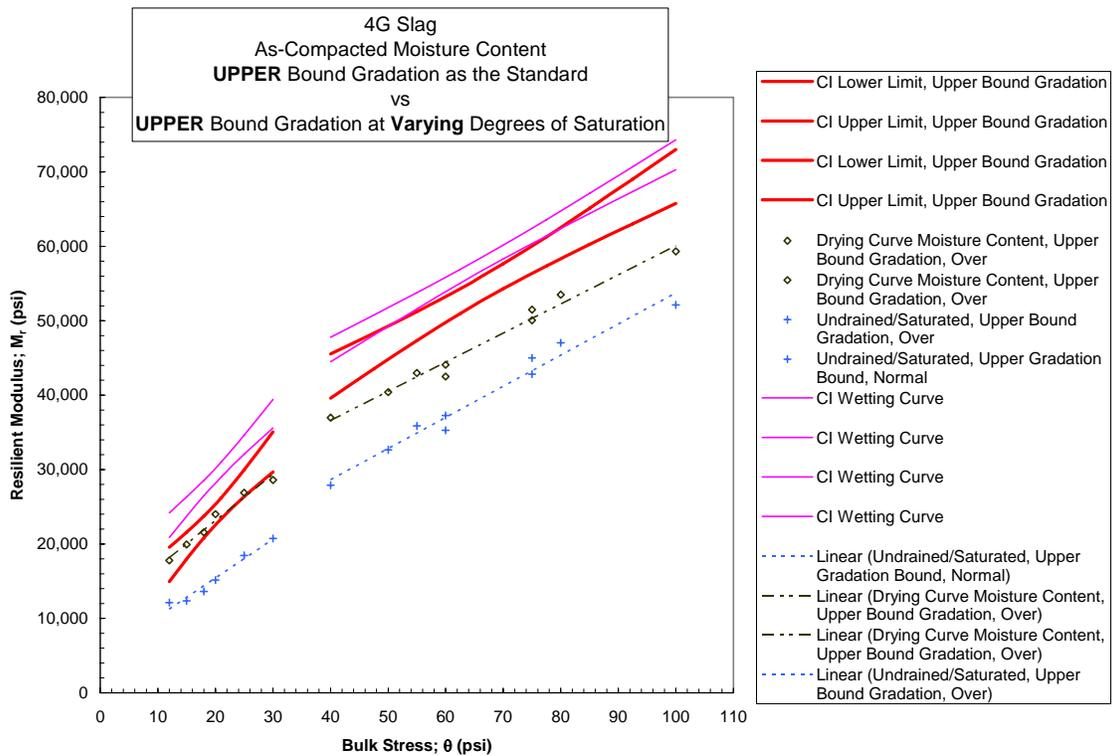
Figure 4.2-18 Slag Upper Bound Gradation Comparing Effect of MC with Wetting Curve MC CI Band
