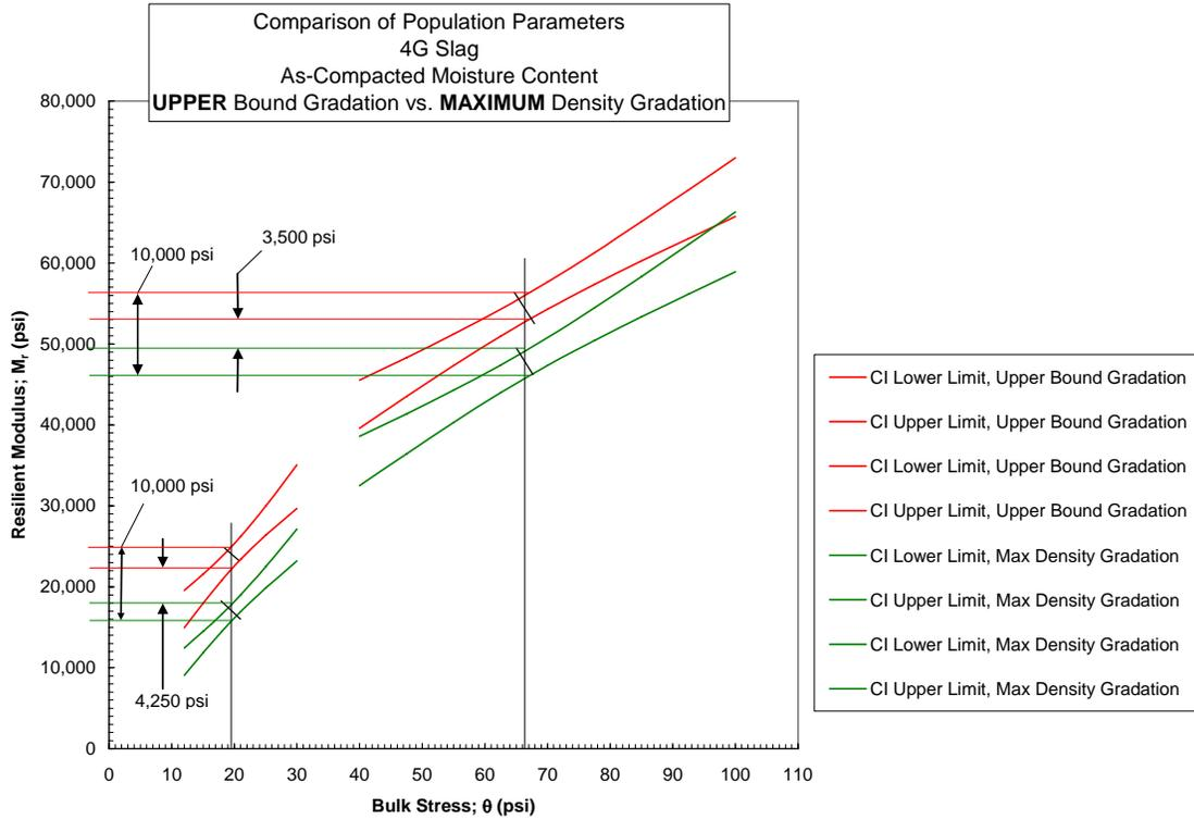
Figure 4.1-21 Stiffness Difference between Upper Bound Gradation and Maximum Density Gradations; Slag
