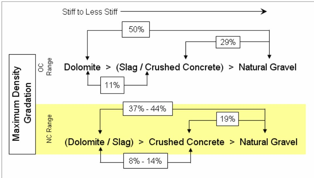
Figure 4.3-9 Quantitative Stiffness Comparison by Material Type for the Maximum Density Gradation
