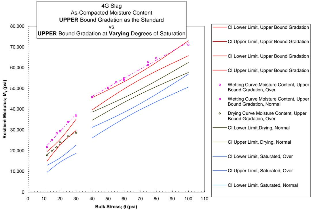
Figure 4.2-19 Slag Upper Bound Gradation Comparing Effect of MC with CI Bands for Drying MC and Fully Saturated MC curves
