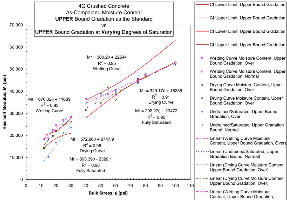
Figure 4.2-24 Crushed Concrete Upper Bound Gradation Comparing Effect of MC
