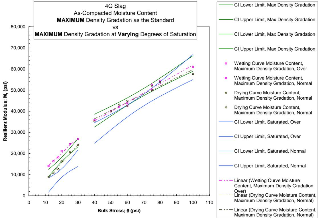
Figure 4.2-21 Slag Maximum Density Gradation Comparing Effect of MC with Fully Saturated CI Band
