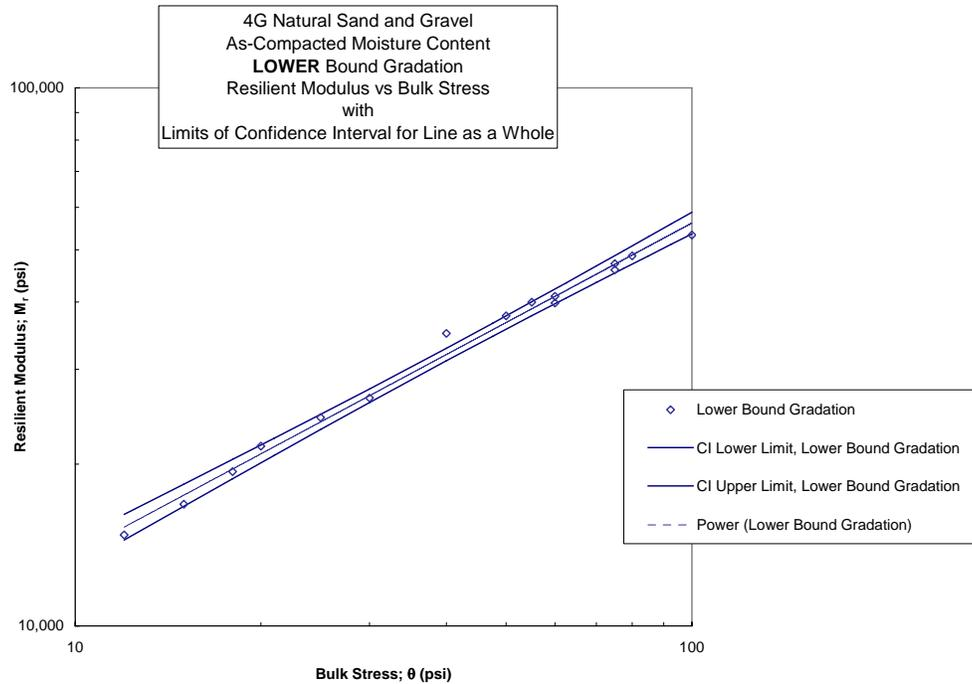
Figure 4.1-4 Resilient Modulus vs Bulk Stress with Limits of 95% Confidence Interval; Log-Log Space
