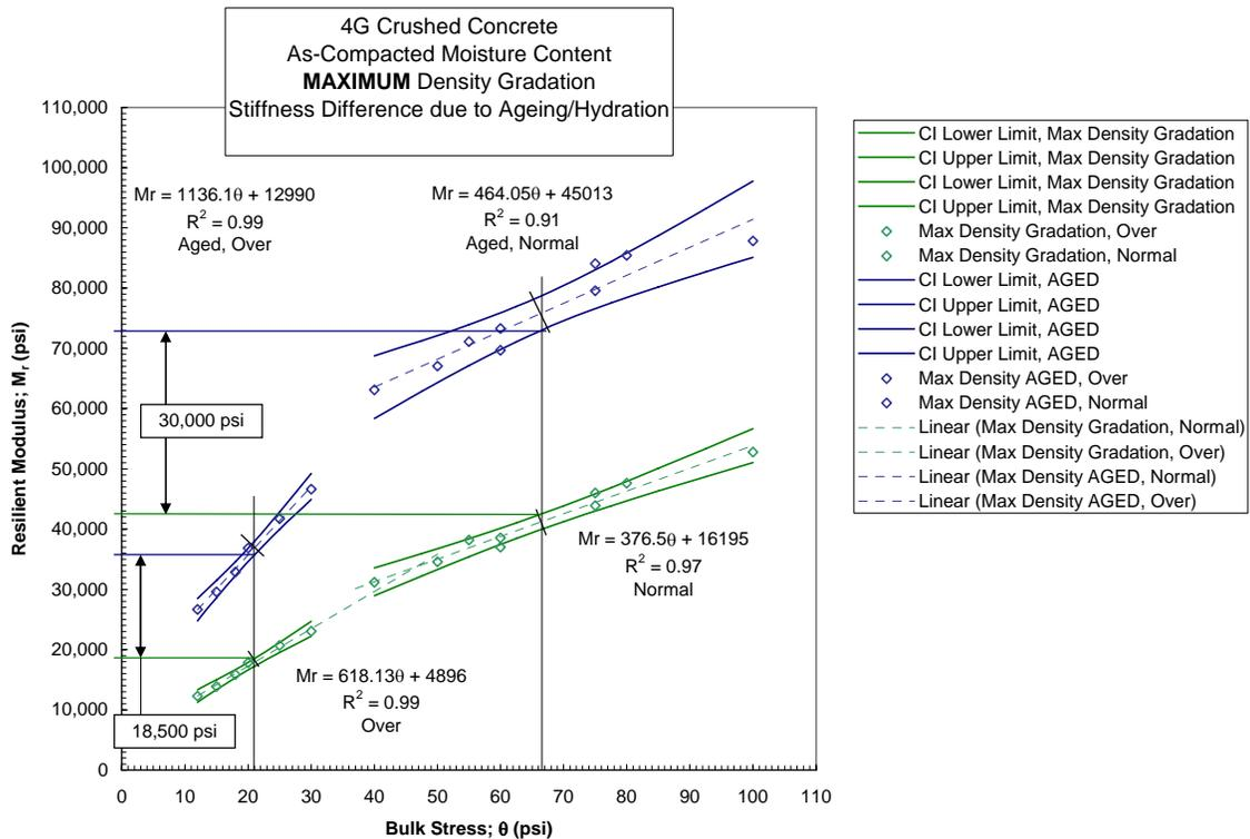
Figure 4.2-27 Increase in Stiffness due to Ageing and Hydration
