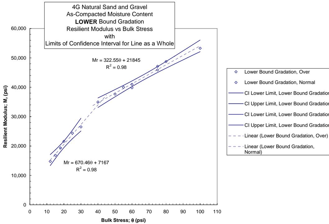
Figure 4.2-1 Resilient Modulus vs Bulk Stress with 95% CI Band - Natural Gravel Lower Bound Gradation Linear-Linear Space
