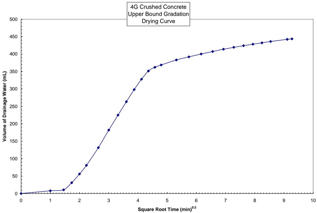
Figure 3.1-12 Drying Curve, Upper Bound Gradation, Crushed Concrete
