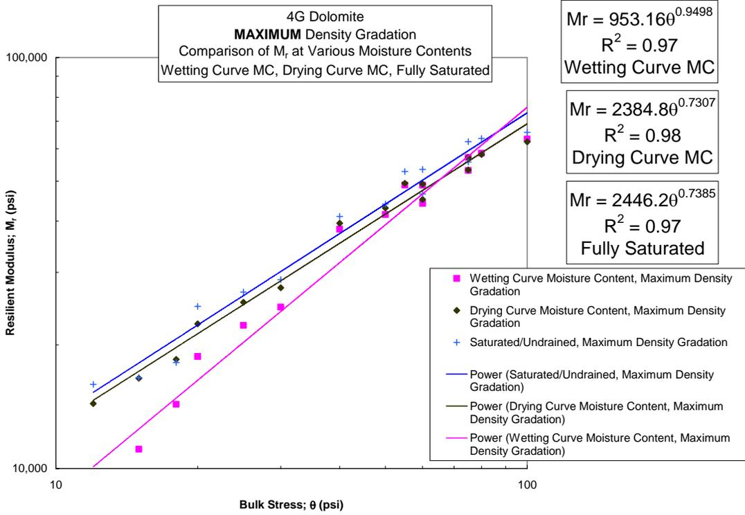
Figure 3.3-12 Dolomite, Maximum Density Gradations, Wetting and Drying Curve MC, Fully Saturated MC
