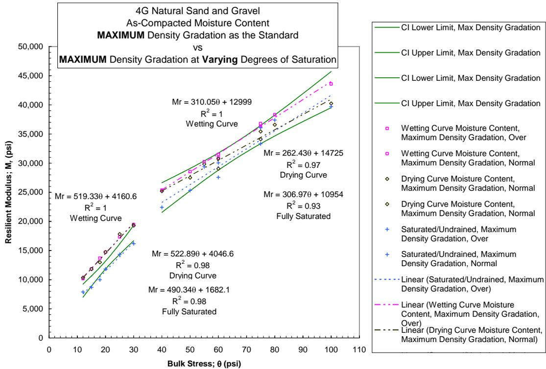
Figure 4.2-9 Natural Gravel Maximum Density Gradation Comparing Effect of MC
