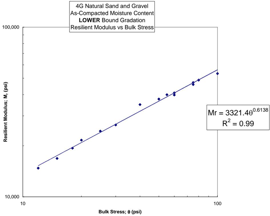
Figure 3.3-1 Natural Gravel, Lower Bound Gradation
