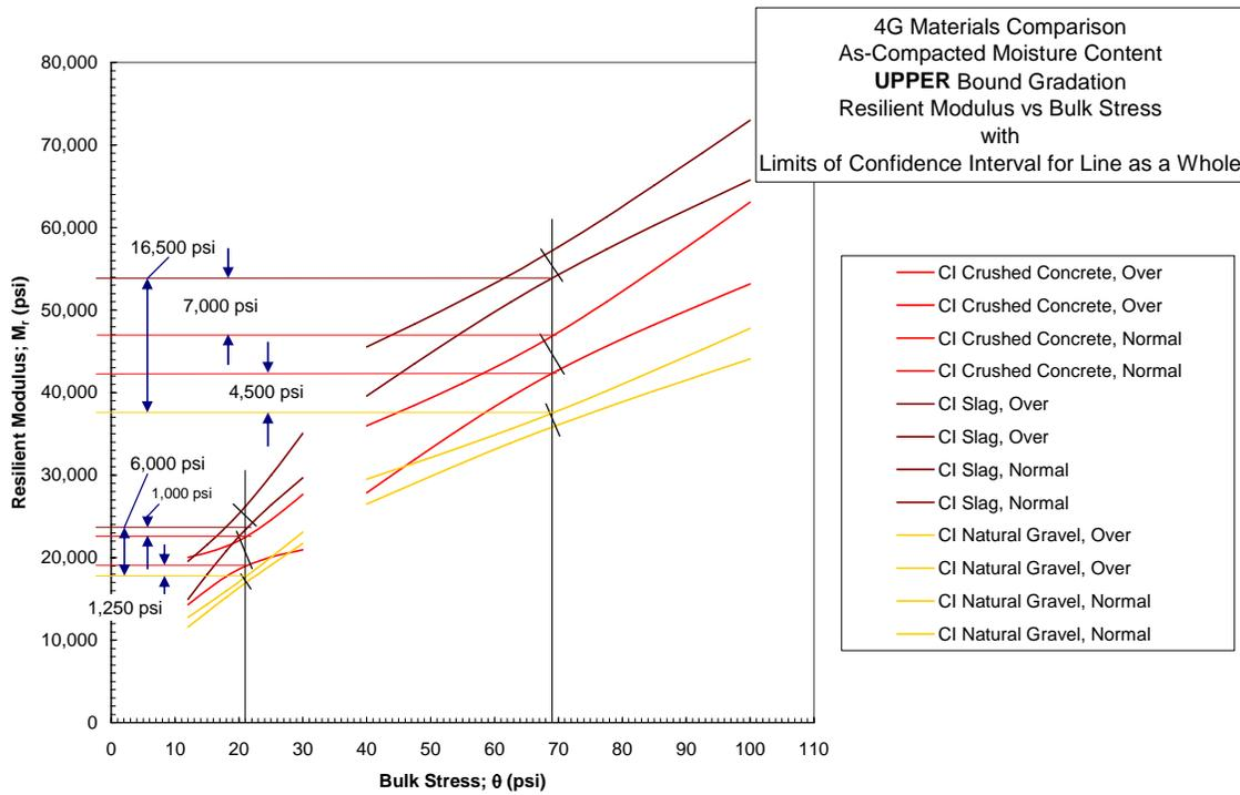
Figure 4.3-3 Upper Bound Gradation Comparing Slag, Crushed Concrete, and Natural Gravel
