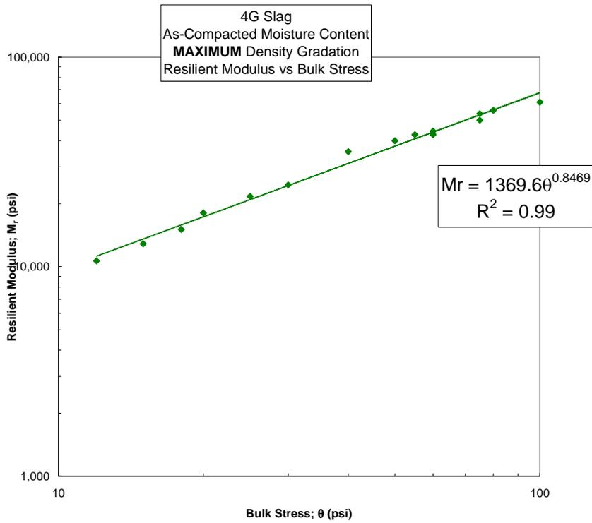
Figure 3.3-15 Slag, Maximum Density Gradation
