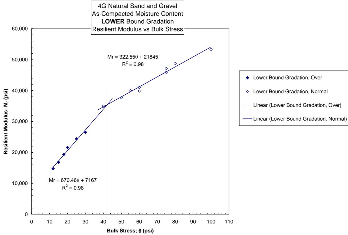
Figure 4.1-10 Natural Gravel Lower Bound Gradation; Linear-Linear Space with Inflection between Overconsolidated State and Normally Consolidated State
