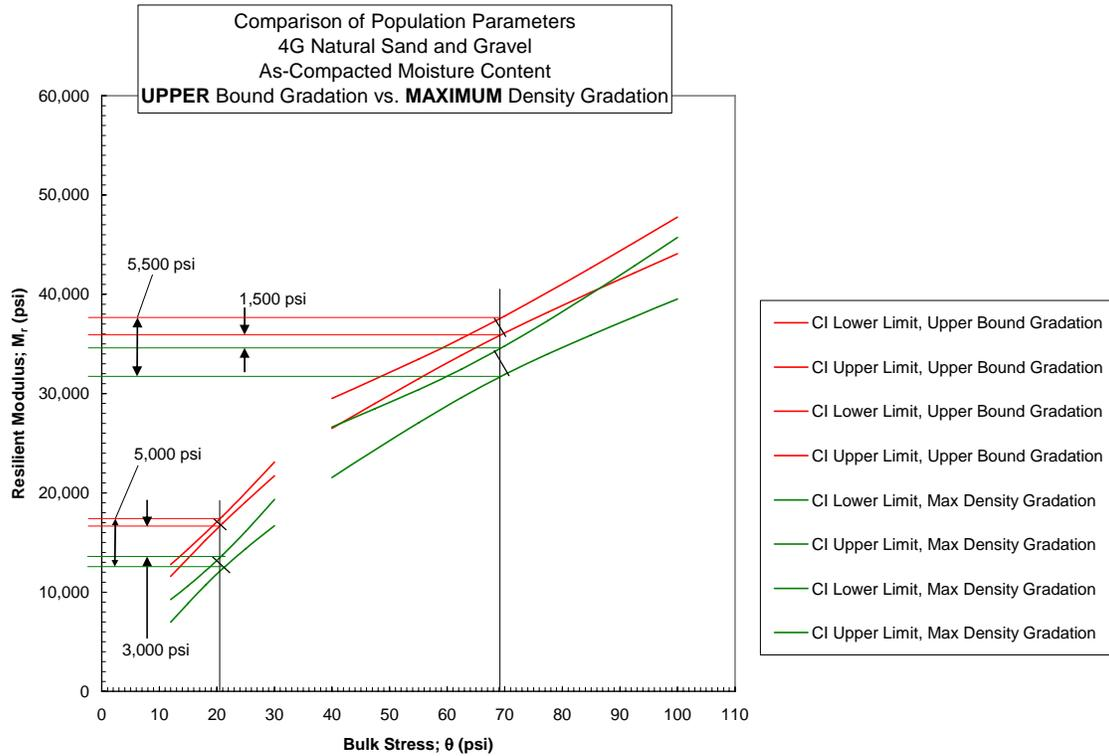
Figure 4.1-15 Stiffness Difference between Upper Bound and Maximum Density Gradations; Natural Gravel
