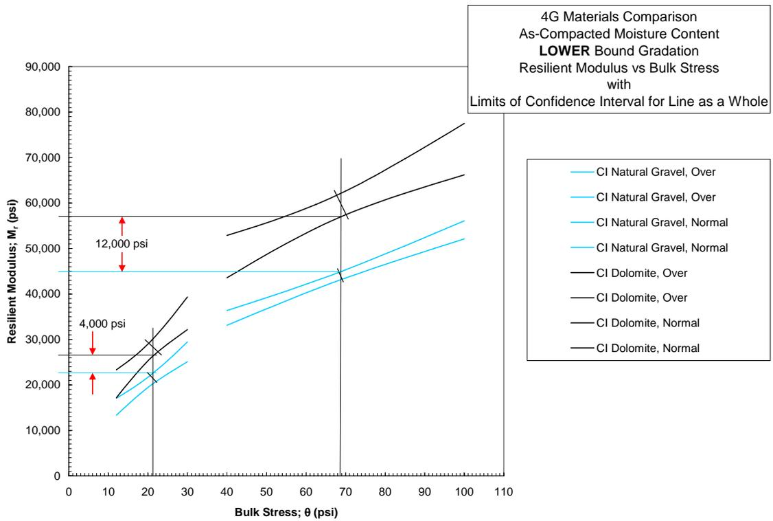
Figure 4.3-2 Lower Bound Gradation Comparing Dolomite and Natural Gravel
