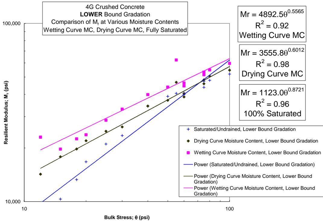
Figure 3.3-22 Crushed Concrete, Lower Bound Gradations, Wetting and Drying Curve MC, Fully Saturated MC
