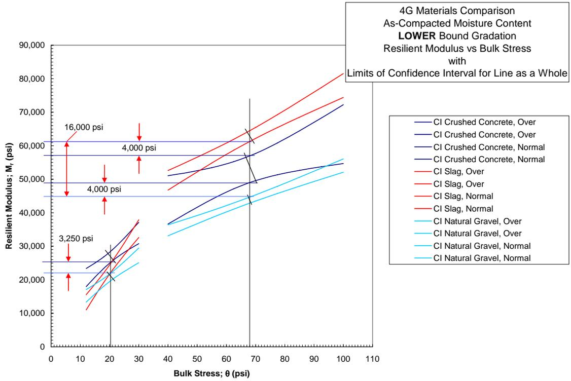
Figure 4.3-1 Lower Bound Gradation Comparing Slag, Crushed Concrete, and Natural Gravel
