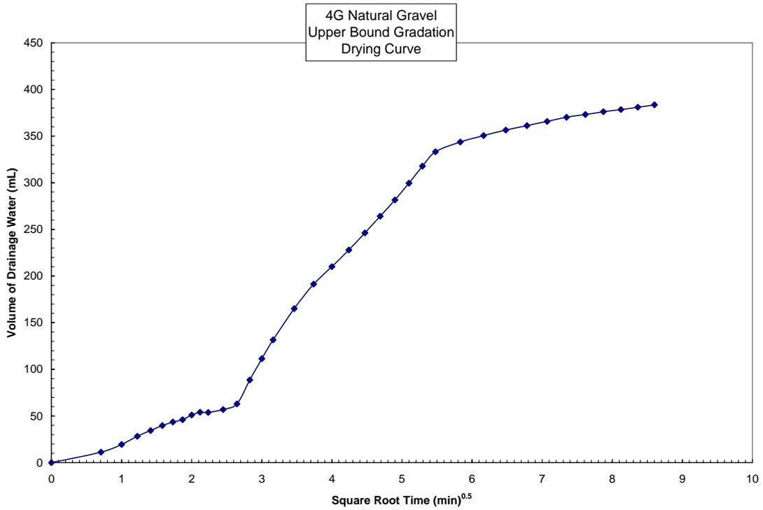
Figure 3.1-2 Drying Curve, Upper Bound Gradation, Natural Gravel
