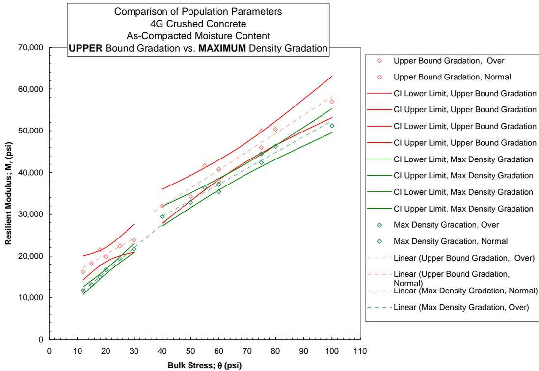
Figure 4.1-24 Stiffness Difference between Upper Bound and Maximum Density Gradations; Crushed Concrete
