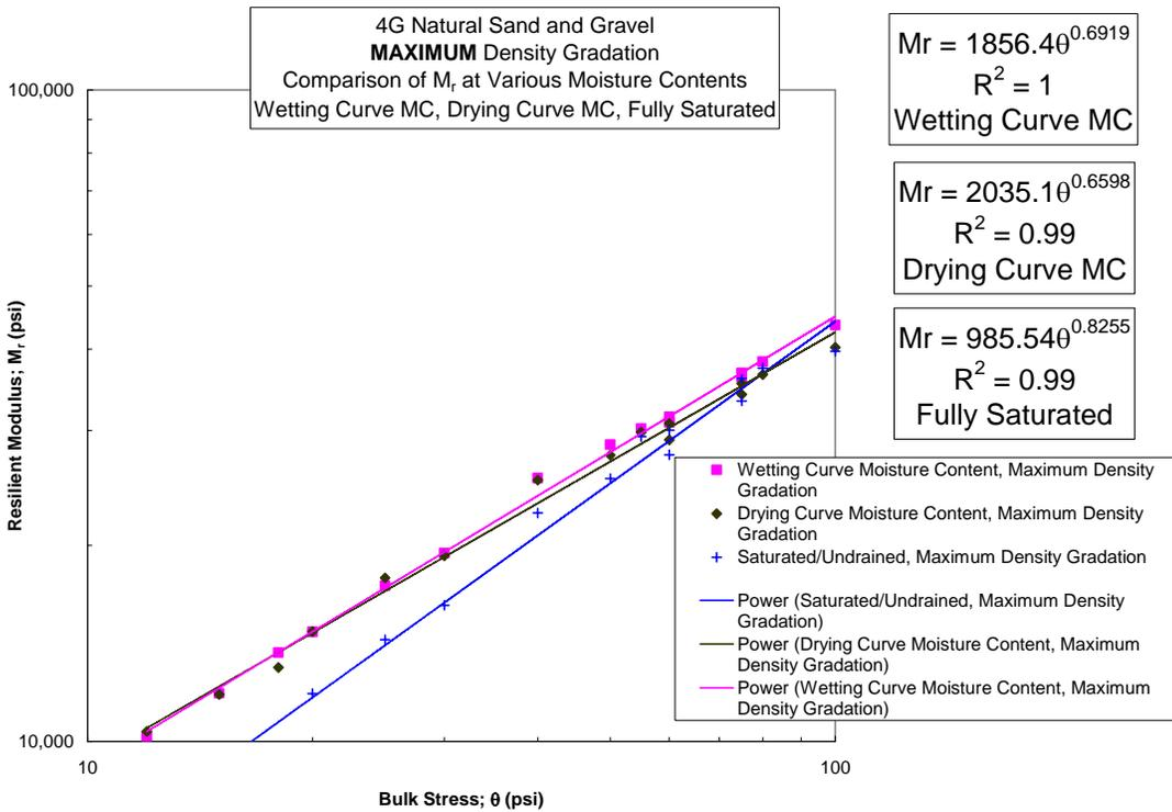
Figure 3.3-6 Natural Gravel, Maximum Density Gradations, Wetting and Drying Curve MC, Fully Saturated MC
