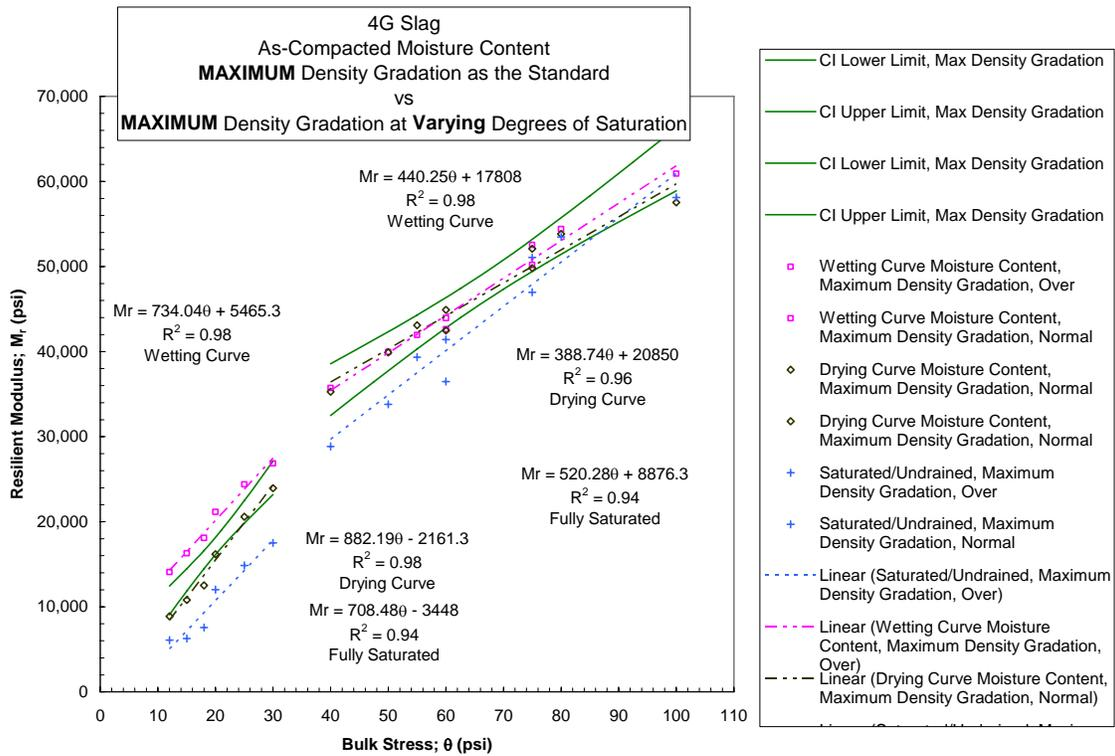
Figure 4.2-20 Slag Maximum Density Gradation Comparing Effect of MC
