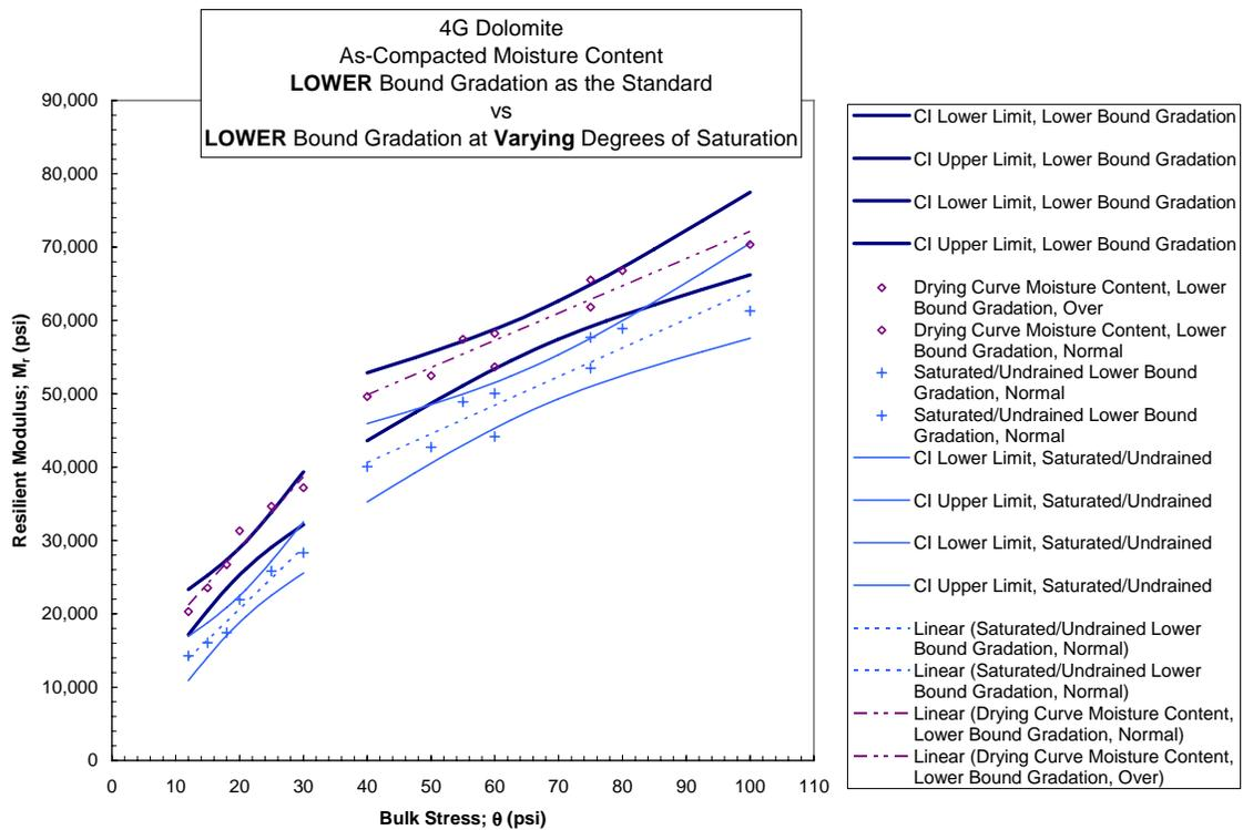
Figure 4.2-11 Dolomite Lower Bound Gradation Comparing Effect of MC with Fully Saturated CI Band
