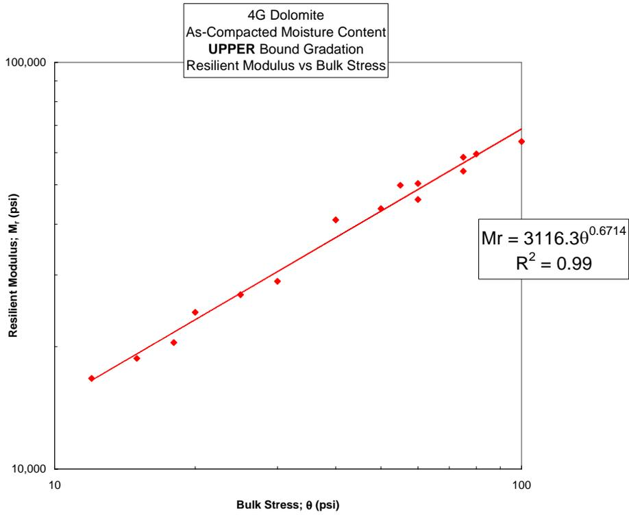
Figure 3.3-8 Dolomite, Upper Bound Gradation
