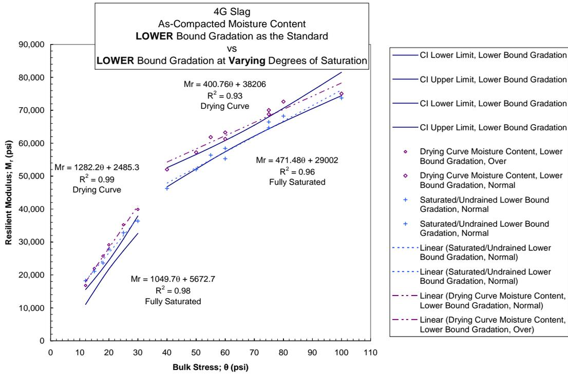
Figure 4.2-15 Slag Lower Bound Gradation Comparing Effect of MC
