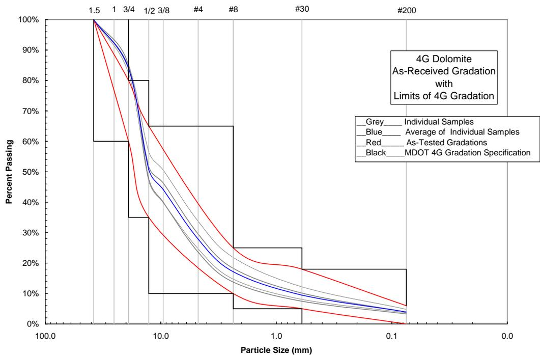
Figure 2.2-2 As-Received and As-Tested Gradations; 4G Dolomite
