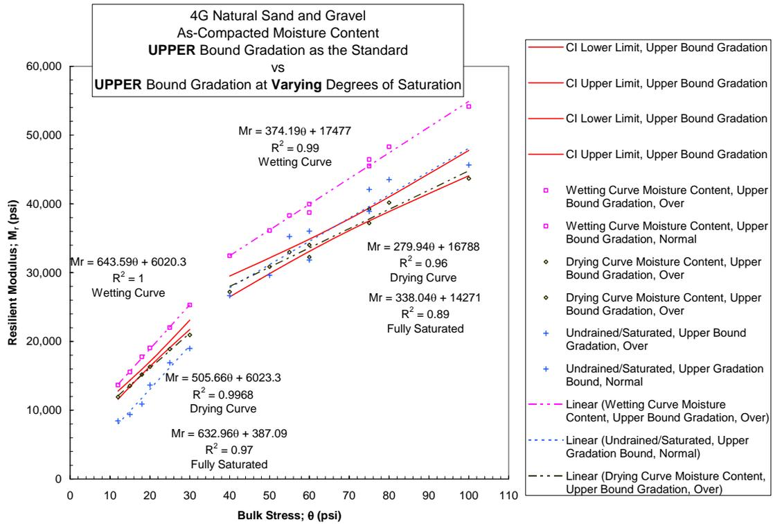
Figure 4.2-7 Natural Gravel Upper Bound Gradation Comparing Effect of MC
