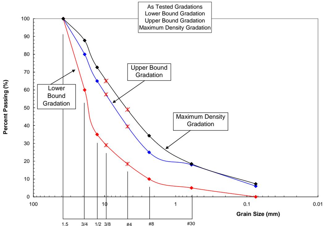
Figure 4.1-1 Lower and Upper Bounds of 4G Gradation Curves and the Curve of Maximum Density
