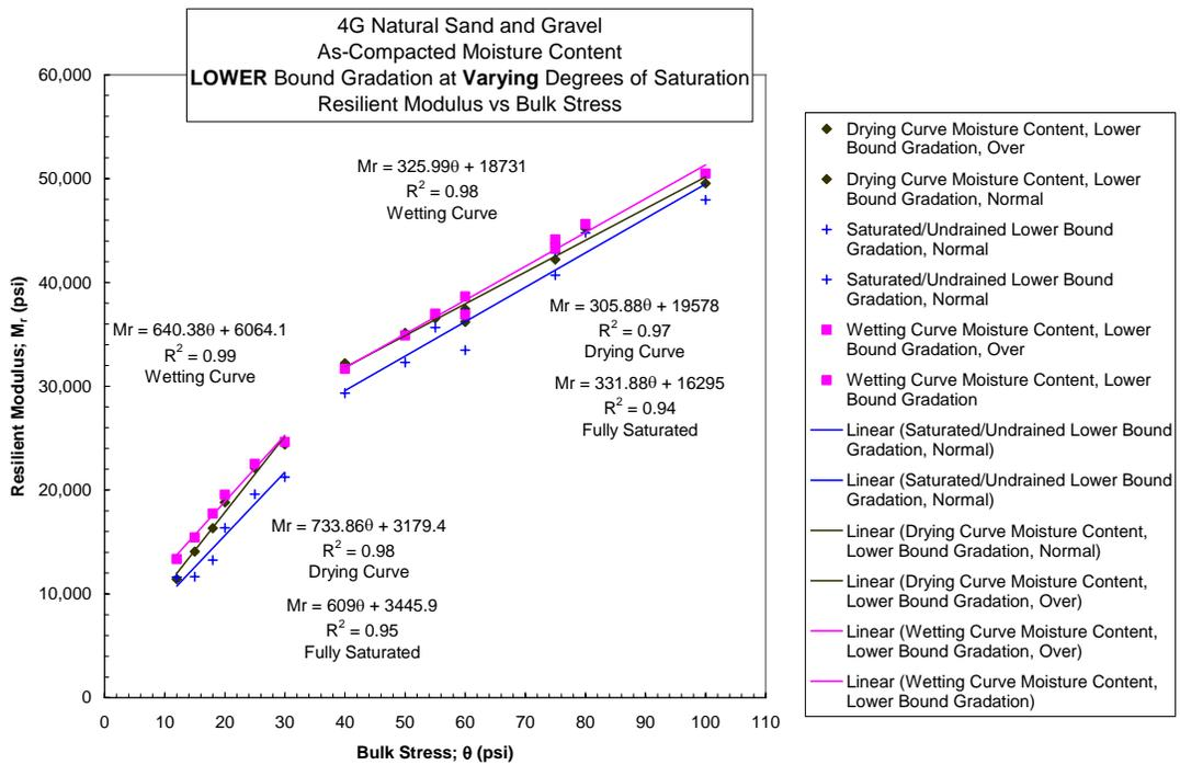
Figure 4.2-3 Resilient Modulus Curves for Wetting Curve MC, Drying Curve MC, and Fully Saturated MC. Natural Gravel Lower Bound Gradation; Linear-Linear Space
