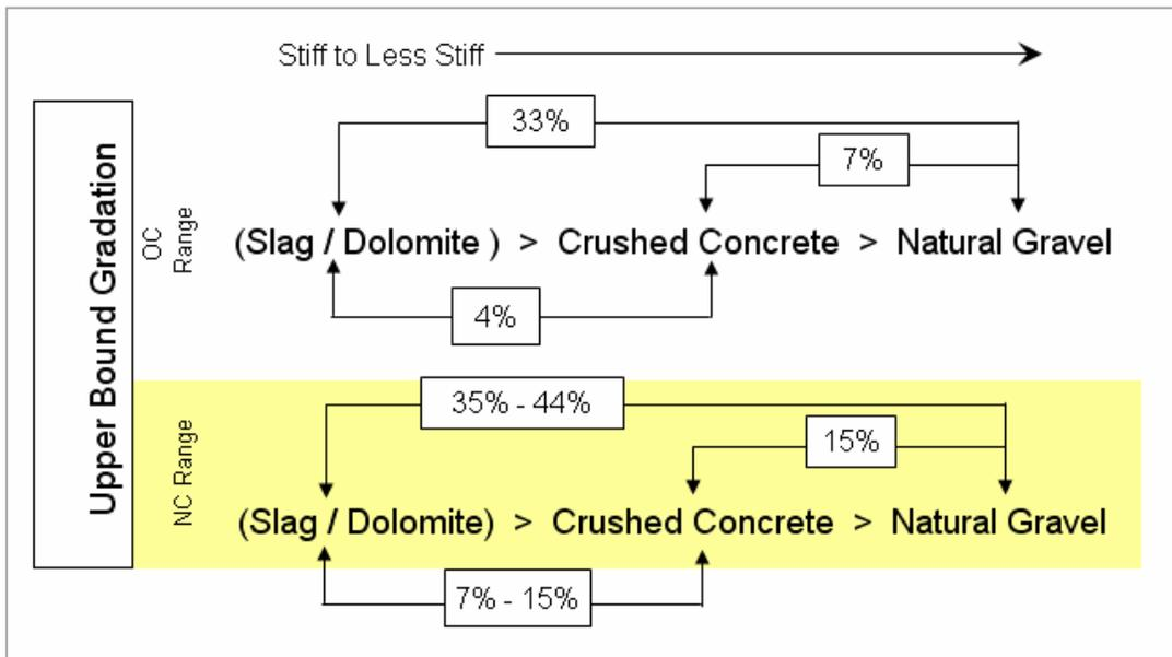
Figure 4.3-8 Quantitative Stiffness Comparison by Material Type for the Upper Bound Gradation
