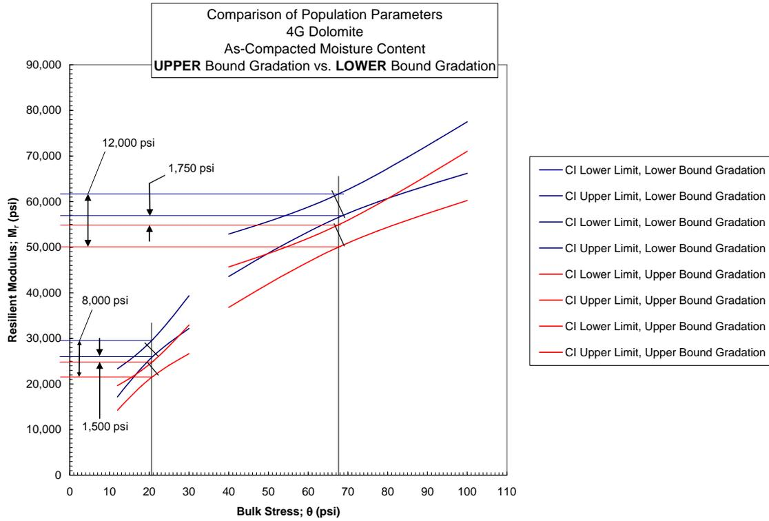
Figure 4.1-17 Stiffness Difference between Upper and Lower Bound Gradations; Dolomite
