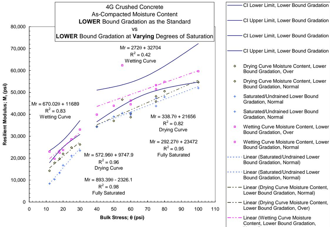
Figure 4.2-22 Crushed Concrete Lower Bound Gradation Comparing Effect of MC
