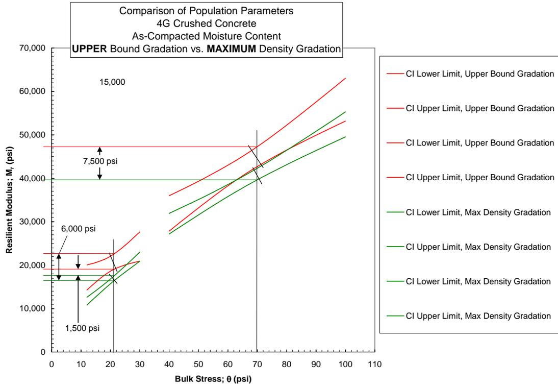
Figure 4.1-25 Stiffness Difference between Upper Bound Gradation and Maximum Density Gradations; Crushed Concrete
