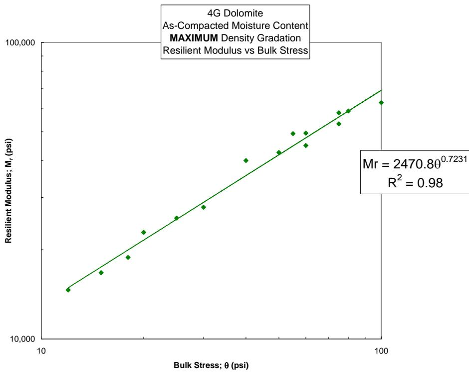
Figure 3.3-9 Dolomite, Maximum Density Gradation
