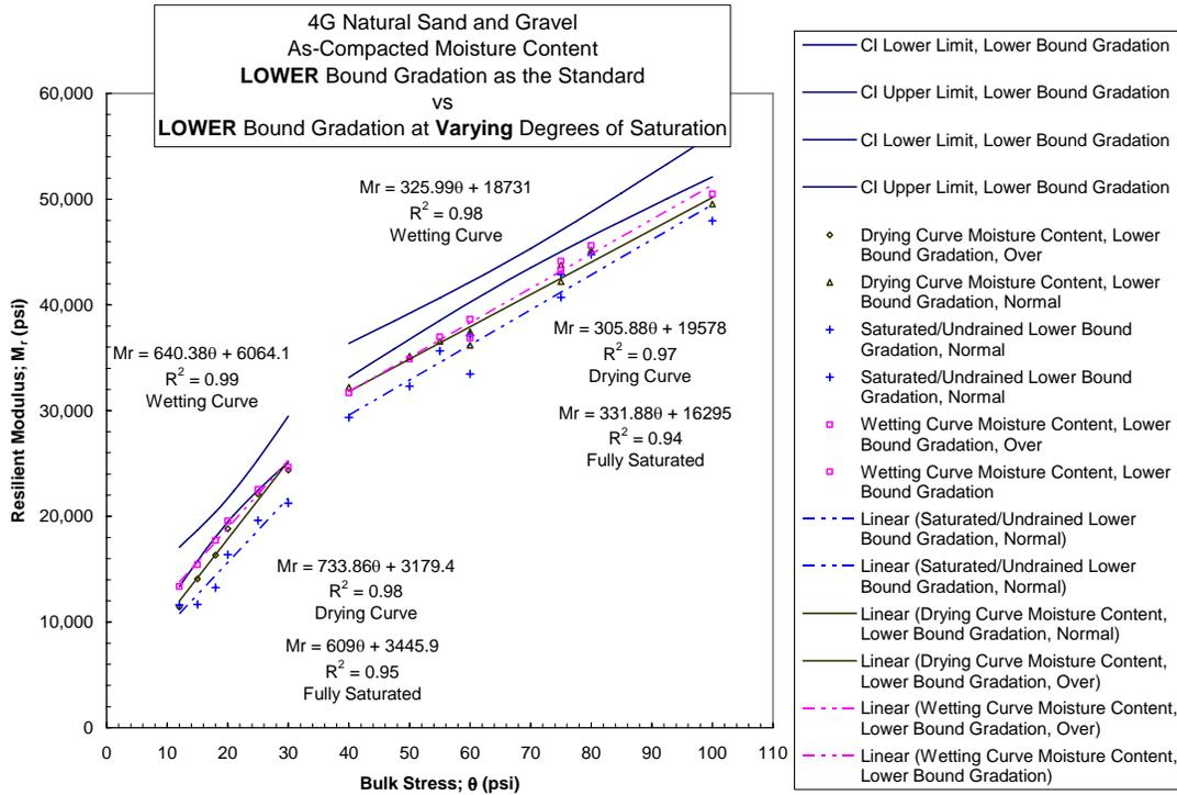
Figure 4.2-4 Resilient Modulus Curves for Wetting Curve MC, Drying Curve MC, and Fully Saturated MC with CI Band for as-compacted MC. Natural Gravel Lower Bound Gradation; Linear-Linear Space
