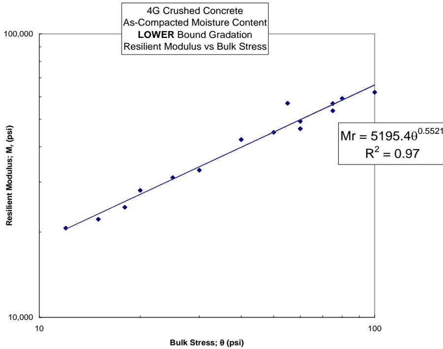
Figure 3.3-19 Crushed Concrete, Lower Bound Gradation
