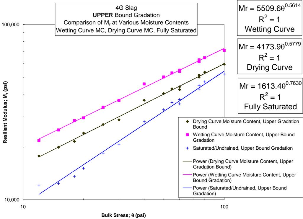
Figure 3.3-17 Slag, Upper Bound Gradations, Wetting and Drying Curve MC, Fully Saturated MC
