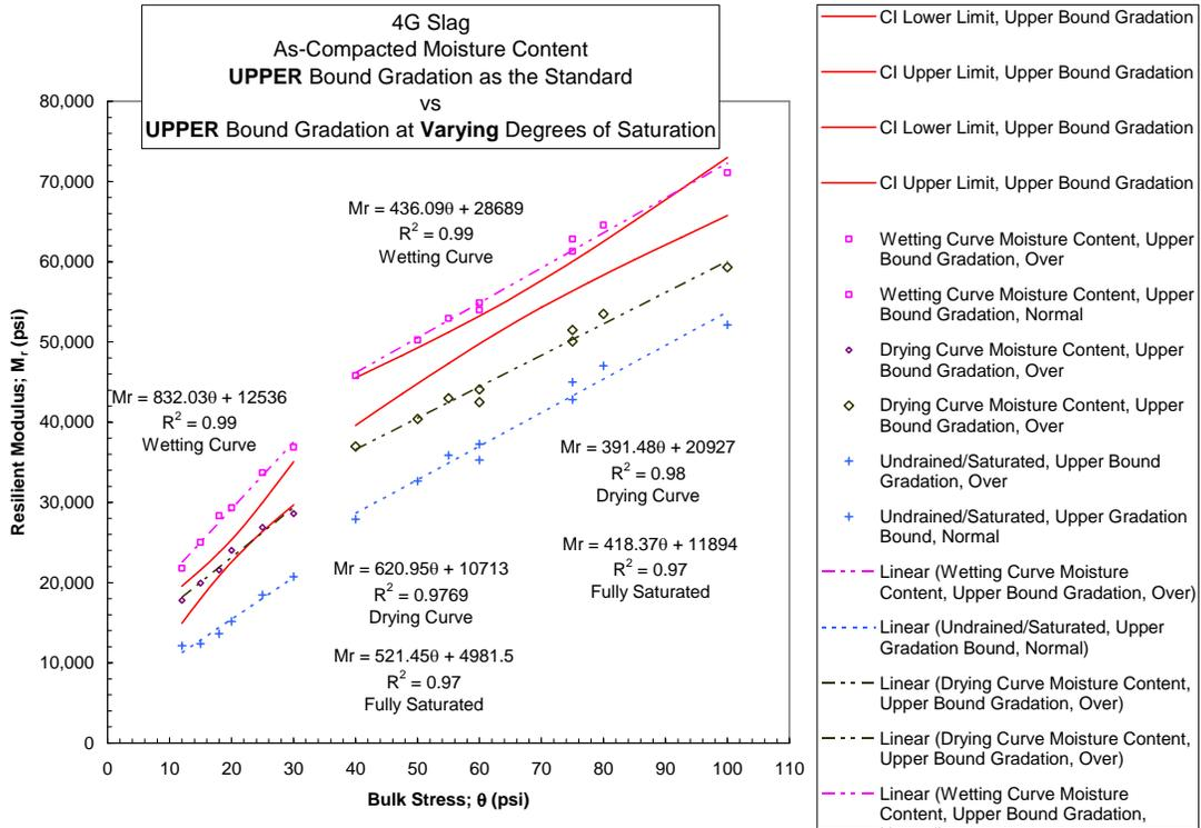
Figure 4.2-17 Slag Upper Bound Gradation Comparing Effect of MC
