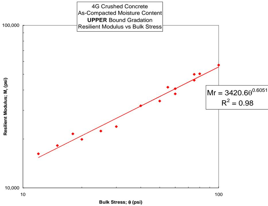
Figure 3.3-20 Crushed Concrete, Upper Bound Gradation
