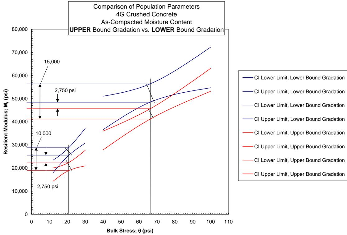
Figure 4.1-23 Stiffness Difference between Upper and Lower Bound Gradations; Crushed Concrete
