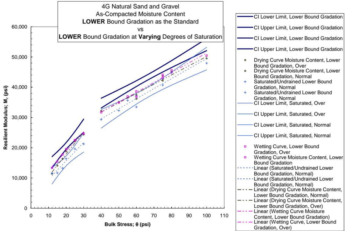
Figure 4.2-6 Natural Gravel Lower Bound Gradation Comparing Effect of MC with Fully Saturated MC CI Band
