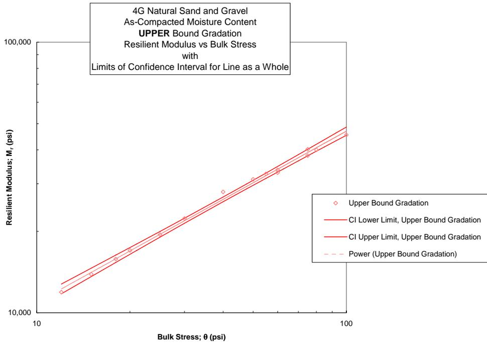
Figure 4.1-5 Resilient Modulus vs Bulk Stress with Limits of 95% Confidence Interval; Log-Log Space
