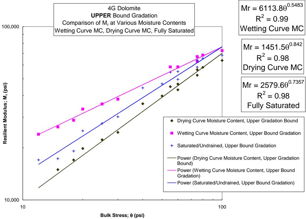
Figure 3.3-11 Dolomite, Upper Bound Gradations, Wetting and Drying Curve MC, Fully Saturated MC
