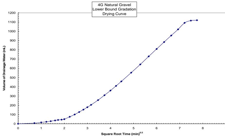
Figure 3.1-1 Drying Curve, Lower Bound Gradation, Natural Gravel
