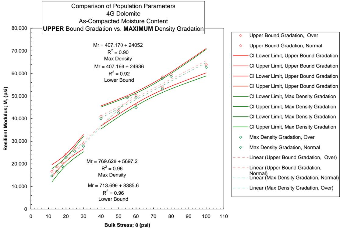
Figure 4.1-18 Stiffness Difference between Upper Bound Gradation and Maximum Density Gradations; Dolomite
