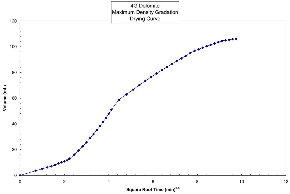
Figure 3.1-7 Drying Curve, Maximum Density Gradation, Dolomite
