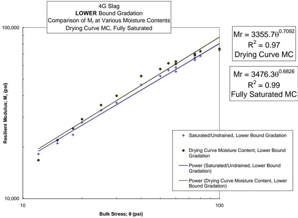
Figure 3.3-16 Slag, Lower Bound Gradations, Drying Curve MC, Fully Saturated MC
