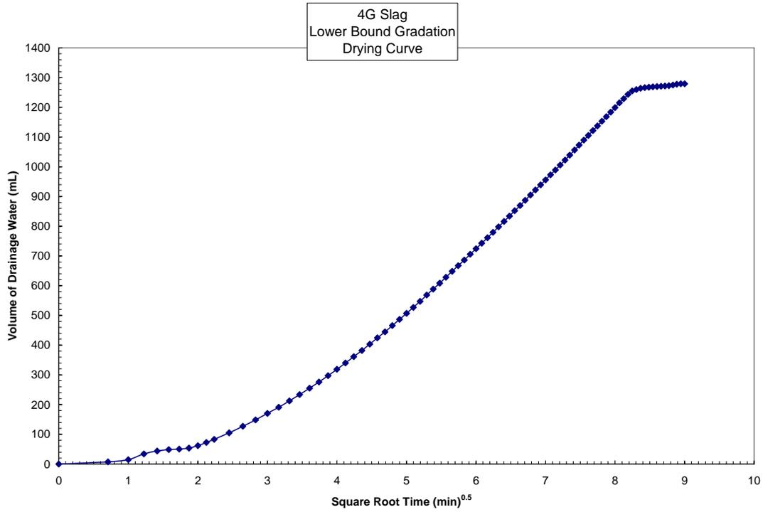
Figure 3.1-8 Drying Curve, Lower Bound Gradation, Slag
