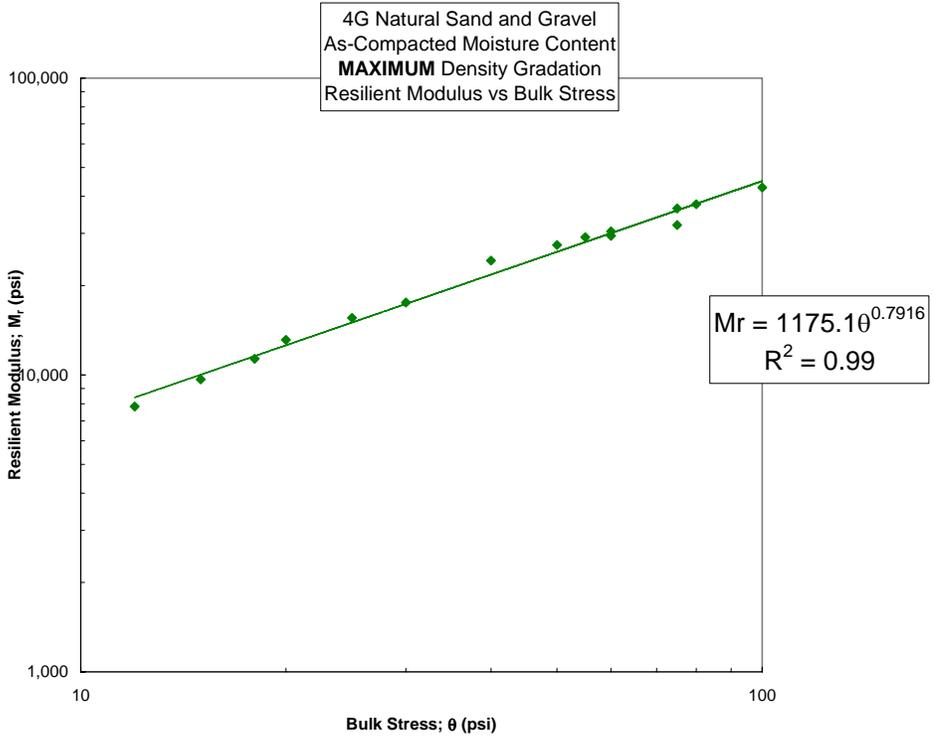
Figure 3.3-3 Natural Gravel, Maximum Density Gradation
