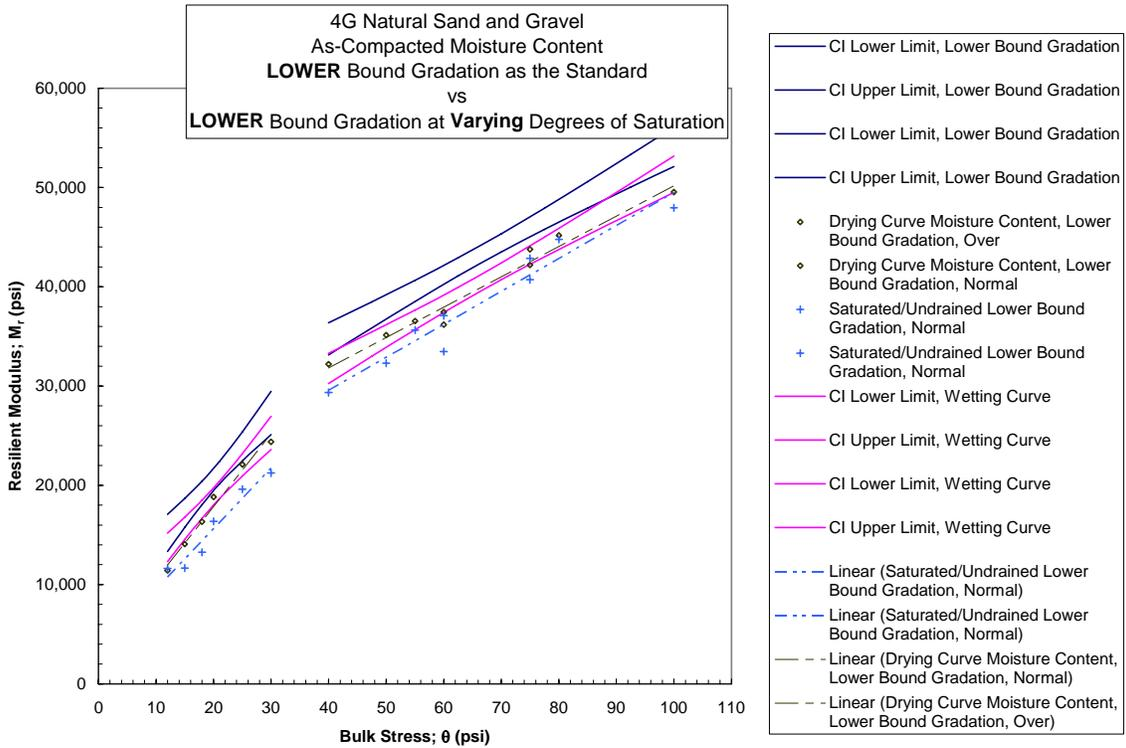
Figure 4.2-5 Natural Gravel Lower Bound Gradation Comparing Effect of MC with Wetting Curve MC CI Band
