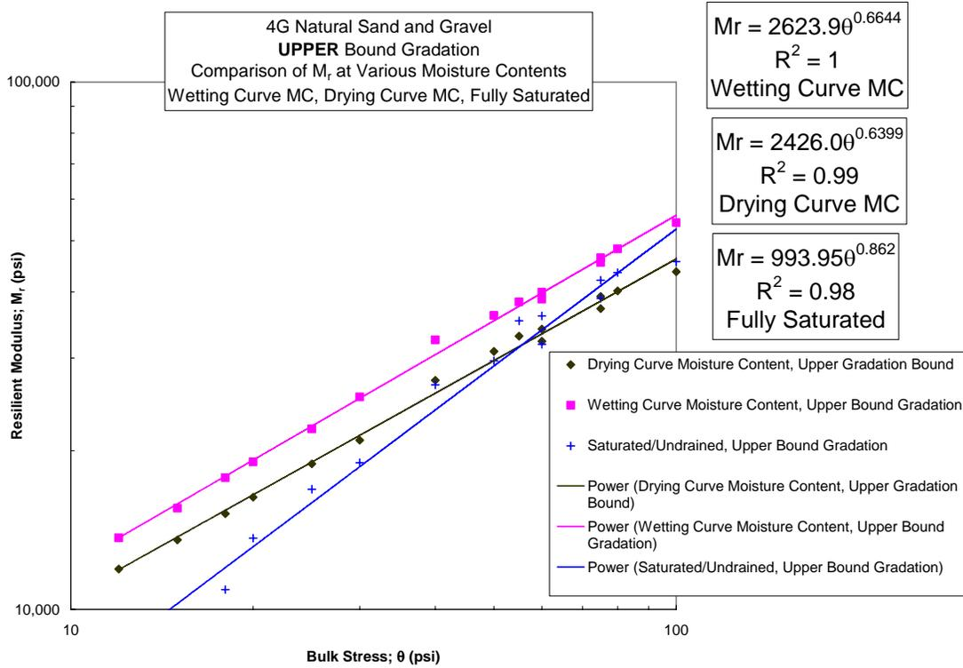
Figure 3.3-5 Natural Gravel, Upper Bound Gradations, Wetting and Drying Curve MC, Fully Saturated MC
