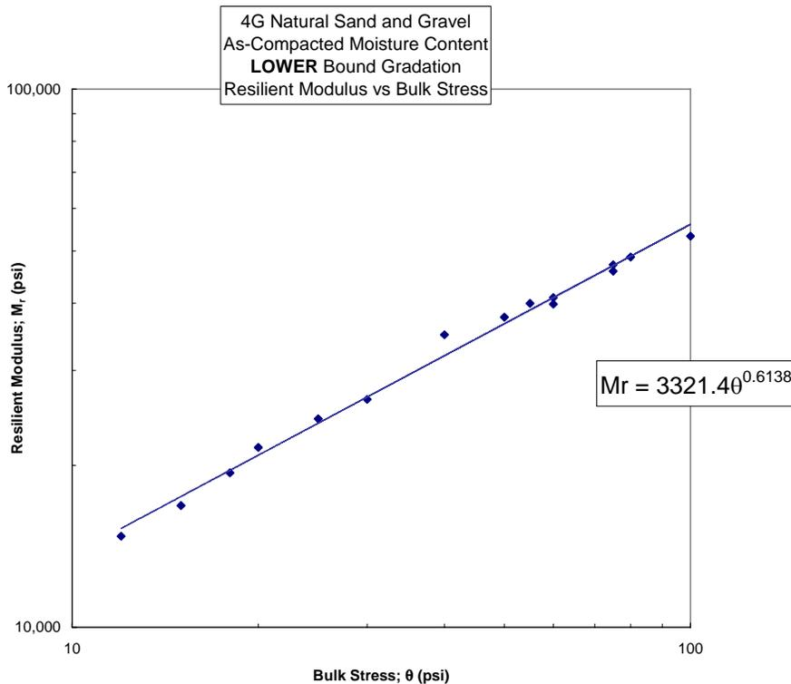
Figure 4.1-2 Natural Gravel Resilient Modulus vs Bulk Stress; Log-Log Space
