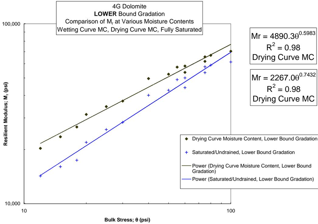
Figure 3.3-10 Dolomite, Lower Bound Gradations, Drying Curve MC, Fully Saturated MC
