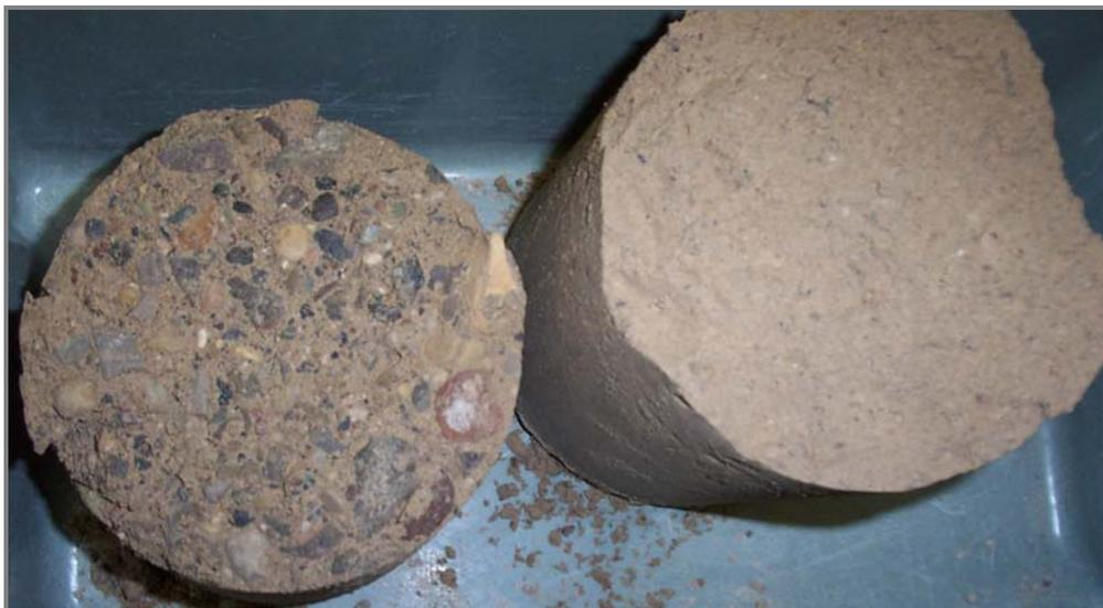
Figure 2.3-1 Example of Fines and Fine Aggregate Migration and Segregation at Lift Interfaces
