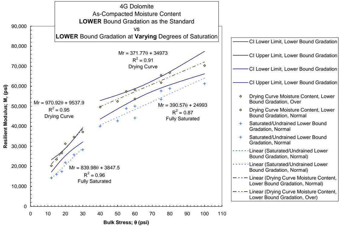
Figure 4.2-10 Dolomite Lower Bound Gradation Comparing Effect of MC
