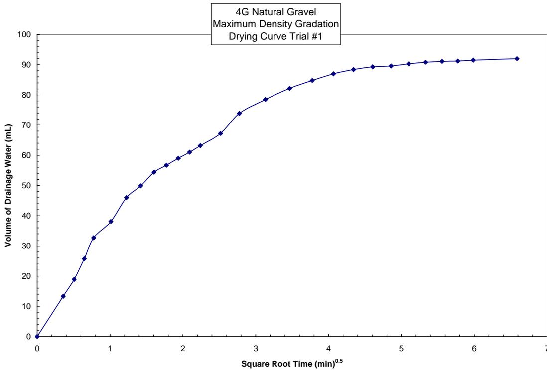
Figure 3.1-3 Drying Curve, Maximum Density Gradation, Natural Gravel Trial no. 1
