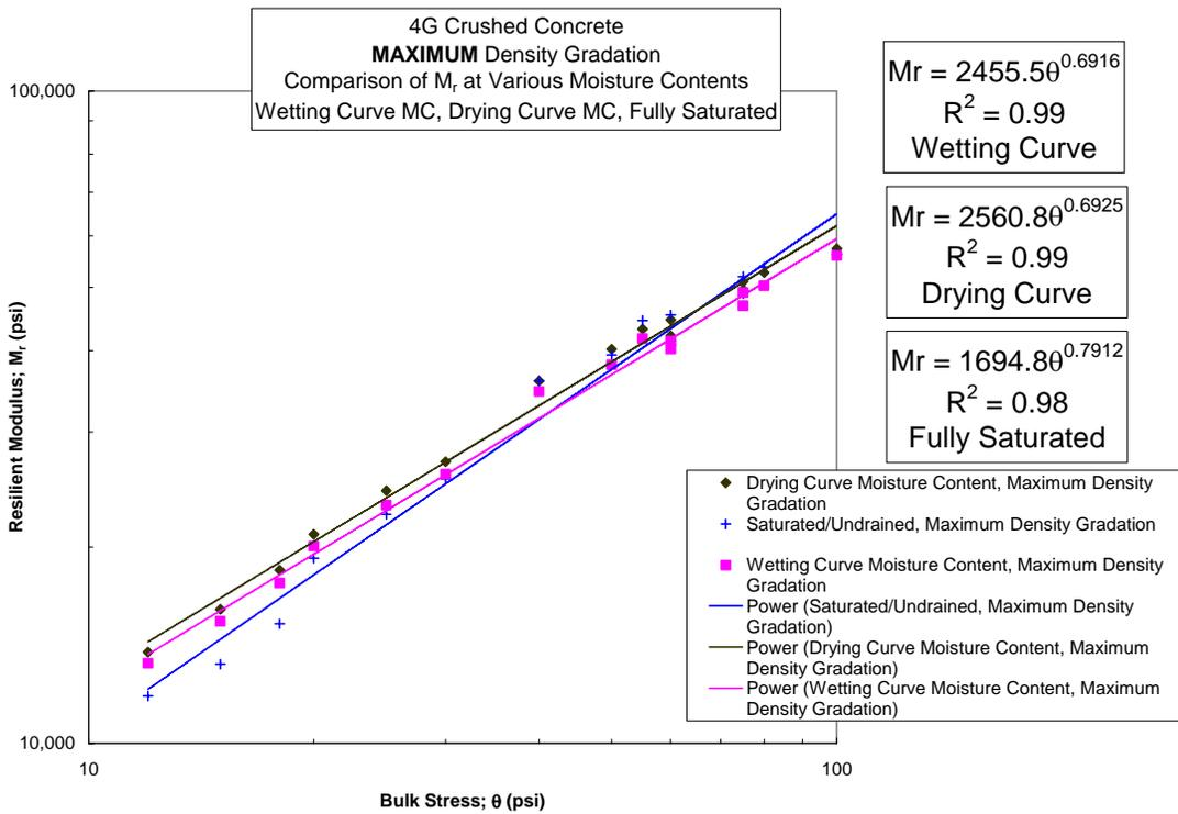
Figure 3.3-24 Crushed Concrete, Maximum Density Gradations, Wetting Curve MC, Drying Curve MC, Fully Saturated MC
