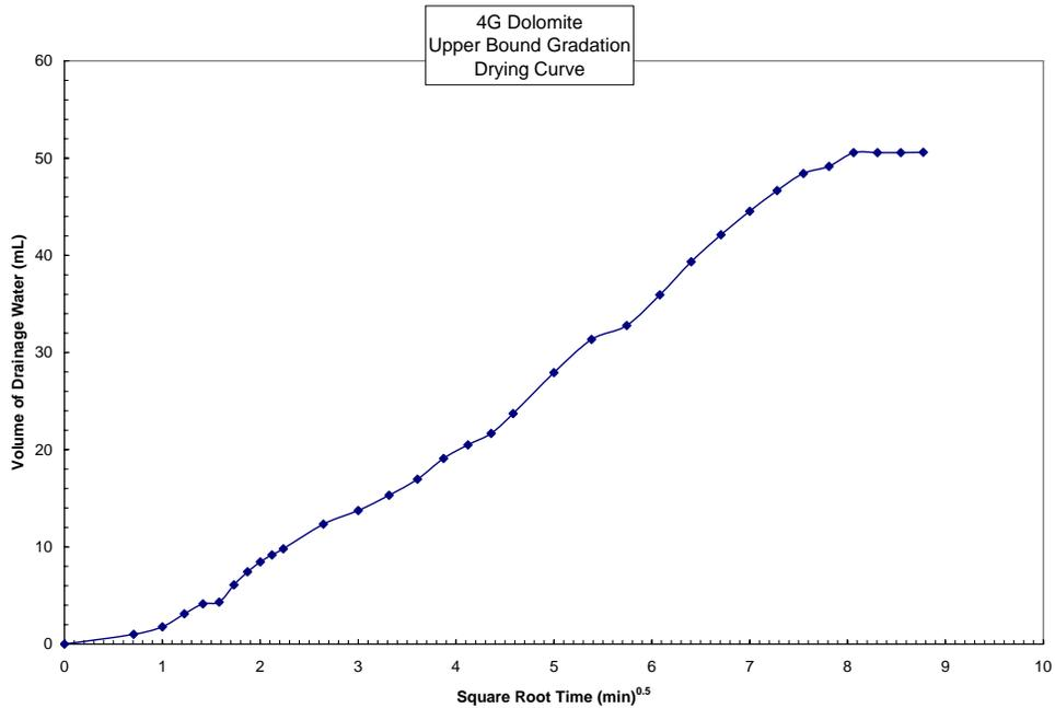
Figure 3.1-6 Drying Curve, Upper Bound Gradation, Dolomite
