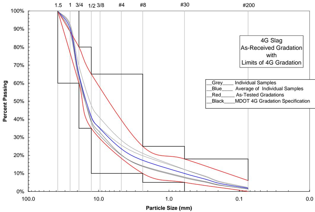
Figure 2.2-3 As-Received and As-Tested Gradations; 4G Slag
