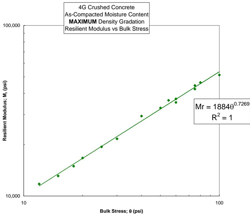
Figure 3.3-21 Crushed Concrete, Maximum Density Gradation
