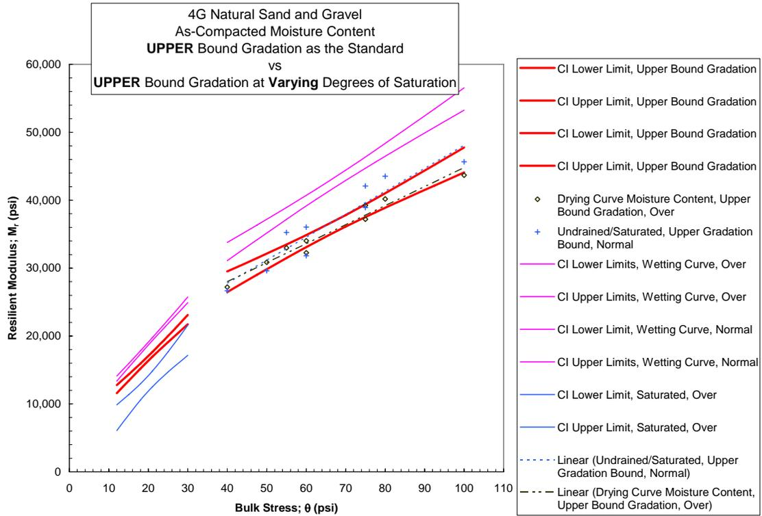
Figure 4.2-8 Natural Gravel Upper Bound Gradation Comparing Effect of MC with Wetting Curve MC CI Band and Full Saturated MC CI Band (overconsolidated region)
