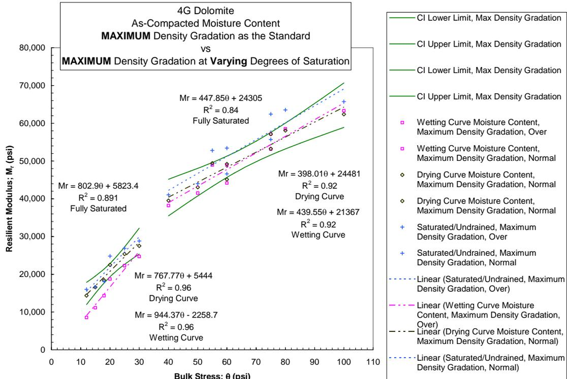
Figure 4.2-14 Dolomite Maximum Density Gradation Comparing Effect of MC
