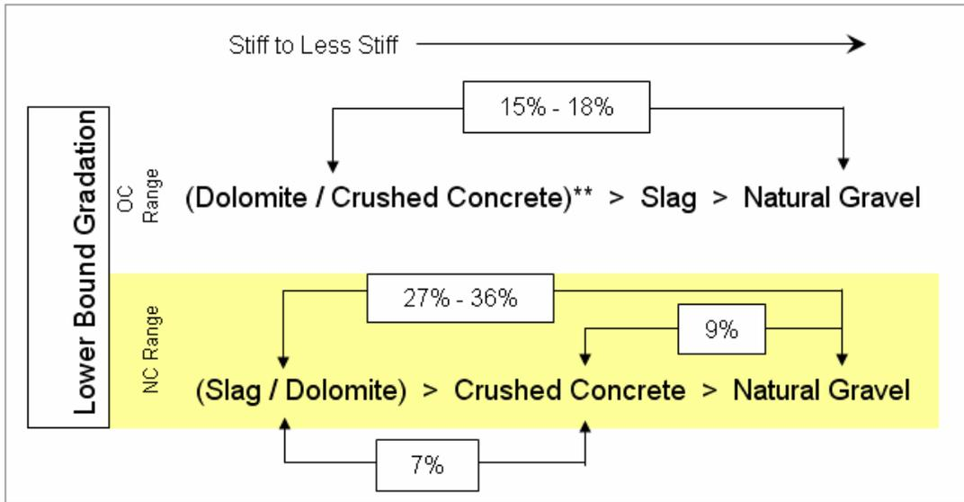
Figure 4.3-7 Quantitative Stiffness Comparison by Material Type for the Lower Bound Gradation
