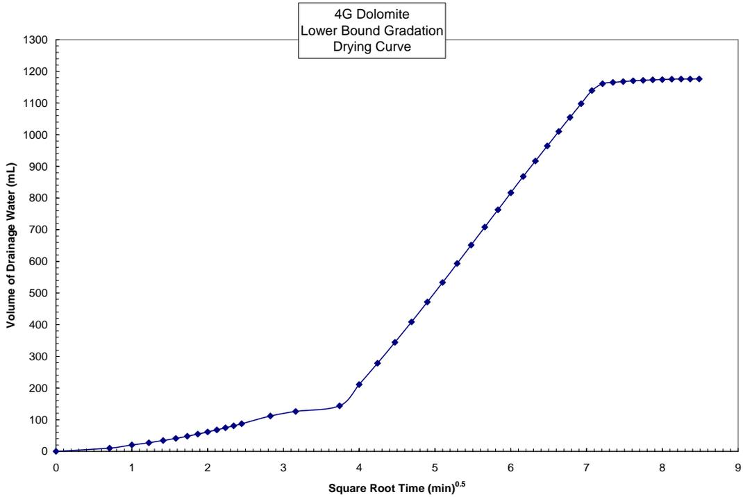
Figure 3.1-5 Drying Curve, Lower Bound Gradation, Dolomite
