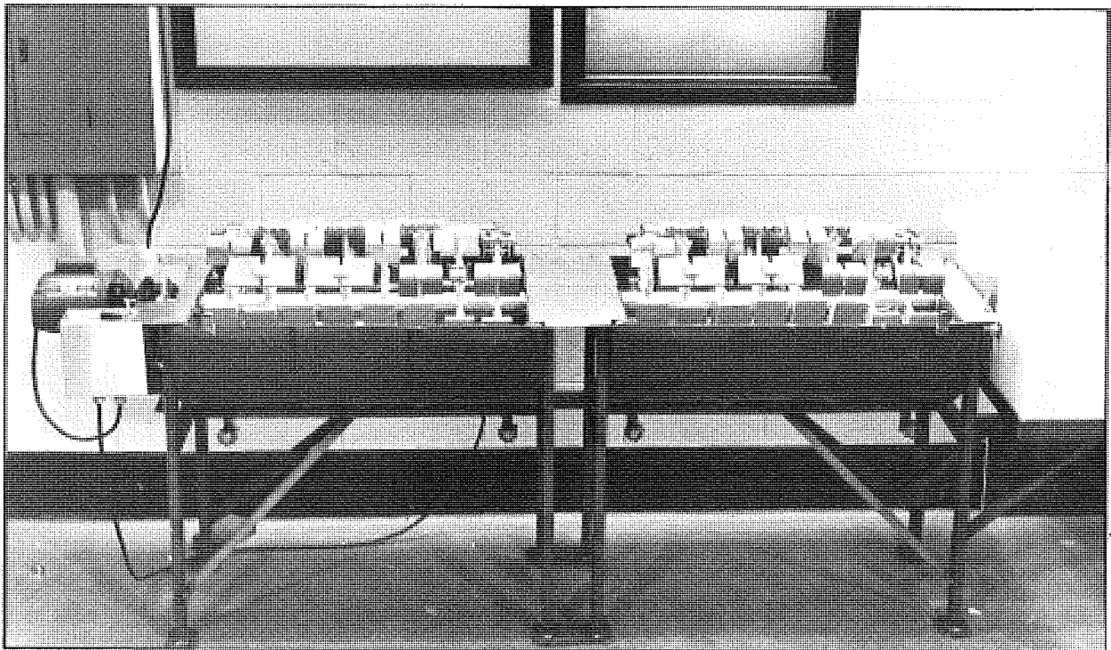
b) With hood removed and specimen exposed (in this instance with CMA on the left and NaCl on the right).
