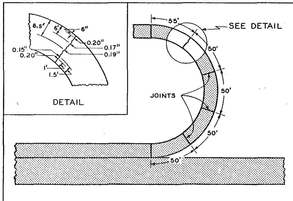
Figure 1. Location of crack and approximate joint spacing on interchange ramp.
