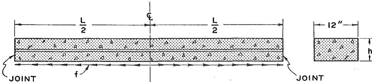
Figure 3. Longitudinal cross-section of a straight pavement subjected to subgrade friction.
