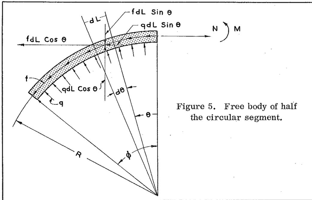
Figure 5. Free body of half the circular segment.
