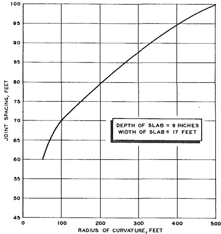
Figure 6. Joint spacing and curve radius variation.
