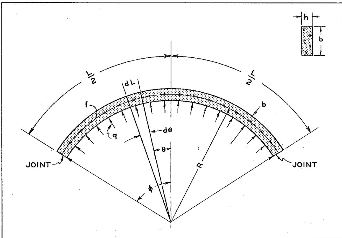
Figure 4. Circular pavement subjected to subgrade friction.
