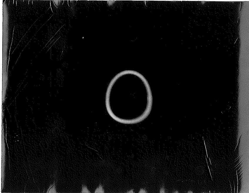
Figure 4. Lissajous figure obtained during test when beam is vibrating at its fundamental frequency.
