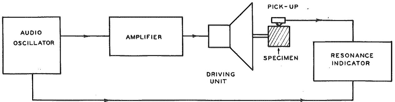
BLOCK DIAGRAM OF SONIC APPARATUS
