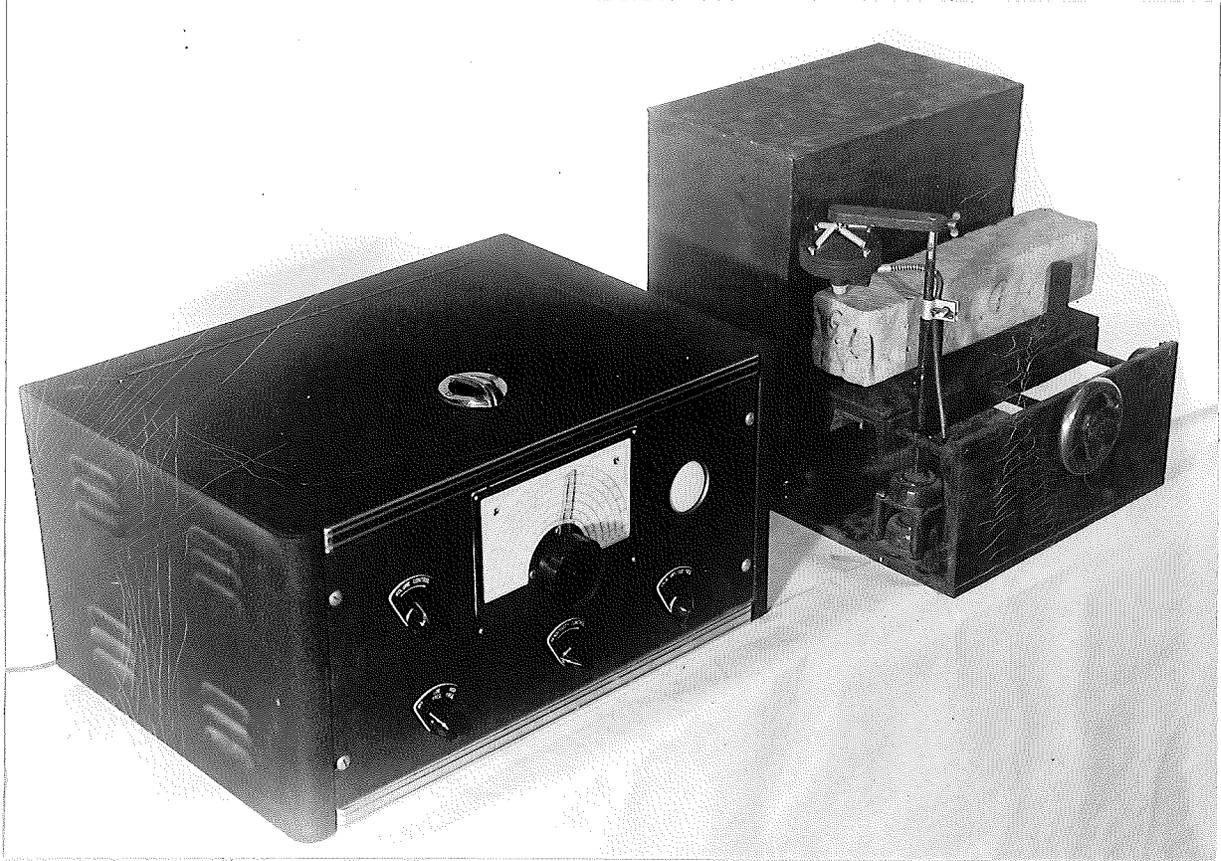
Figure 5. Sonic apparatus ready for test with beam mounted on nodal supports and crystal pick-up in position.
