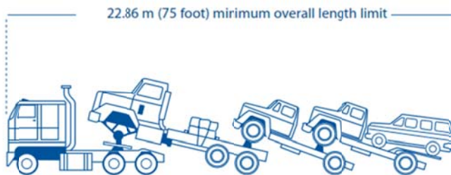
Figure 3. 5. Saddlemount with Fullmount Combination.
