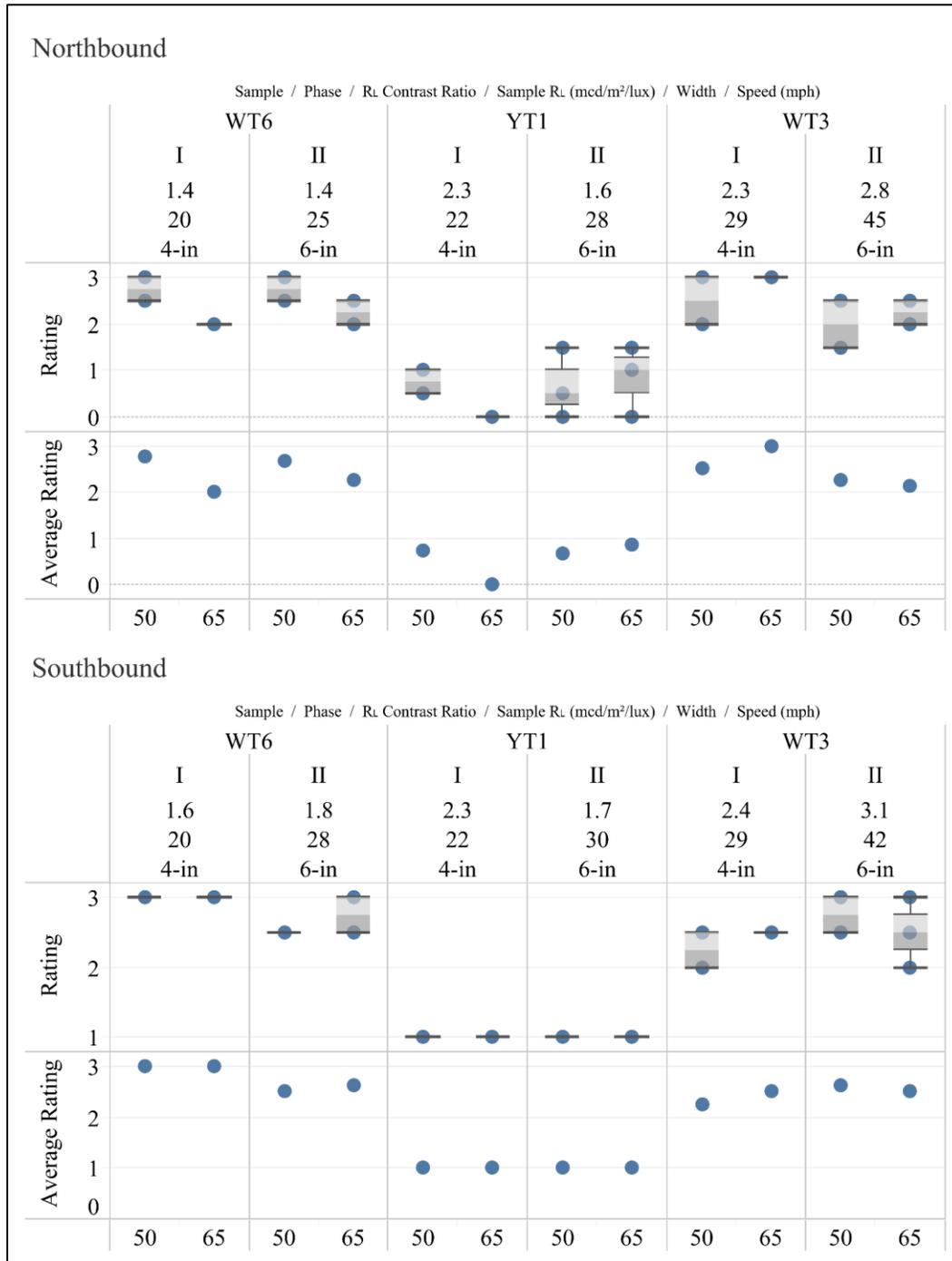
**Figure 26. Phase II 6-inch only Markings by Observation Speed, Dry, Nighttime Conditions**
