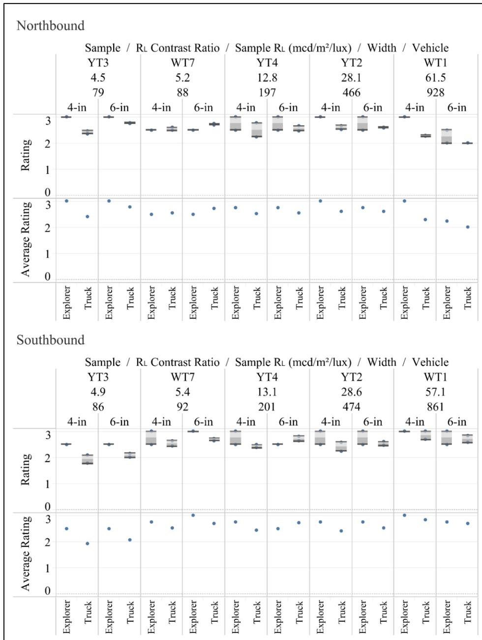
**Figure 38. Dry, Nighttime Observations, 4- and 6-inch Markings by Explorer and F-150**
