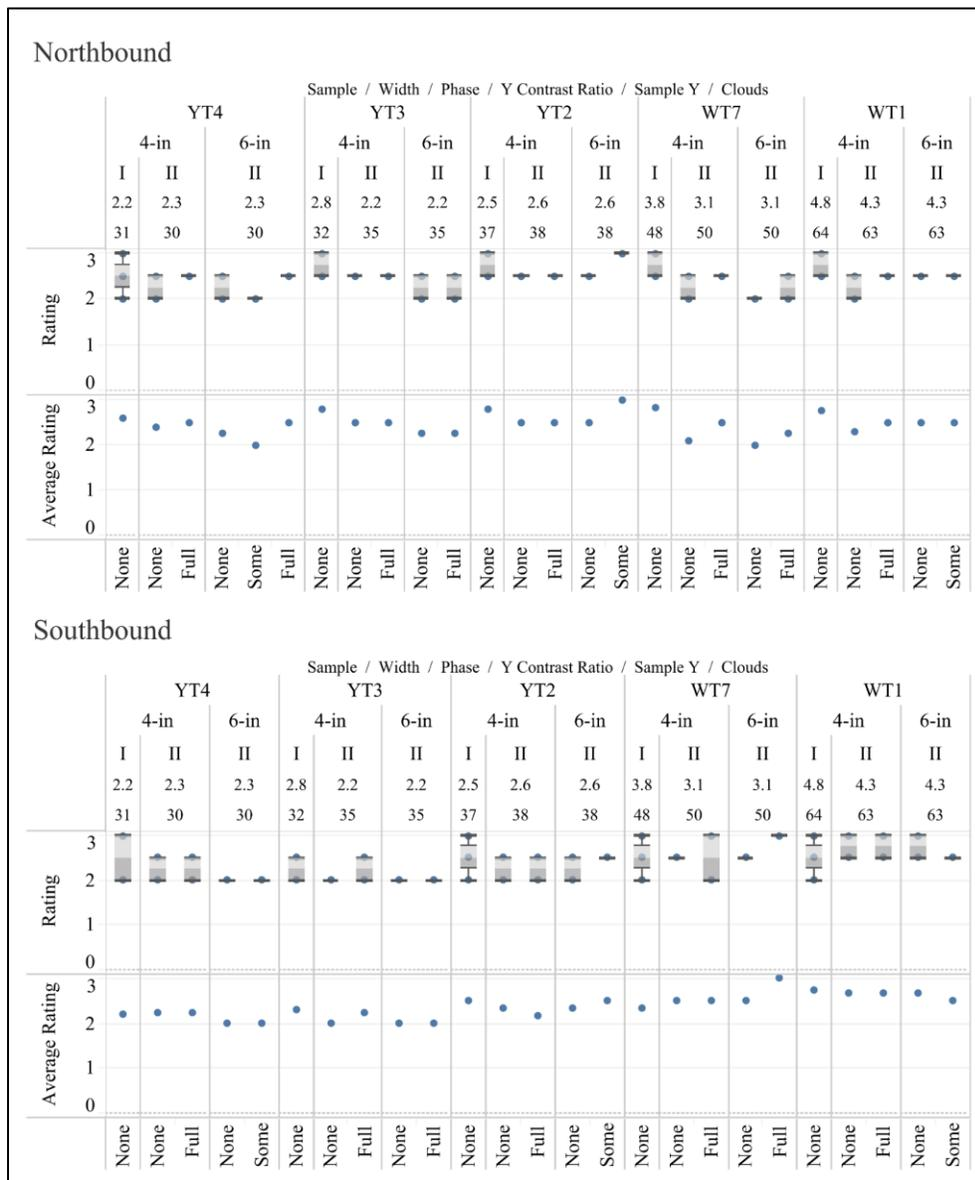
**Figure 27. Phase II 4- and 6-inch Markings Dry, Daytime, Cloud Cover Assessment**
