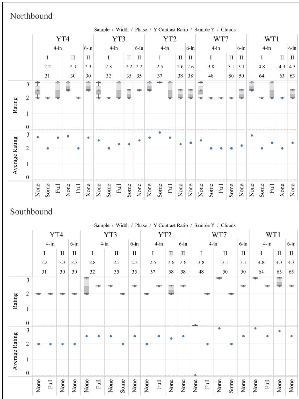
**Figure 29. Phase II 4- and 6-inch Markings Wet, Daytime, Cloud Cover Assessment**
