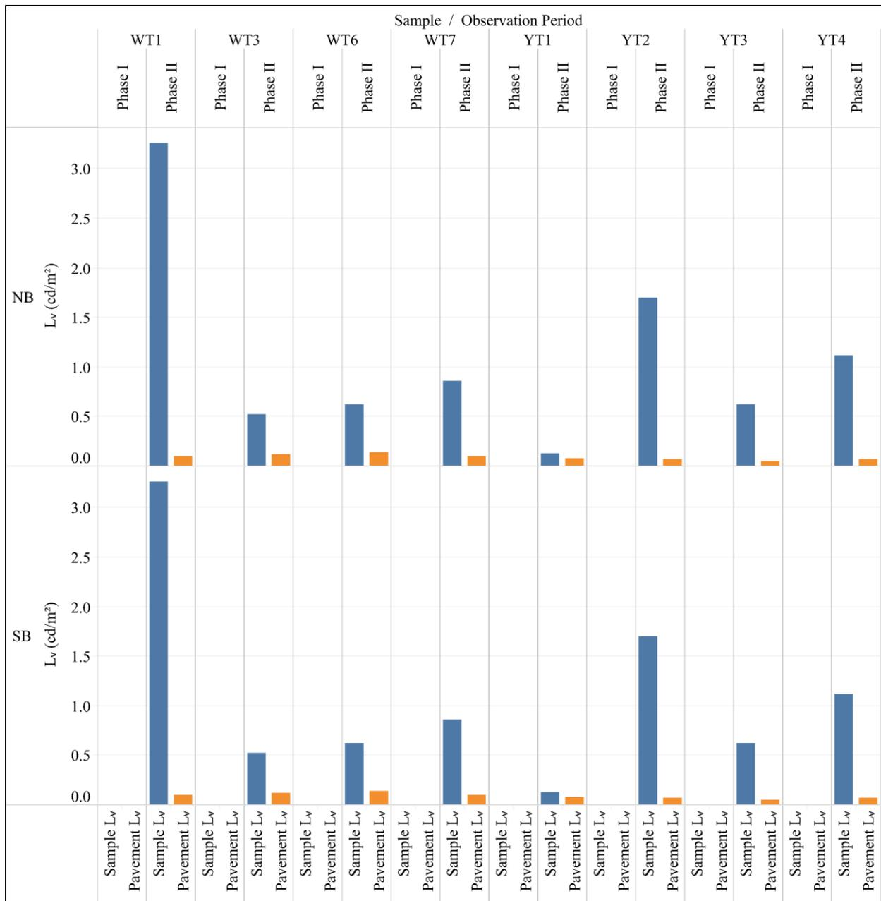
**Figure 18. Phase II CCD Luminance During Wet, Nighttime Conditions**
