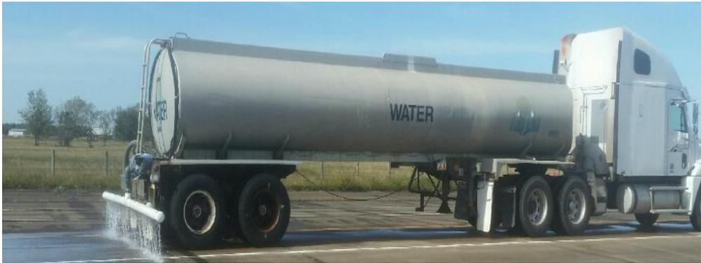
**Figure 2. Water Distribution System on Semi-Trailer**
