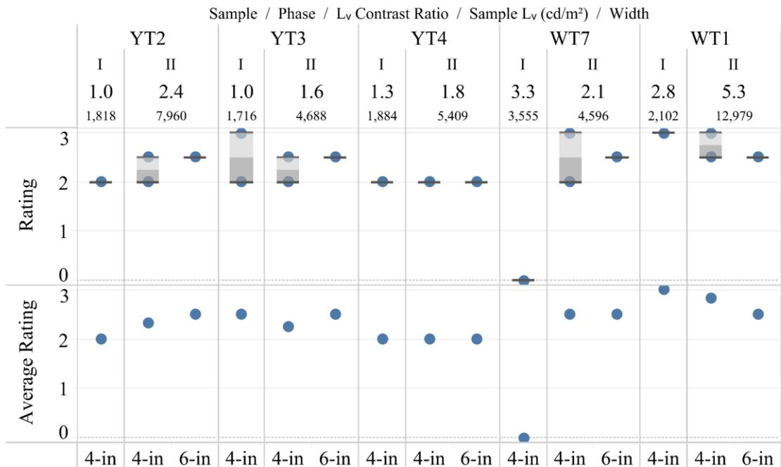
**4- and 6-inch Phase II Sample vs. Luminance Contrast Ratio, Wet, Daytime Conditions**
