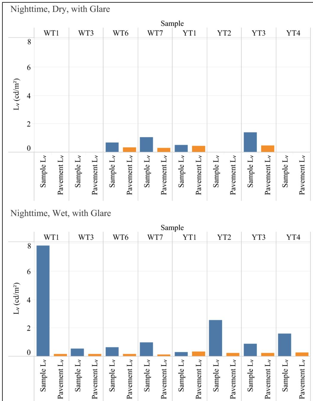
**Figure 21. CCD Luminance During Dry and Wet Nighttime Conditions with Glare**
