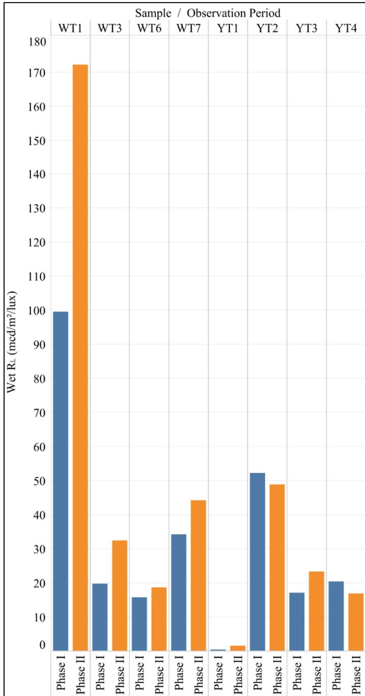
**Figure 14. Marking Recovery Retroreflectivity**
