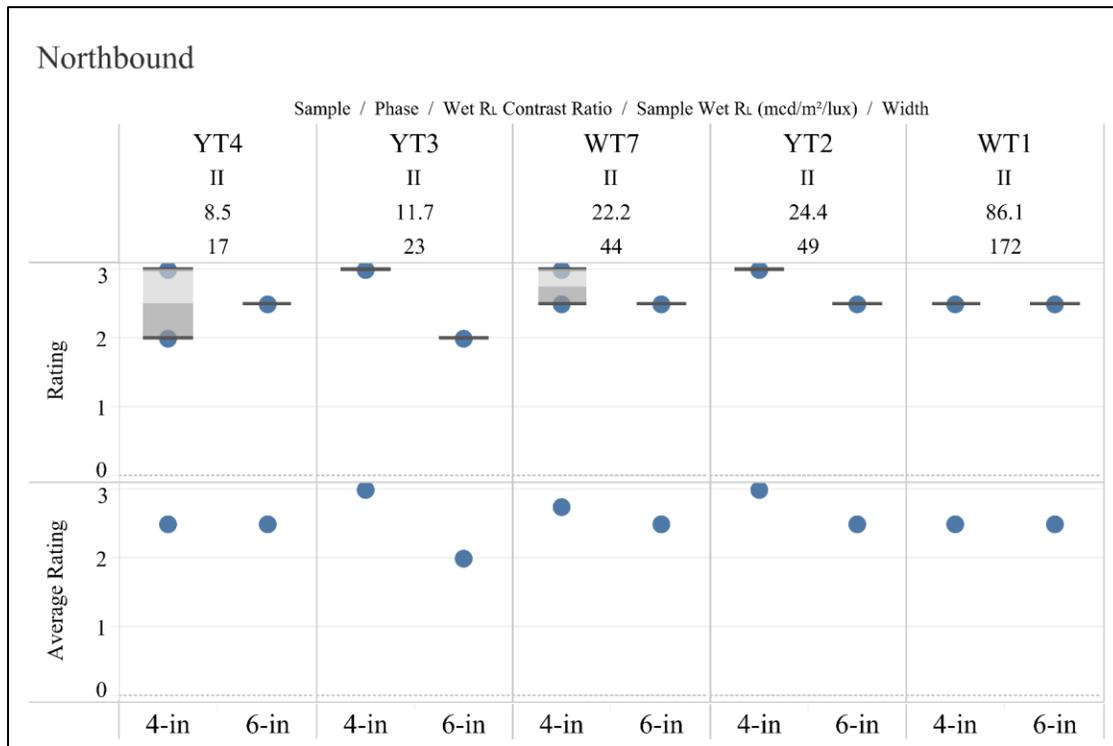
**Figure 43. Wet, Nighttime, Glare Observations, 4- and 6-inch Phase II**
