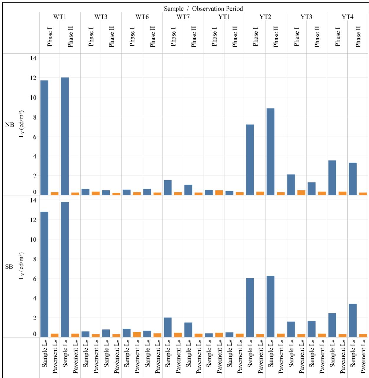
**Figure 16. CCD Luminance Measurements During Dry, Nighttime Conditions**
