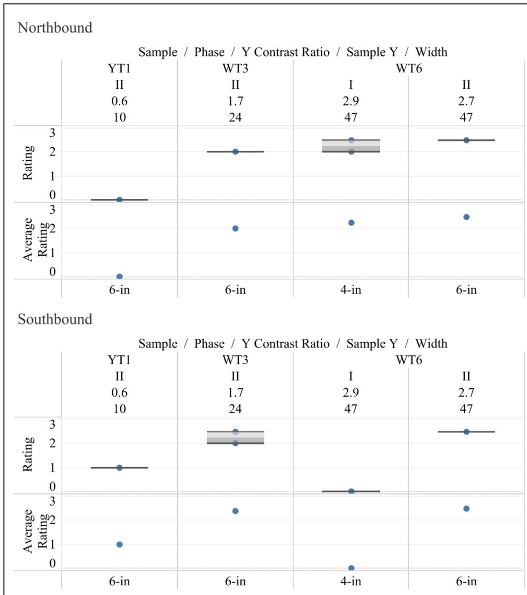
**Figure 36. Wet, Daytime Observations, 4-inch Phase I vs. 6-inch Phase II, Explorer Only**
