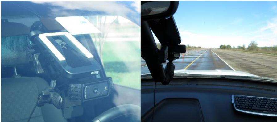
**Figure 4. Mobileye Camera from Exterior and Interior of Ford Explorer**
