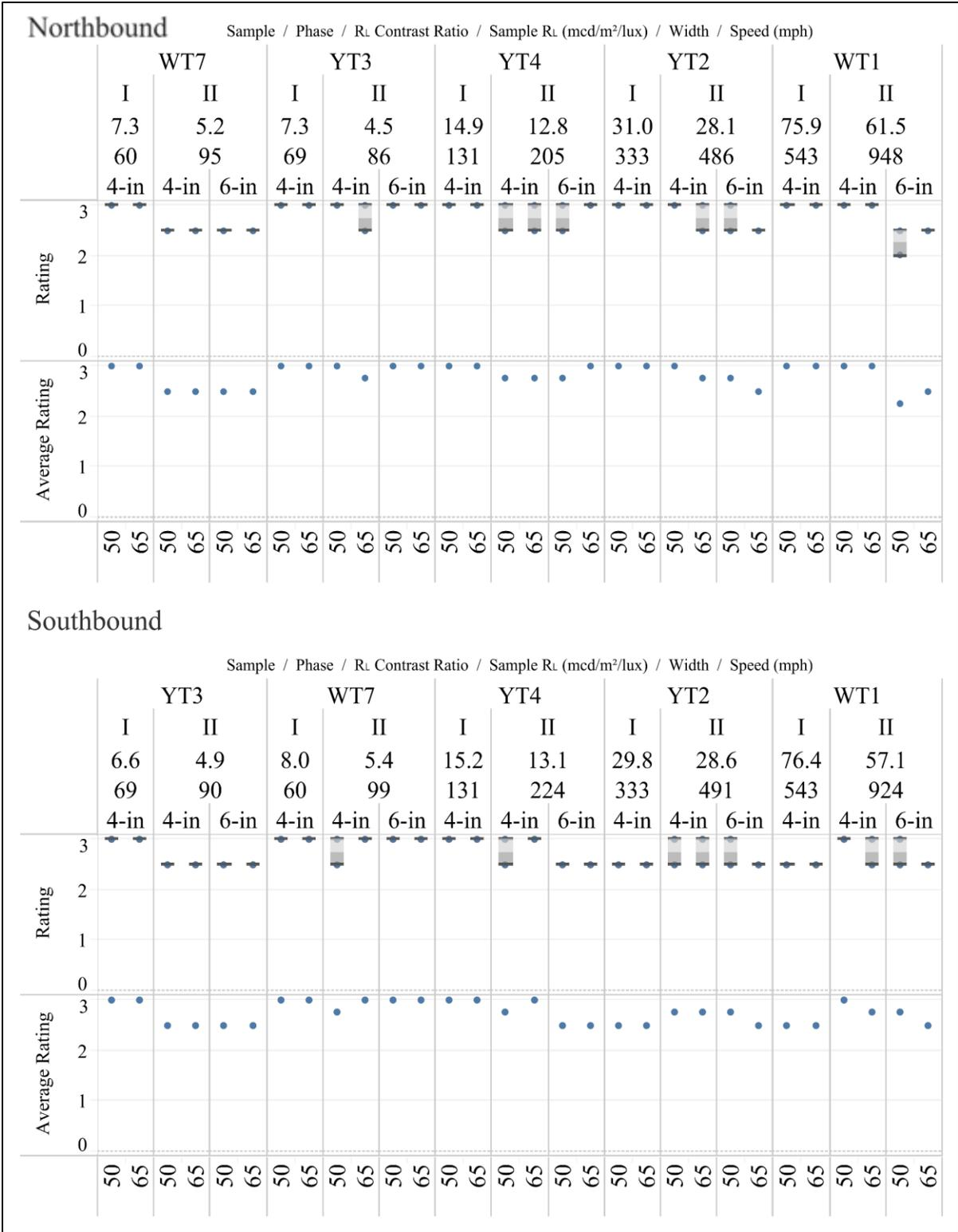
Figure 25. Phase II 4- and 6-inch Markings by Observation Speed, Dry, Nighttime Conditions
