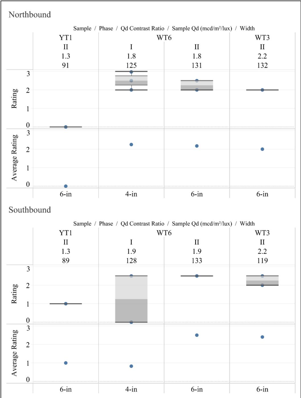
**6-inch Phase II Sample vs. Qd Contrast Ratio, Wet, Daytime Conditions**
