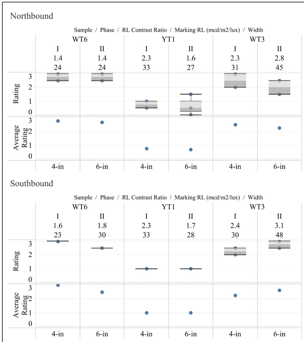
**Figure 39. Dry, Nighttime Observations, 4-inch Phase I vs. 6-inch Phase II, Explorer Only**
