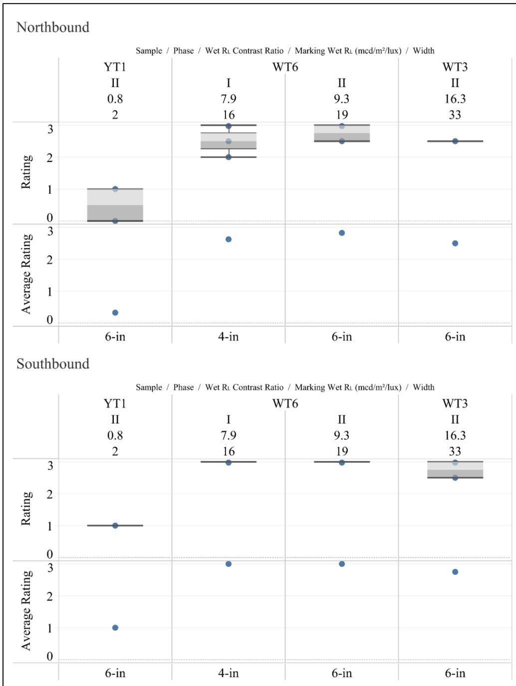
**Figure 41. Wet, Nighttime Observations, 4-inch Phase I vs. 6-inch Phase II**
