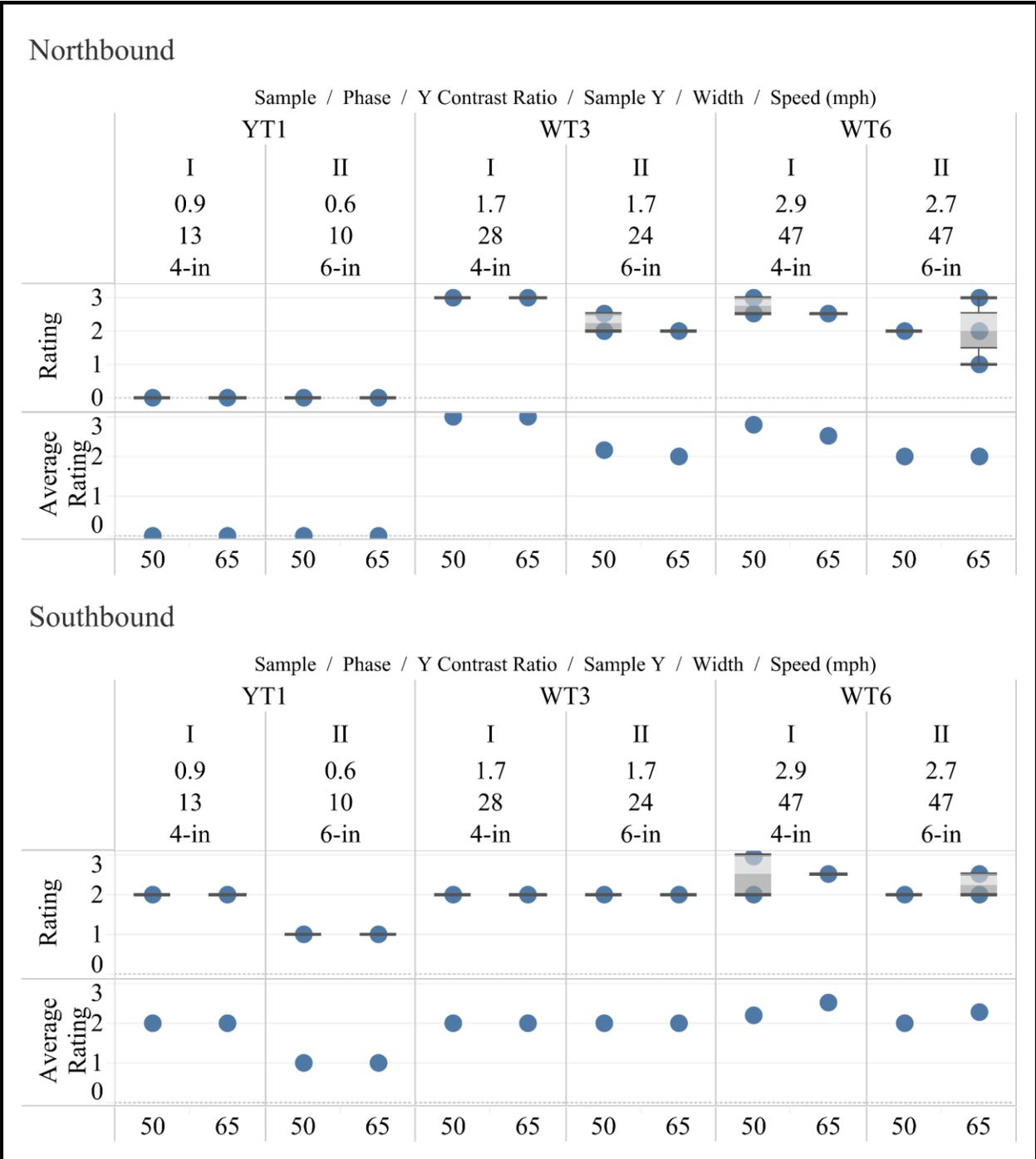
Figure 24. Phase II 6-inch only Markings by Observation Speed, Dry, Daytime Conditions
