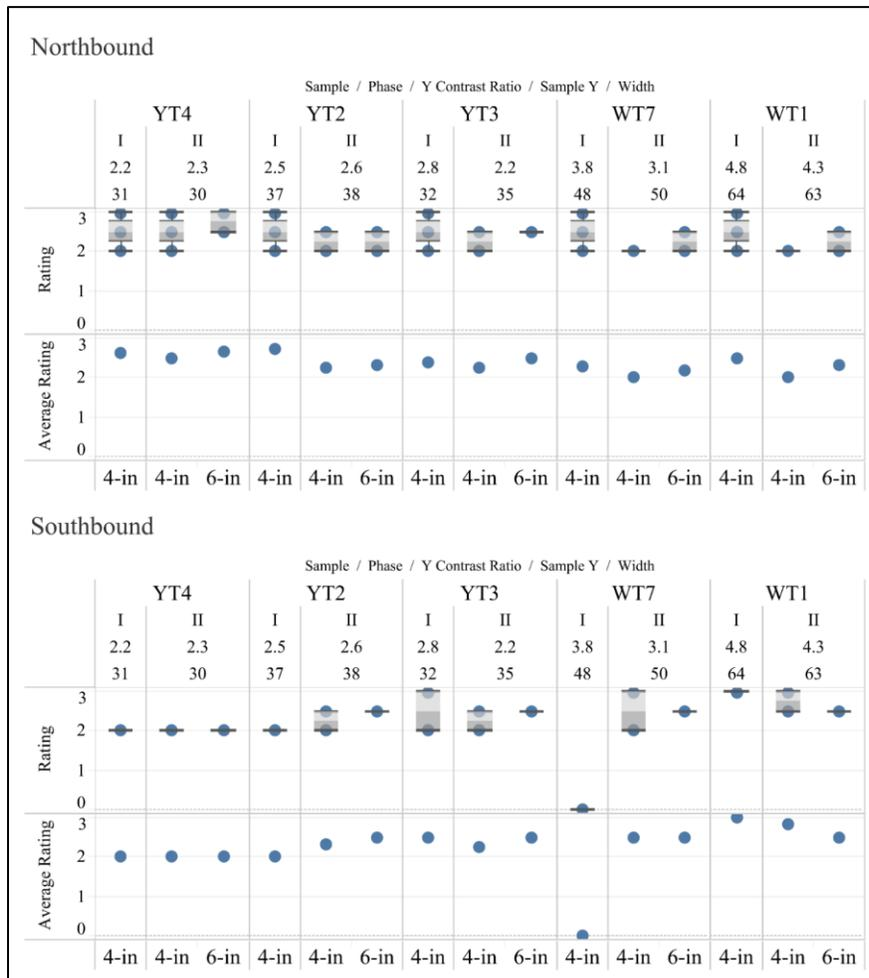
**Figure 34. Wet, Daytime Observations, 4-inch Phase I vs. 4- and 6-inch Phase II**
