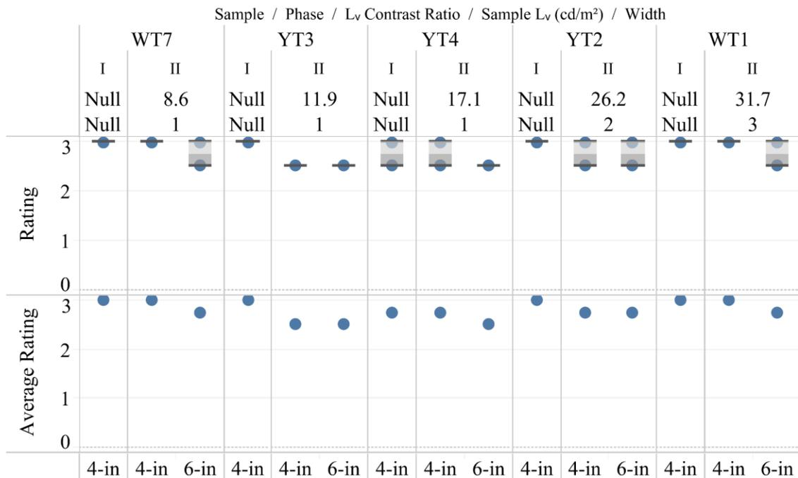
and 6-inch Phase II Sample vs. Luminance Contrast Ratio, Wet, Nighttime Conditions
