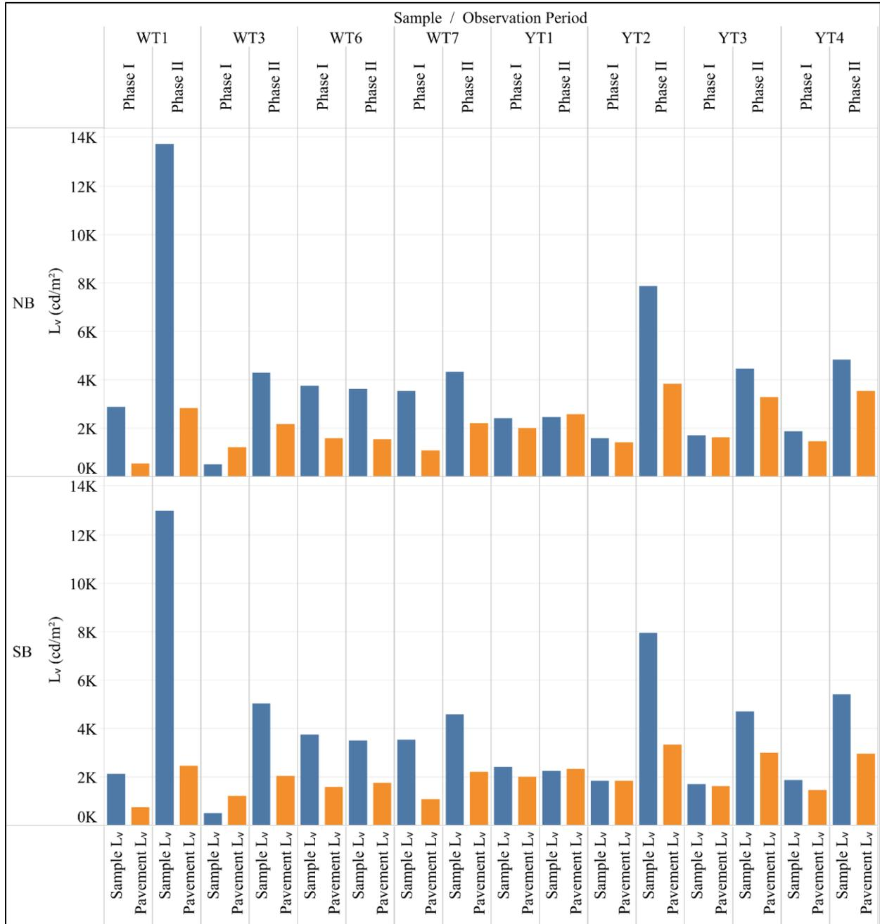
**Figure 12. CCD Luminance Measurements During Wet, Daytime Conditions**
