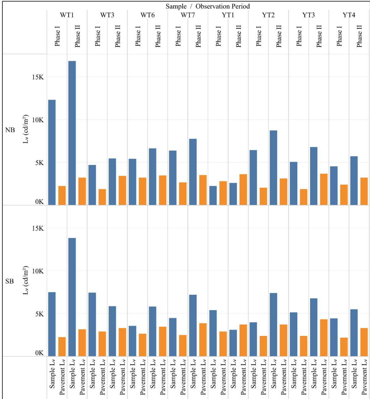
**Figure 10. CCD Luminance During Dry, Daytime Conditions**
