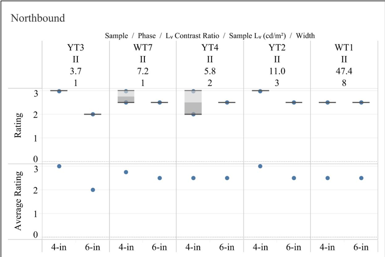
**4- and 6-inch Phase II Sample vs. Luminance Contrast Ratio, Wet, Nighttime, Glare Conditions**
