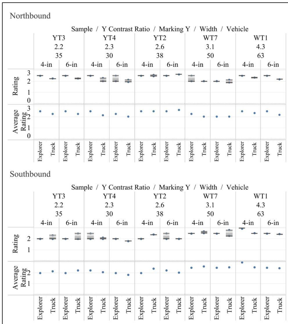
**Figure 32. Dry, Daytime Observations of 4- and 6-inch Markings by Explorer and F-150**
