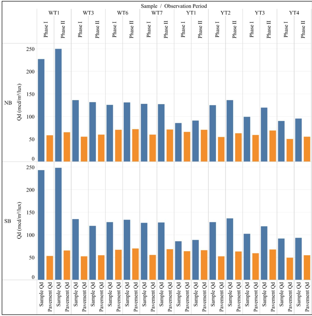
**Figure 9. Retroreflectometer Qd Measurements**
