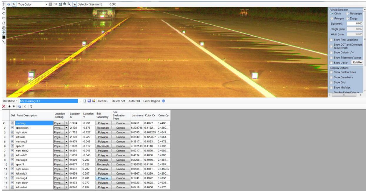
**Figure 17. CCD Camera Interface During Wet, Nighttime Data Collection**
