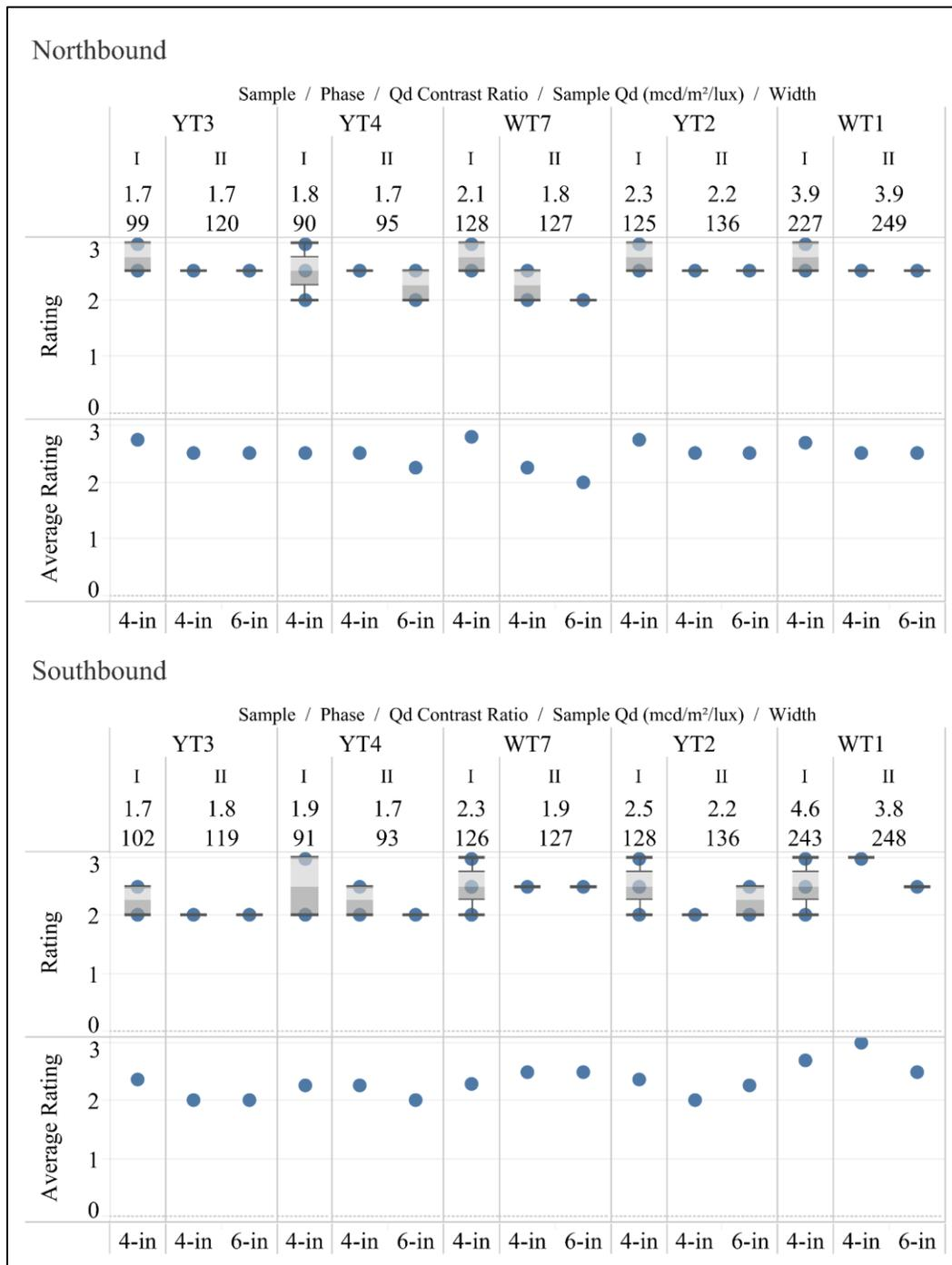
4- and 6-inch Phase II Sample vs. Qd Contrast Ratio, Dry, Daytime Conditions
