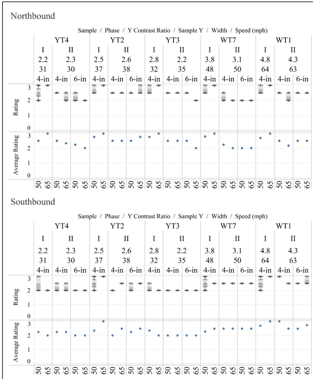
**Figure 23. Phase II 4- and 6-inch Markings by Observation Speed, Dry, Daytime Conditions**
