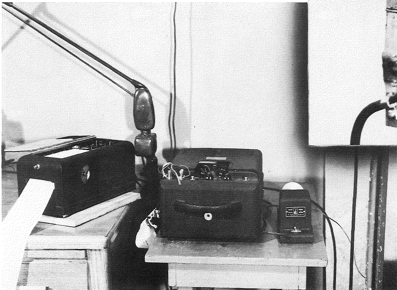
FIGURE 2. TESTING EQUIPMENT USED FOR MEASURING THE FORCE EXERTED BY THE TIE WIRE.
