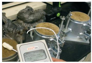
This project showed that thermal conductivity, which is easy to measure, could be used to accurately model the impact of a soil's properties on its freezing behavior.
