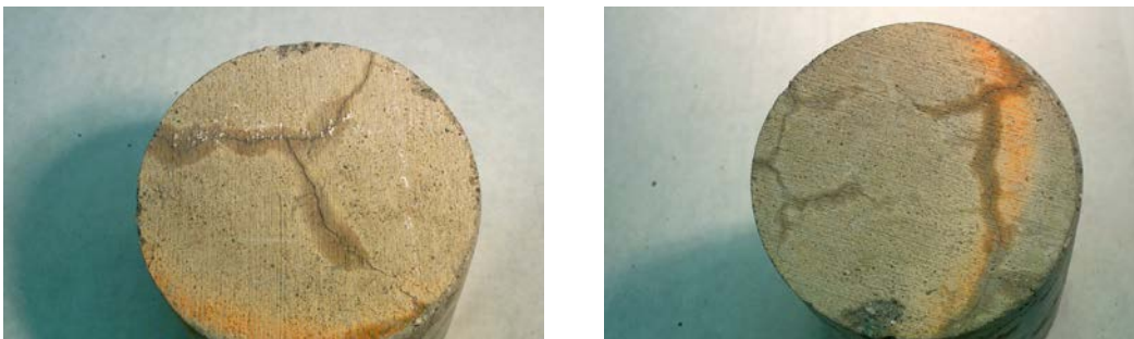
Figure A-35. Map cracking at the top surface of cores F1 (left) and F2 (right).
