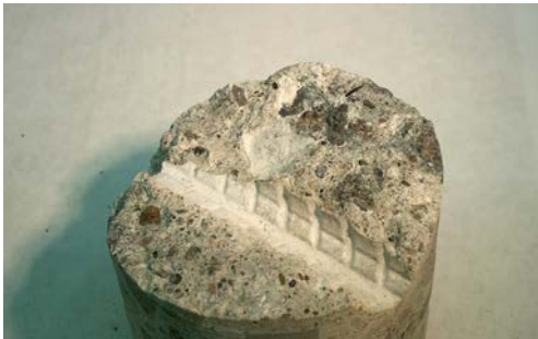
Figure A-34. Imprint of rebar in core F2.
