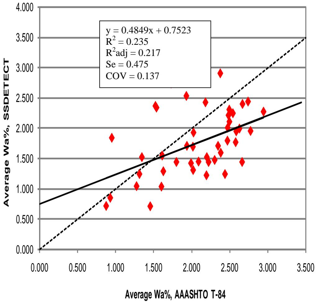
**Figure 4 AAASHTO T-84 against SSDETECT Water Absorption (Wa %)**
