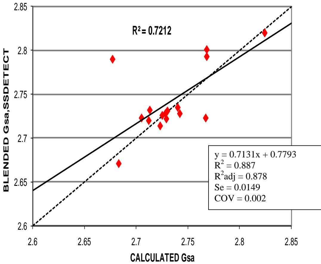
**Figure 7 Blended-Calculated against SSDetect Gsa**
