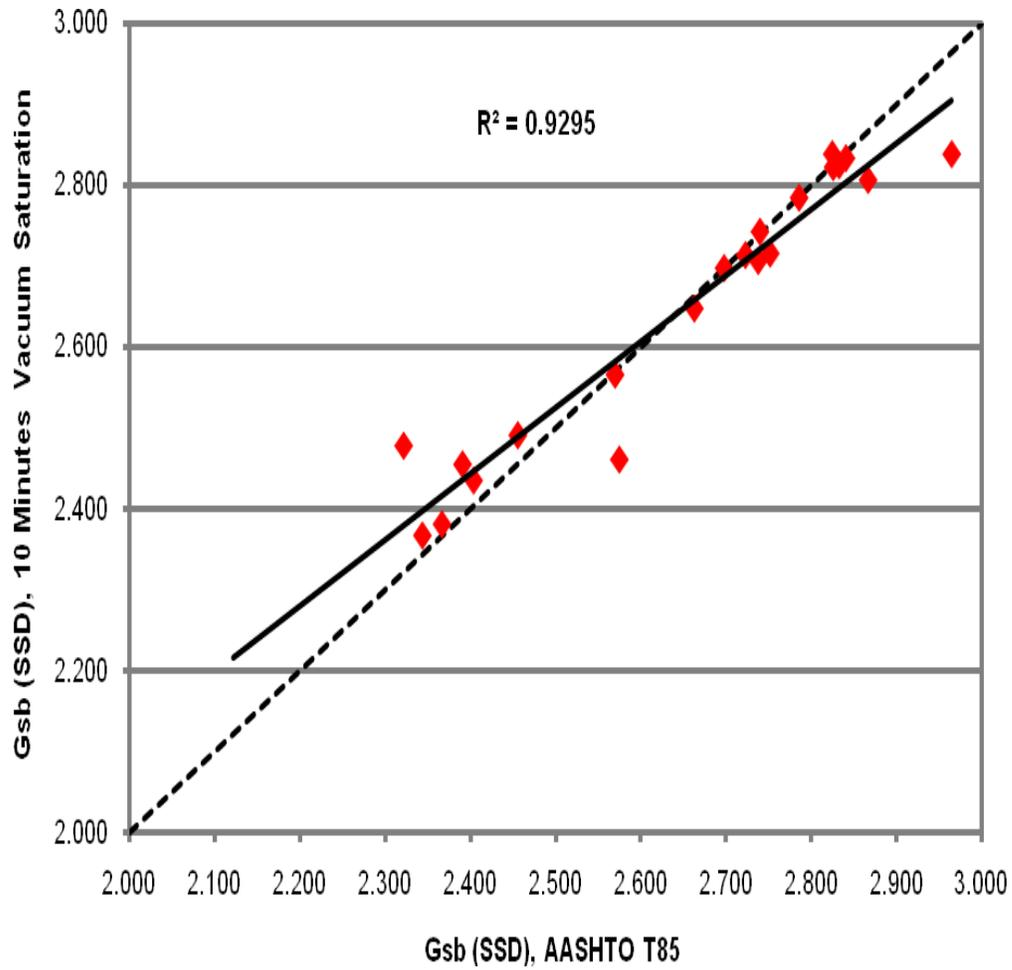
**Figure 12 AASHTO T-85 against 10 Minutes Vacuum Saturation Test for Gsb (SSD)**
