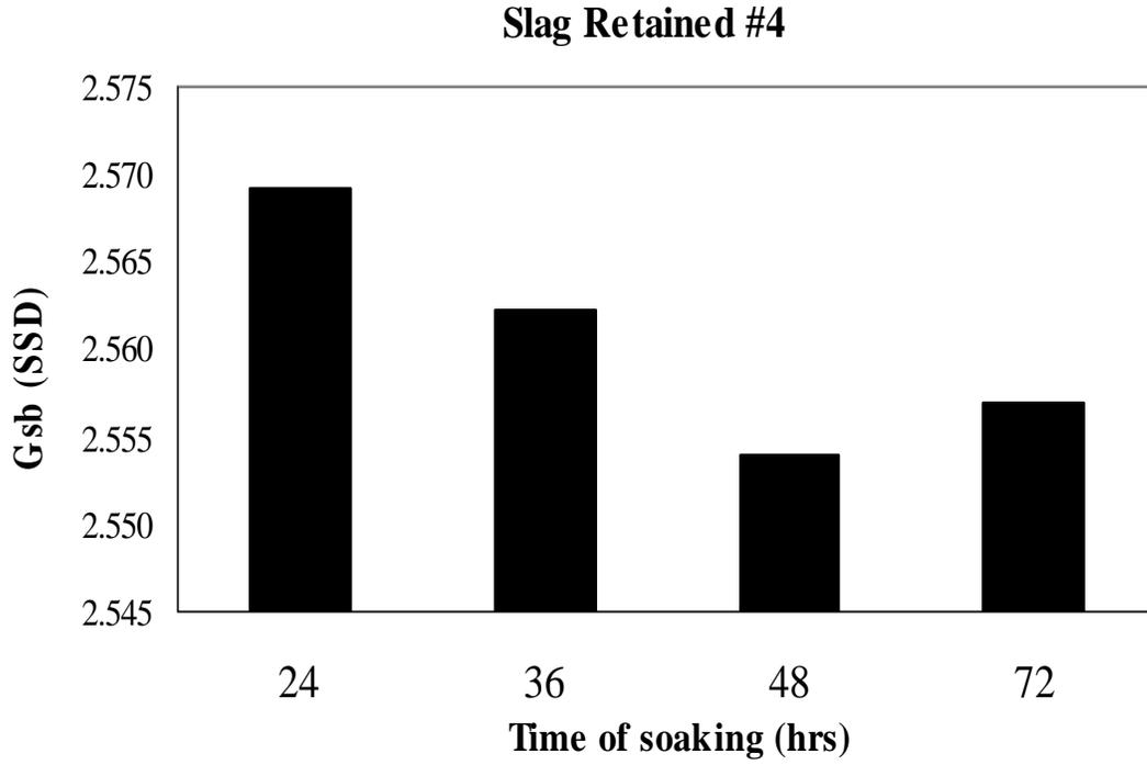
**Figure 26 Gsb (SSD) test results over 24, 36, 48 and 72 hours of soaking periods**
