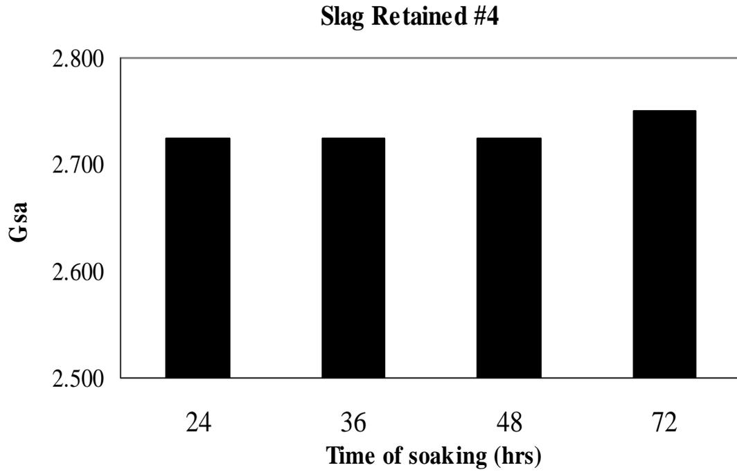
**Figure 27 Gsa test results over 24, 36, 48 and 72 hours of soaking periods**
