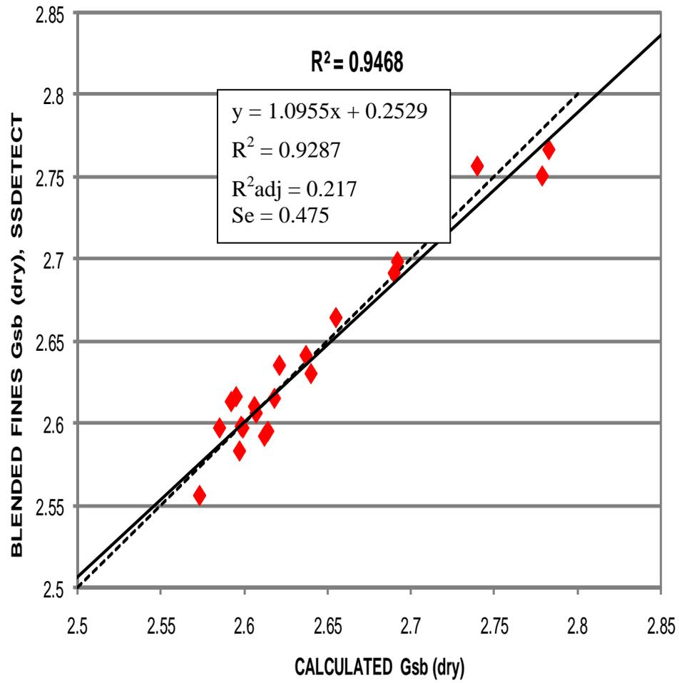
**Figure 5 Blended-Calculated against SSDetect Gsb (dry)**
