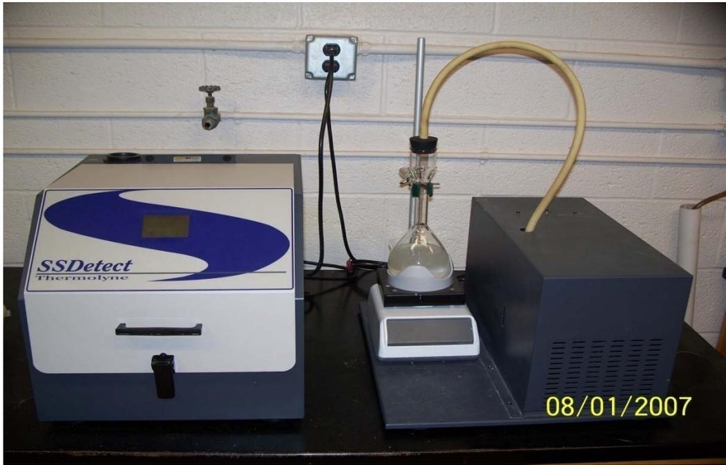
**Figure 5. The SSDetect with AVU unit**
