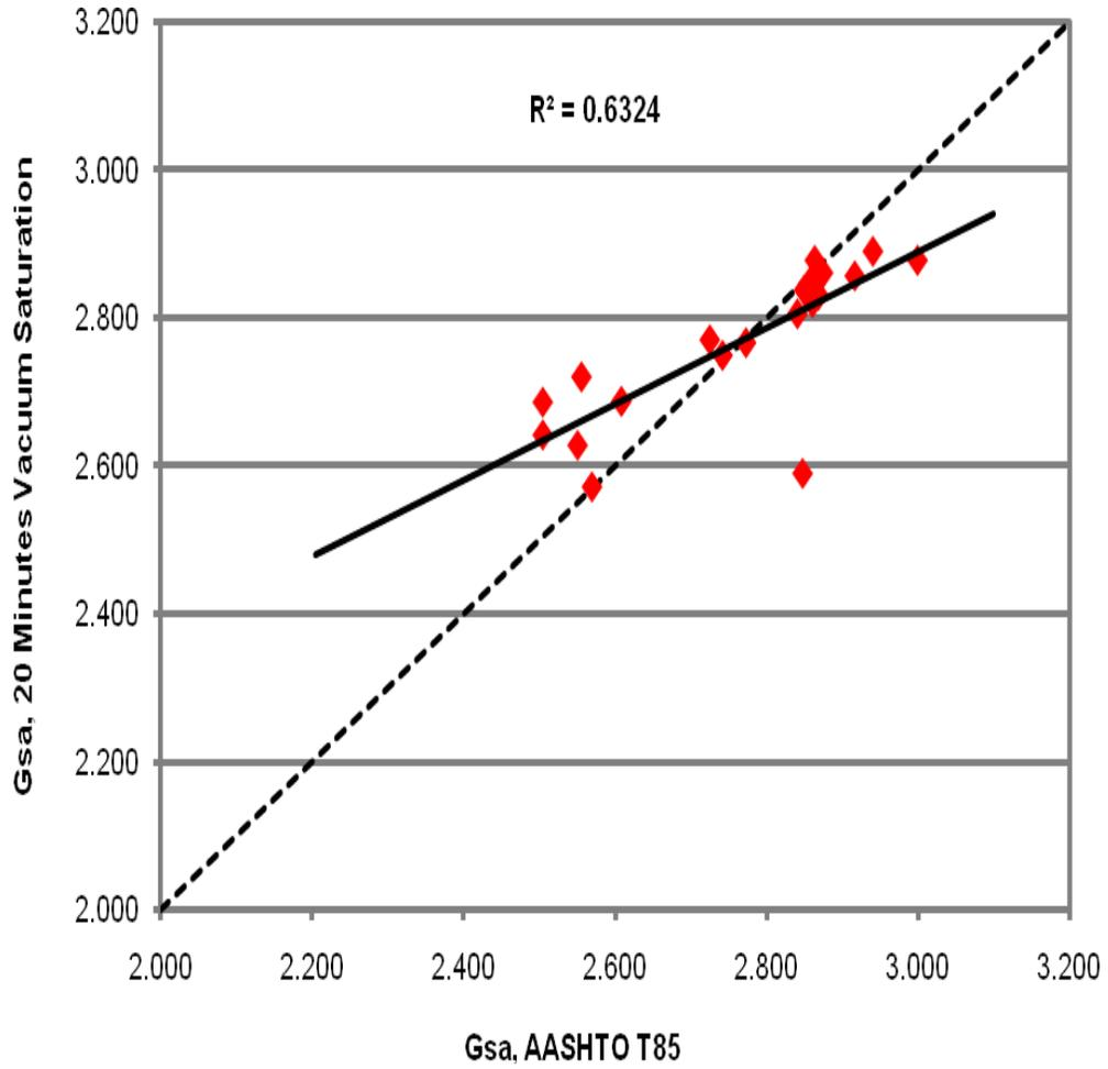
**Figure 16 AASHTO T-85 against 20 Minutes Vacuum Saturation Test for Gsa**
