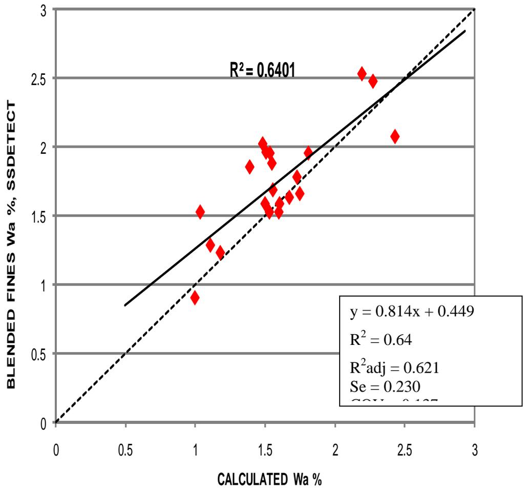
**Figure 8 Blended-Calculated against SSDetect Wa%**
