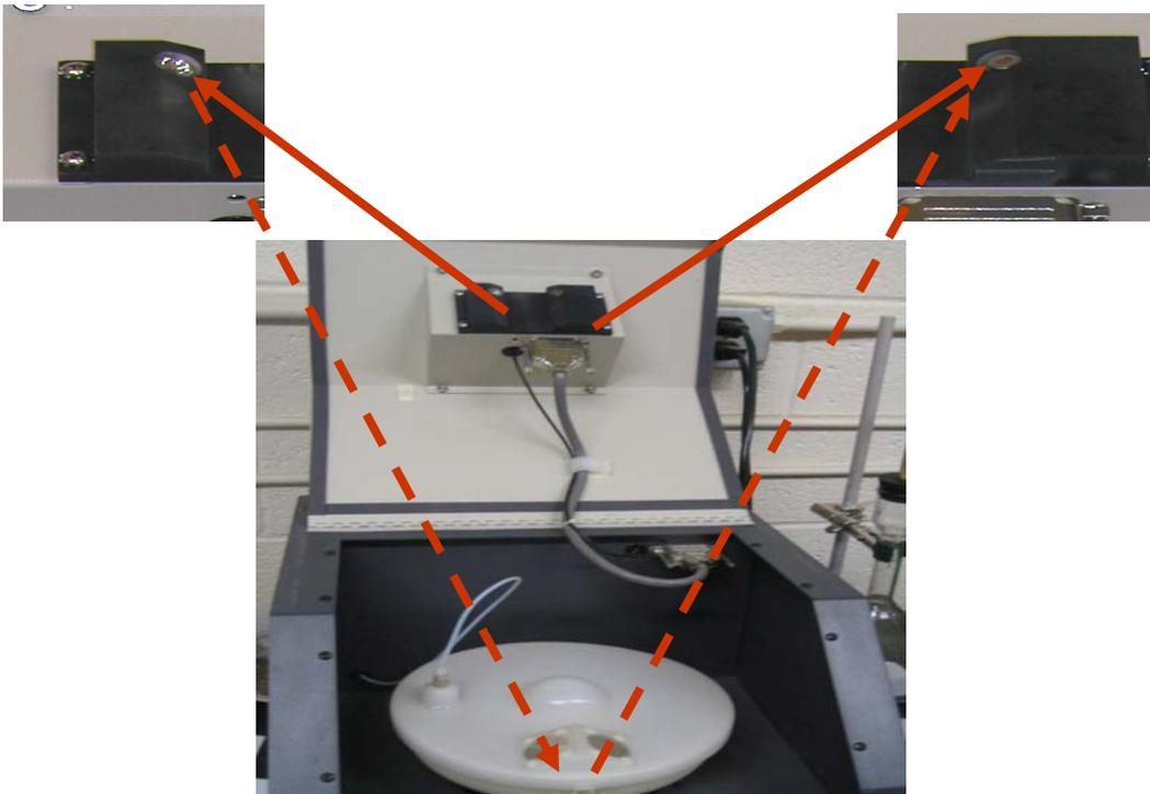
**Figure 6 Internal components of the SSDetect**
