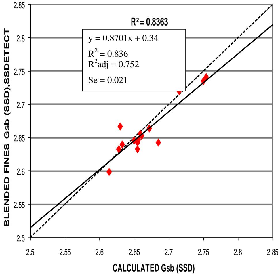
**Figure 6 Blended-Calculated against SSDetect Gsb (SSD)**
