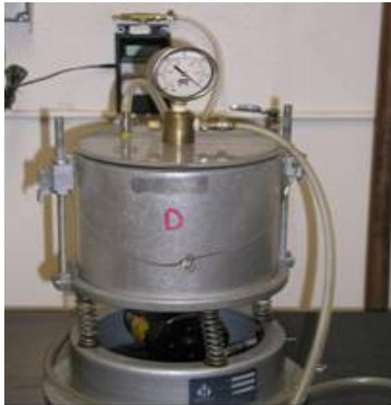
**Figure 9. The Vacuum saturation apparatus used to expel the air in the coarse aggregate mass and force water into the pores of the aggregates**
