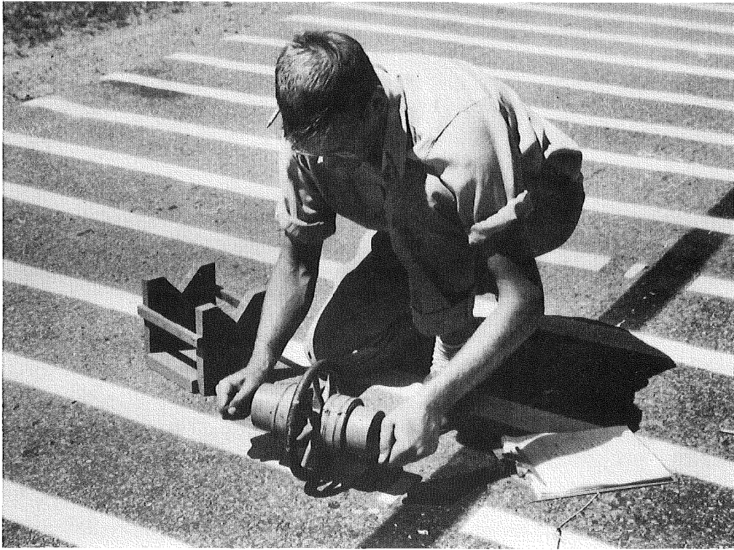
Figure 9. Drying time tests with standard ASTM wheel.
