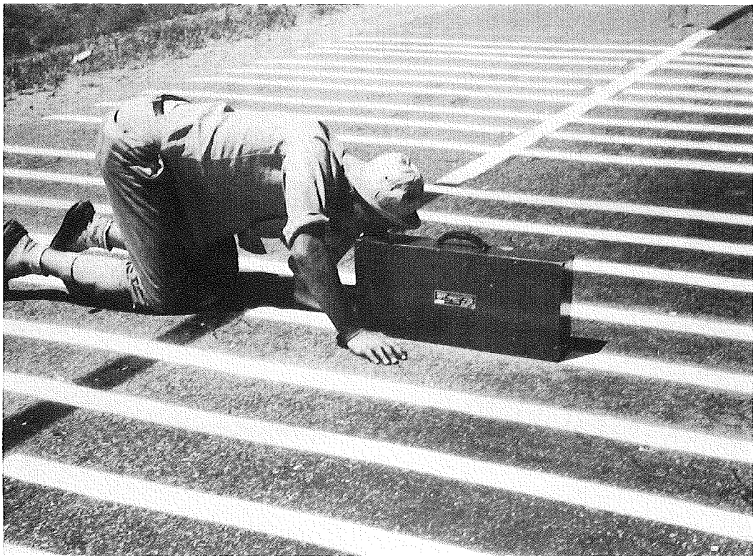
Figure 10. Taking night visibility readings on test stripes.
