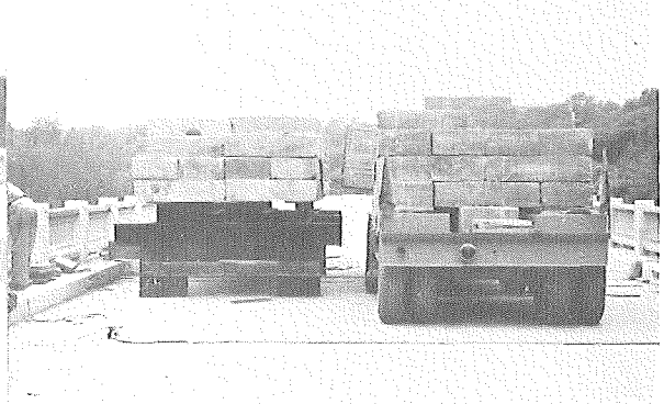
FIGURE 10. METHOD OF OBTAINING TWO-TRUCK LOAD CONDITIONS
