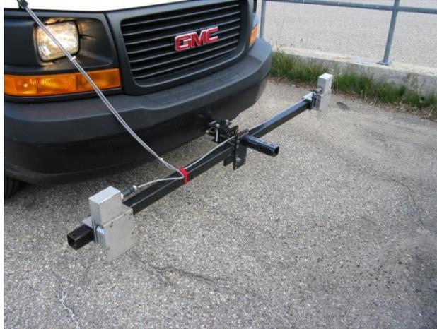
**Figure 16 – MDOT Profilometry Van - Front View**
