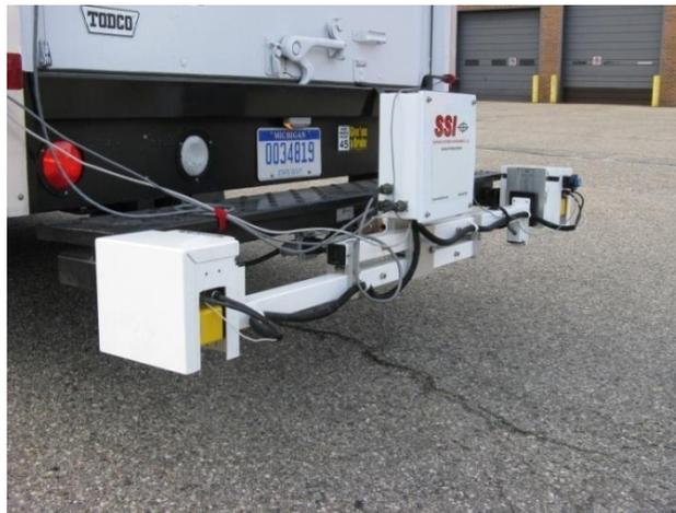
**Figure 17 – MDOT Profilometry Van - Rear View**
