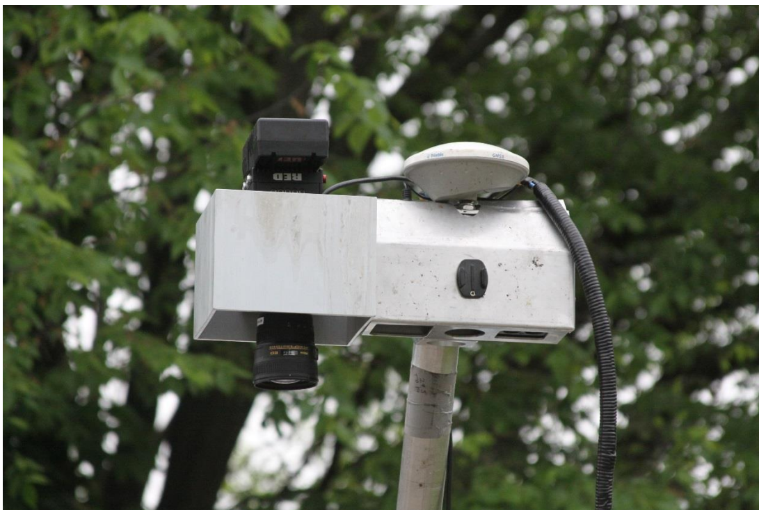
Figure 4-20: BridgeGuard Thermal Camera and RED Epic Mounted on Vehicle attached Boom.
