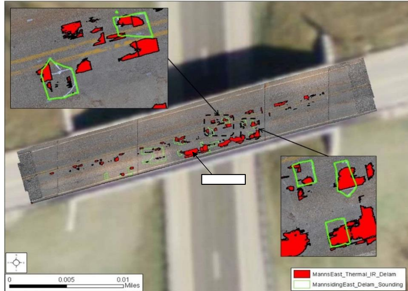
Figure 2-9: Combined Results of Thermal IR Imagery Chain Drag Inspection.
