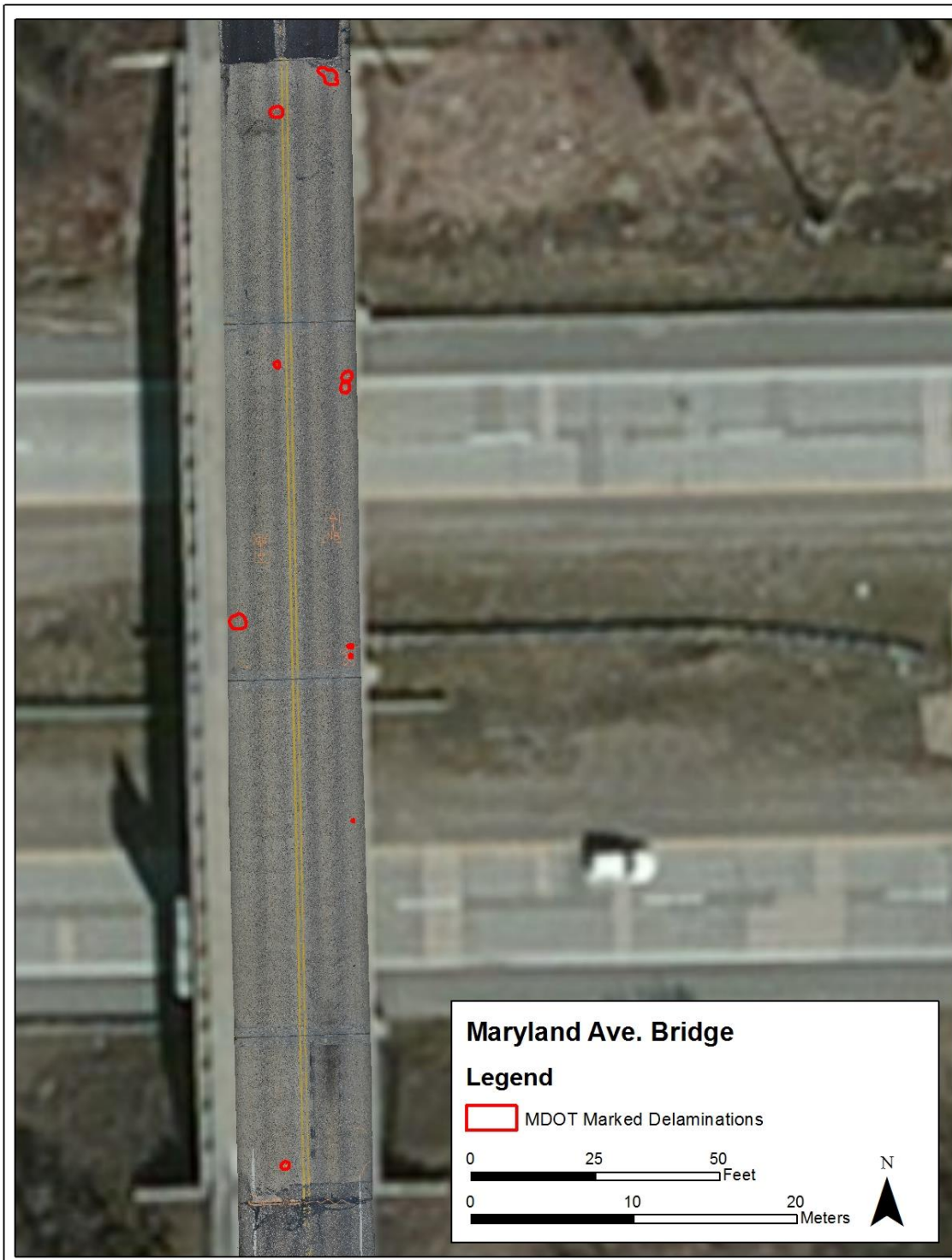
Figure 4-14: Georeferenced Sketch of the Results of the Deck Sounding of Maryland Ave. Showing the Locations of Delaminations.
