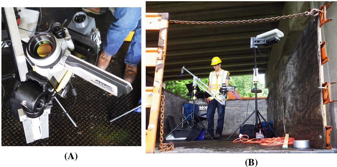
Figure 6-17: (A) FLIR SC640 and FLIR Tau 2 Thermal Infrared Cameras (B) Tripod Mounted Solaira Infrared Heater and Thermal Infrared Cameras.
