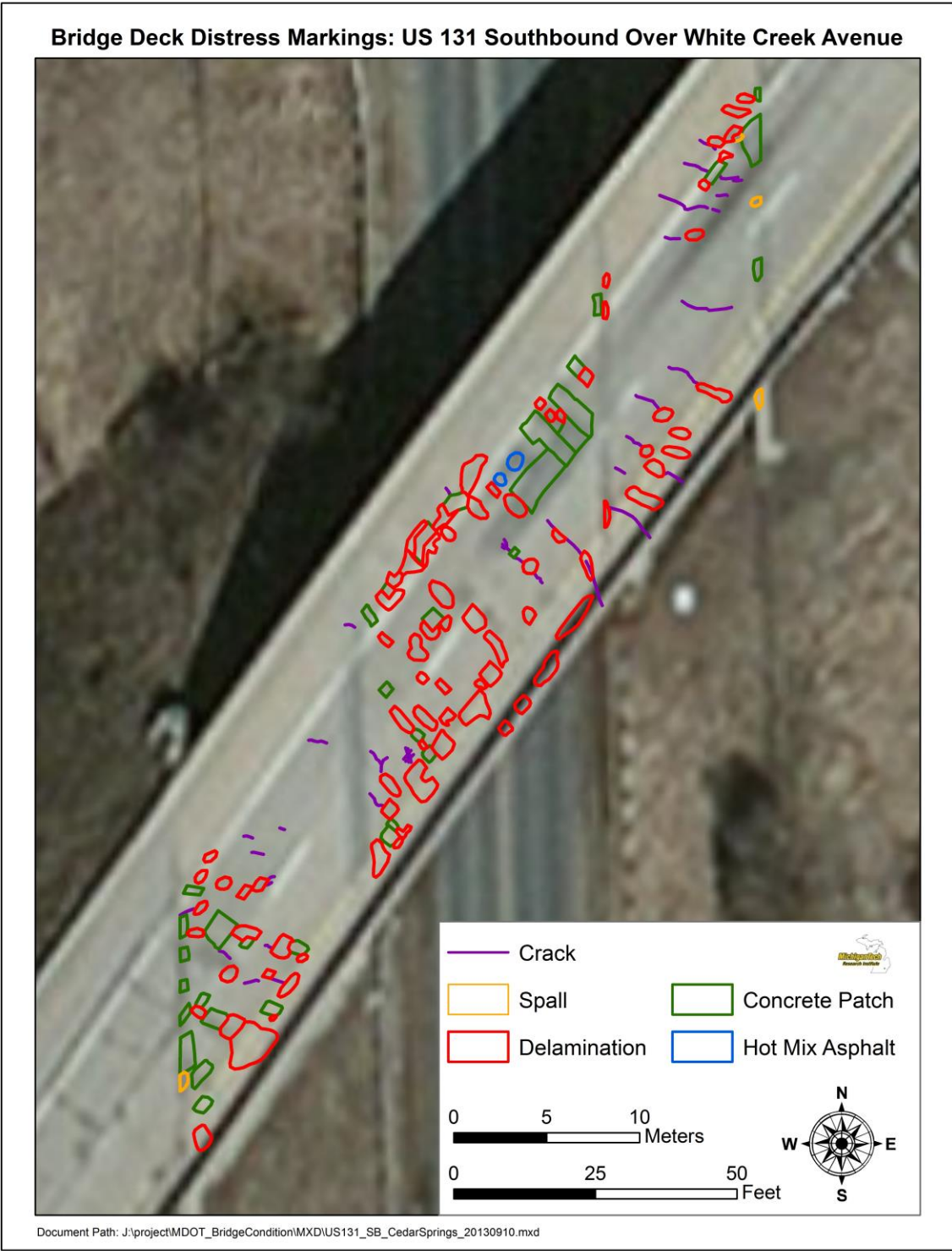
Figure 4-11: Georeferenced Sketch of the Results of the Deck Sounding of the South Bound Bridge of US-131 Showing the Locations of Delaminations, Cracking and Spalls.
