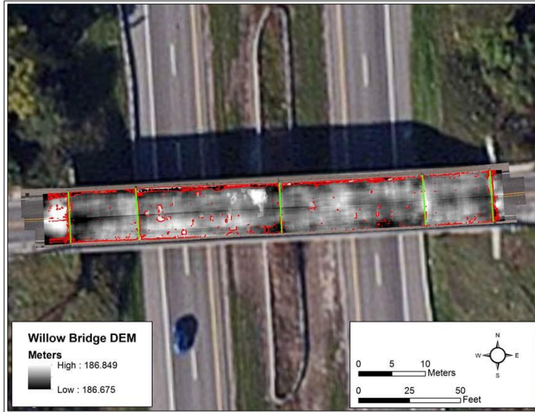
Figure 2-10: Willow Road Bridge Digital Elevation Model (DEM) and Spall Map Layer on ArcGIS.
