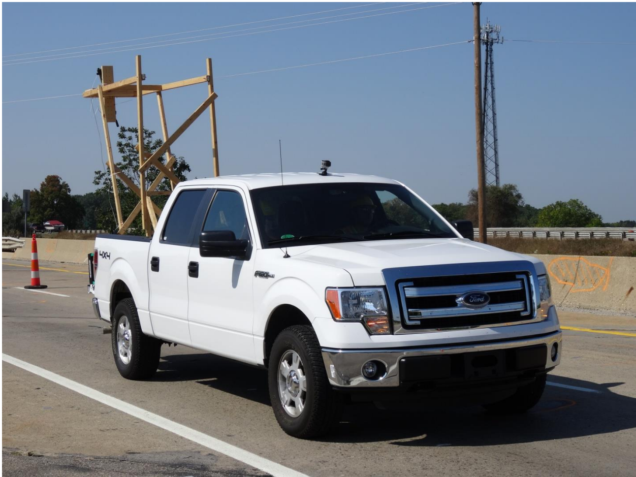
Figure 4-23: The Collection Setup for US-131 with a Single GoPro Mounted on the Roof of the Collection Vehicle.
