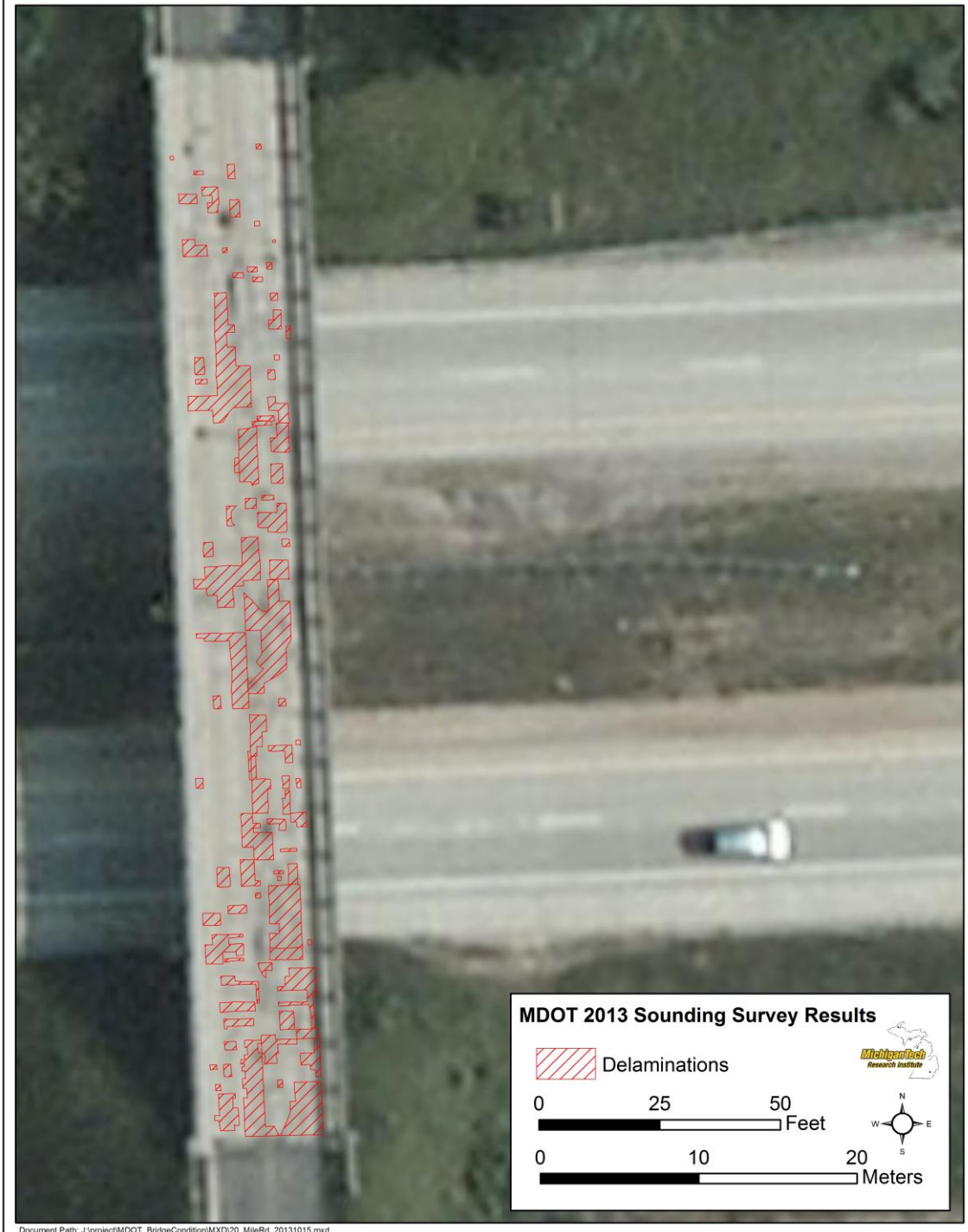
Figure 4-3: Georeferenced Sketch of the Results of the Deck Sounding Showing the Locations of Delaminations. The Total Area Delaminated is 1,276 ft 2 .
