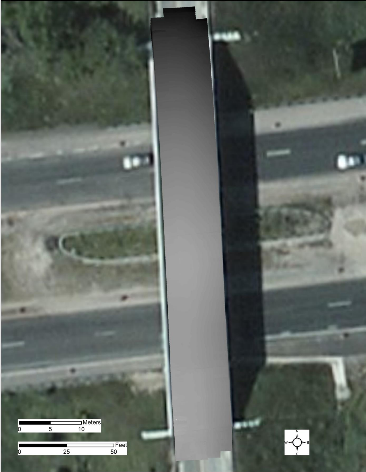
Figure 5-2: DEM of Freer Rd Generated from Imagery Collected from the RED Epic.
