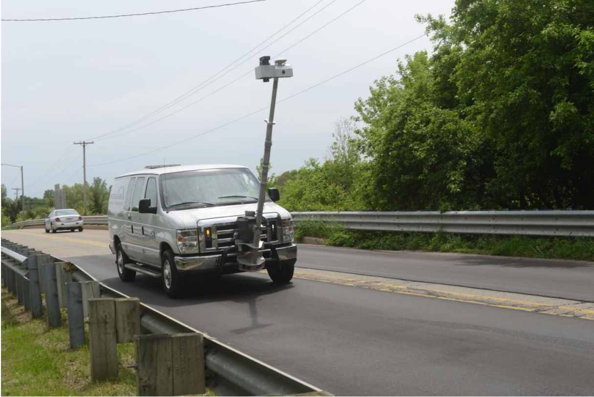
Figure 4-21: Combined 3DOBS and BridgeGuard Collecting Imagery over Maryland Ave. in Grand Rapids.
