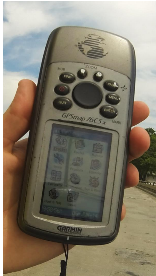
Figure 4-26: Detailed Image Showing the GPS Time in a Photo used to adjust the Time Difference between the Camera and the GPS Unit.
