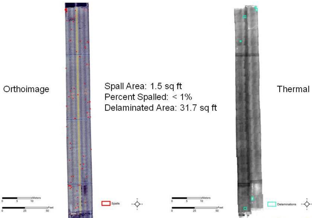
Figure 5-17: Comparison of the Results Generated from 3DOBS High Speed and the BridgeGuard Thermal Cameras as a Combined System over Maryland Ave.
