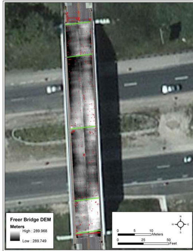
Figure 2-12: Freer Road Bridge Digital Elevation Model (DEM) and Spall Map Layer on ArcGIS.
