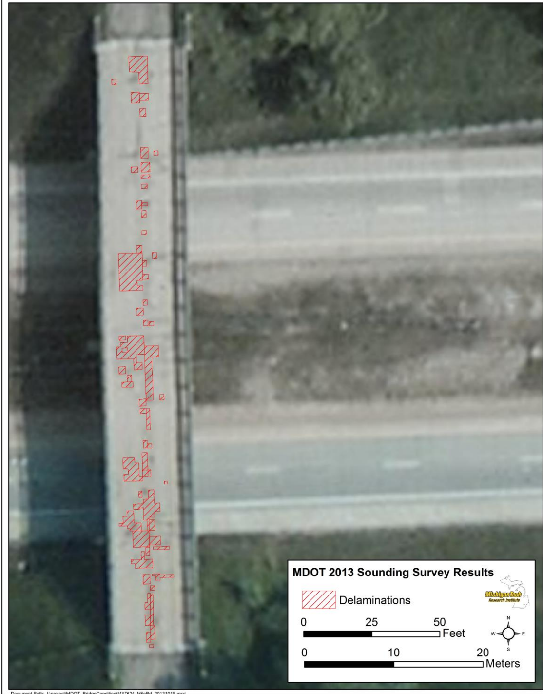
Figure 4-6: Georeferenced Sketch of the Results of the Deck Sounding of 24 Mile Rd Showing the Locations of Delaminations. The Total Area Delaminated is 762 ft 2
