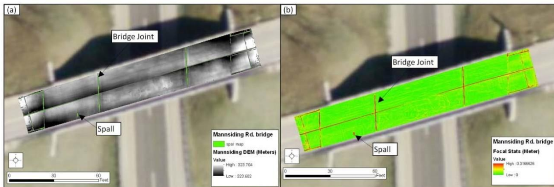
Figure 2-8: A) Mannsiding Road Bridge Digital Elevation Model (DEM) and Spall Map Layer on ArcGIS, B) Mannsiding Road Bridge Spall Map Generated with Spall Detection Algorithm.
