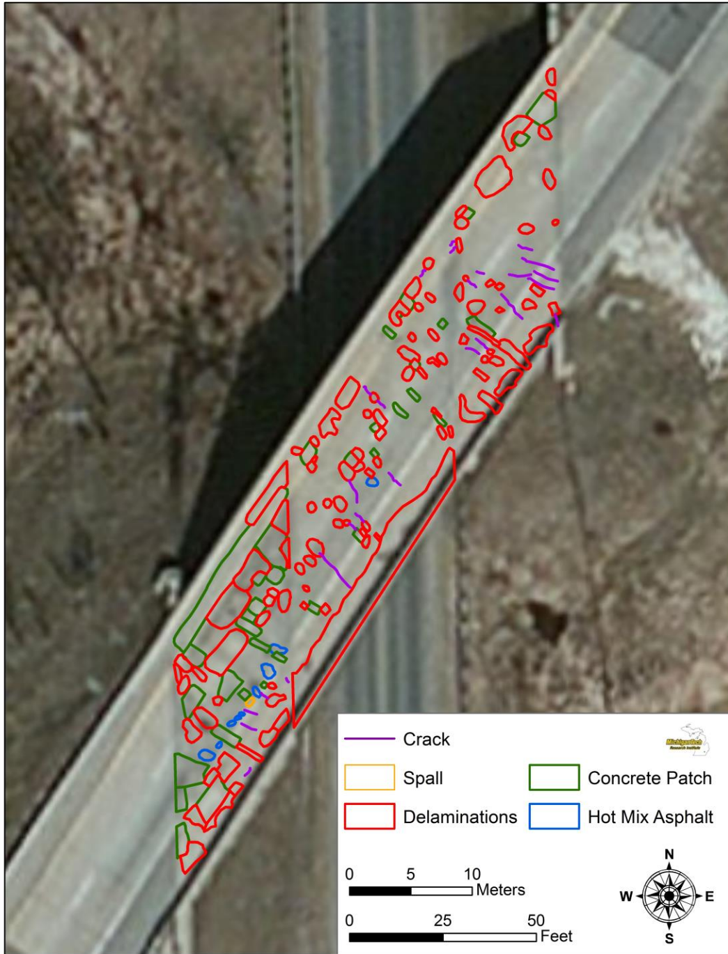
Figure 4-10: Georeferenced Sketch of the Results of the Deck Sounding of the North Bound Bridge of US-131 Showing the Locations of Delaminations, Cracking and Spalls.
