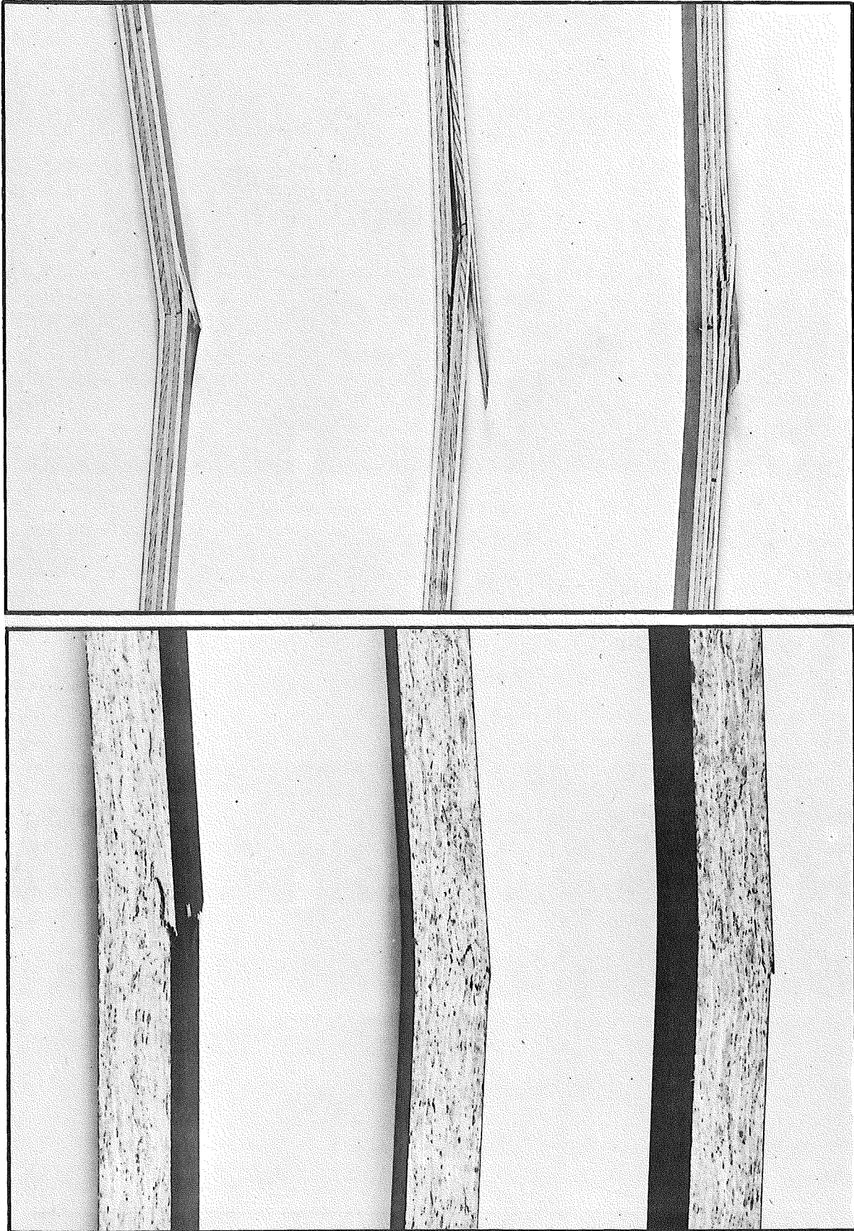
Figure 4. Typical static bending test failures of dry-condition specimens, with fiber board at left, and plywood at right.
