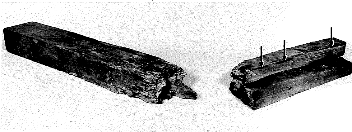
Figure 3 (below). Two parts of decayed post (Sample 63 MR-288); arrows indicate darker areas which show very little penetration of preservative into the wood.
