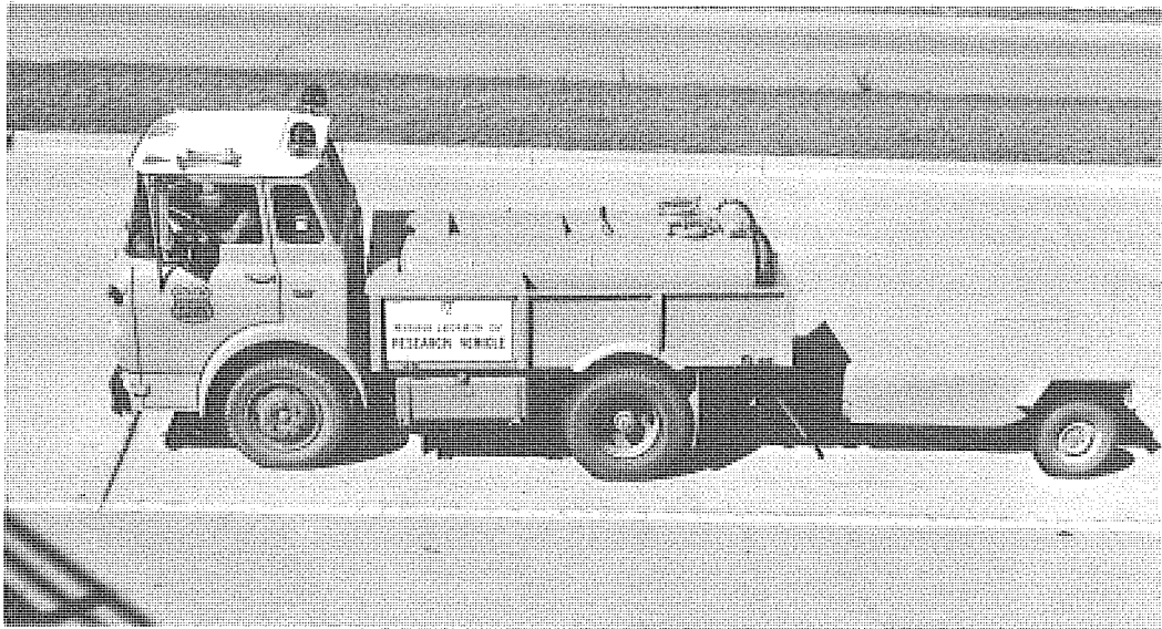
Figure 1. Tow vehicle and skid trailer.
