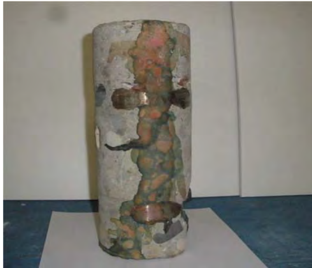
Figure 6-7 63174-S05-1 carrying I-75 NB over 14 Mile Road core exposed to Rainbow Indicator
