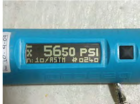
(d) Reading showing the compressive strength after 10 impacts
