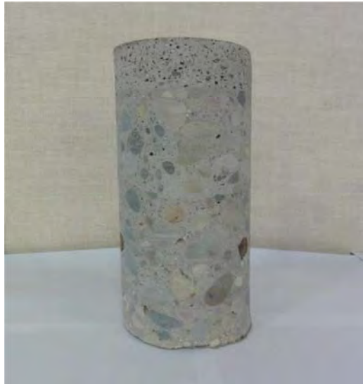
(d) Concrete core taken from bridge deck
