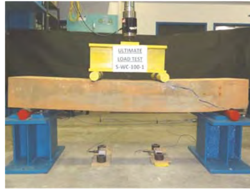
(b) Flexure/shear mode
