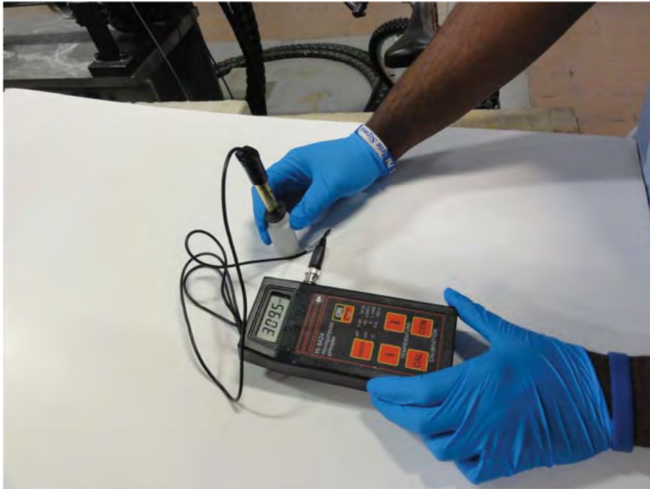
Figure 4-16 Voltage reading (mV) of concrete powder solution
