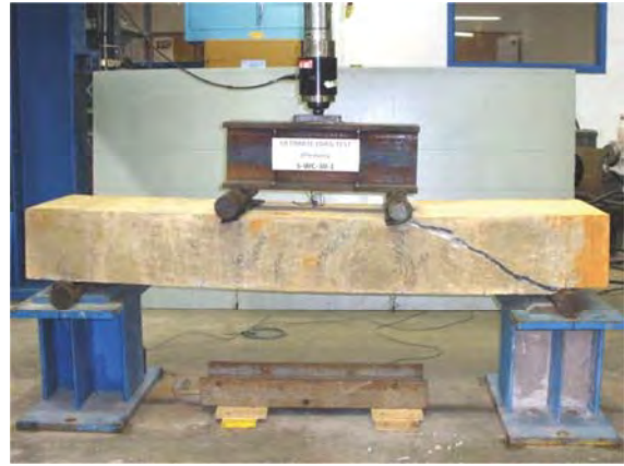
b. Flexure/shear mode of failure
