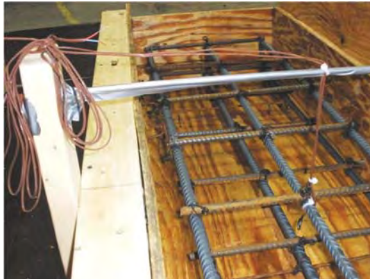
Figure 3-7 Thermocouples located at core of the specimen before casting concrete
