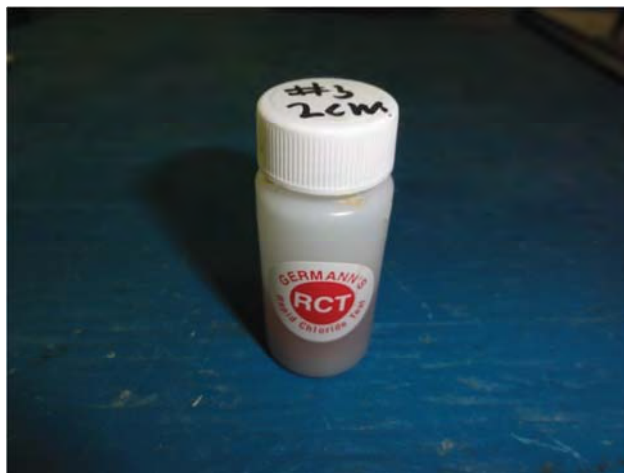
Figure 4-15 Concrete Powder sample mixed in the extraction solution
