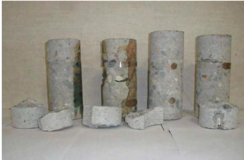
Figure 4-23 63174-S05-1 carrying I-75 NB over 14 Mile Road cores
