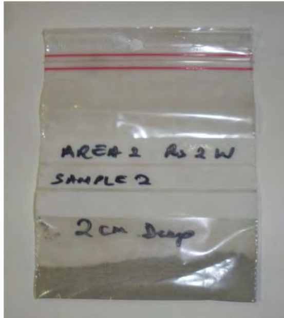
Figure 4-12 Concrete powder taken from Area A2 at 2 cm depth from the bottom
