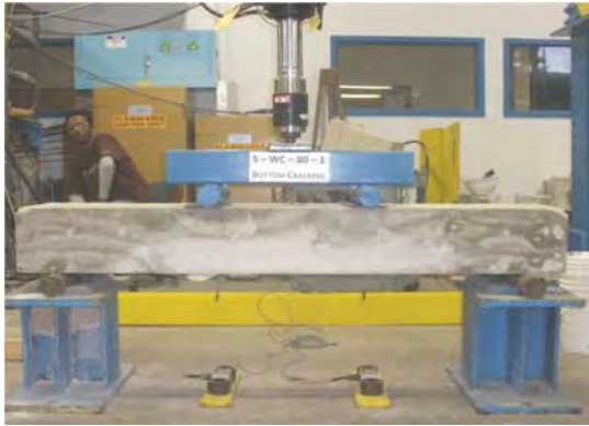
(a) Actuator applying load on the specimen
