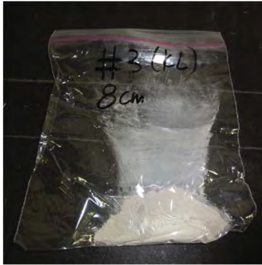
Figure 4-14 Concrete powder taken from core at a depth of 8cm
