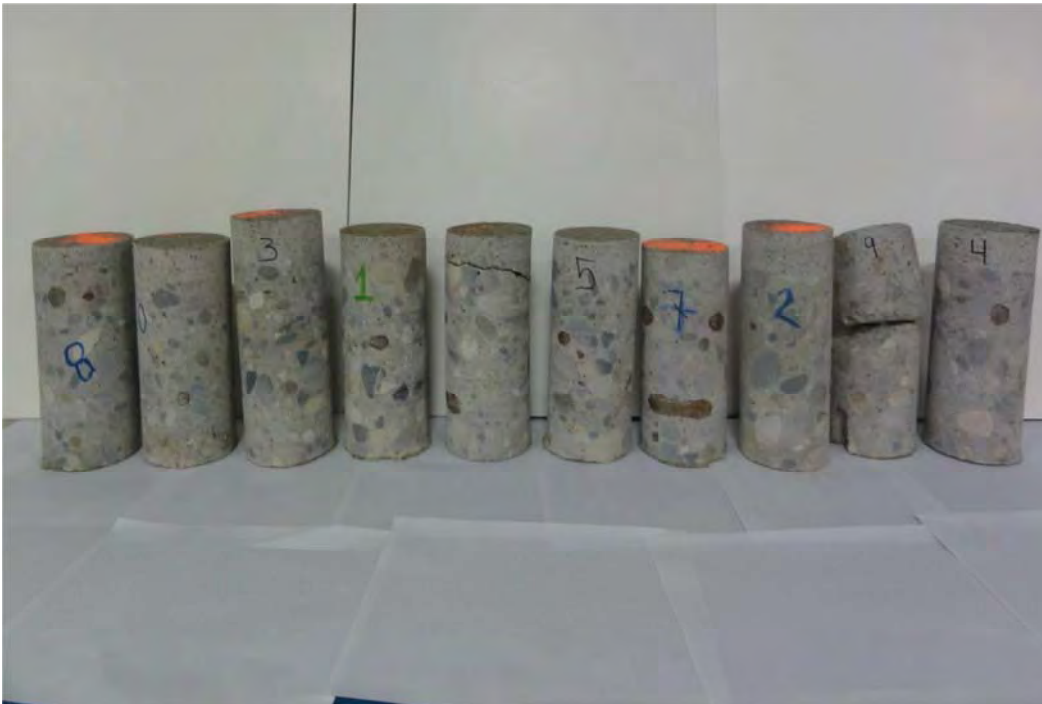
Figure 4-34 63022-S01 carrying I-96 over Kent Lake Road cores (Cores 1, 2, 3, 7, 8, 9 and 10 were from the right lane; Cores 4, 5 and 6 were from the interior shoulder)
