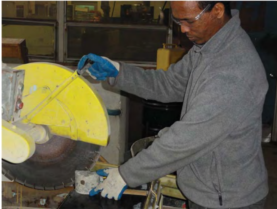
Figure 3-31 Sample preparation of bridge cores taken during field sampling.
