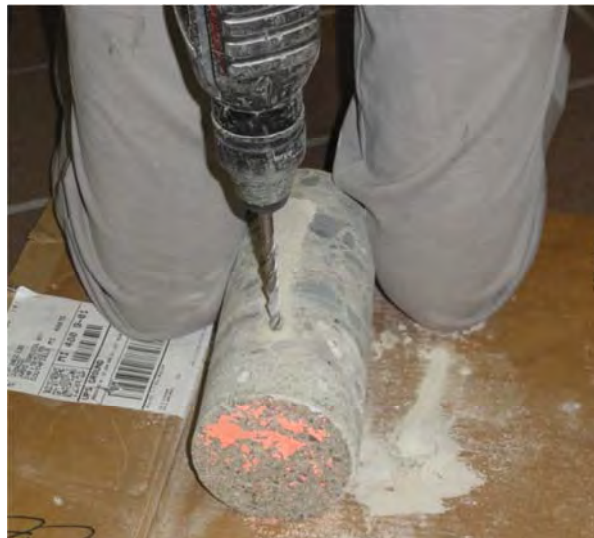
Figure 4-13 Collecting of concert powder from full depth of cores
