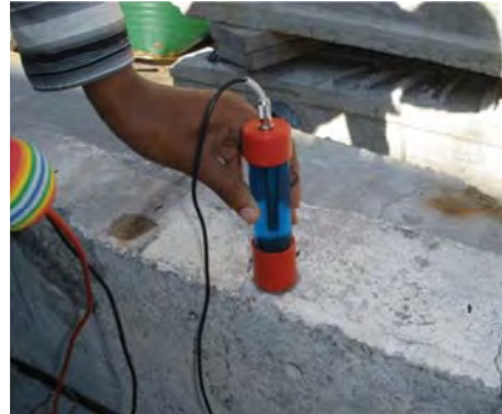
(b) Placing rod electrode against concrete surface
