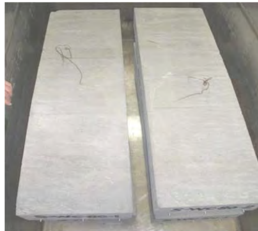
(b) Final arrangement of specimens before filling tank with saltwater
