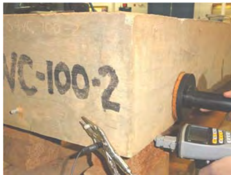
(c) Measuring corrosion rate
