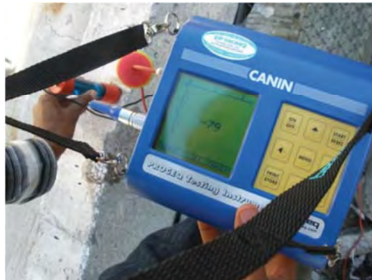
(c) Measuring potential using CANIN
