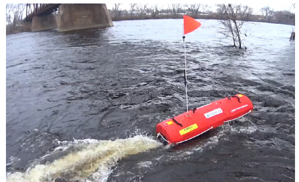
A remote-controlled USV equipped with a sonar unit can maneuver around bridge piers and abutments during a high-flow event.
