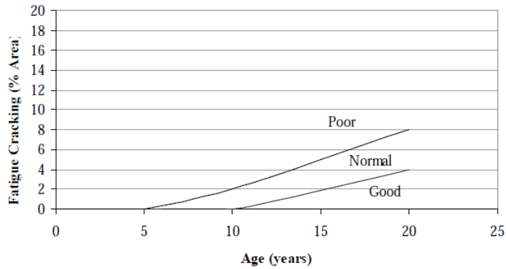
Figure 4-11 Pavement performance criteria for fatigue cracking (6)
