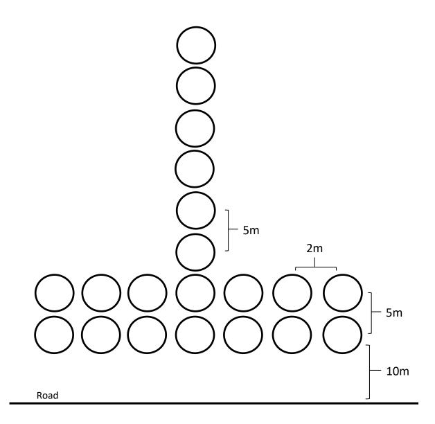
**APPENDIX F**. Temperature logger (iButtonLink Technology model DS1921G-F5# Thermochron 4k) pair orientation above- (soil surface) and belowground (0.15 m subsurface). Temperature loggers were sealed in plastic zipper bags. A brightly colored flag was attached to the surface temperature logger bag for relocation. If in the road right-of-way the flag was bent parallel to the ground (pictured above) to avoid disrupting maintenance activities.
