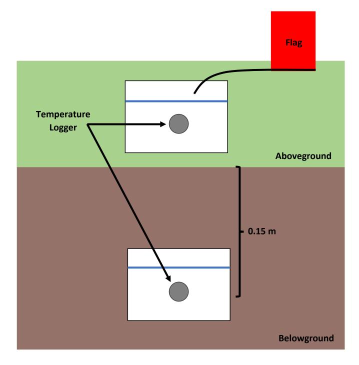
**APPENDIX G**. Temperature logger (iButtonLink Technology model DS1921G-F5# Thermochron 4k) pair orientation above- (soil surface) and belowground (0.15 m subsurface). Temperature loggers were sealed in plastic zipper bags. A brightly colored flag was attached to the surface temperature logger bag for relocation. If in the road right-of-way the flag was bent parallel to the ground (pictured above) to avoid disrupting maintenance activities.
