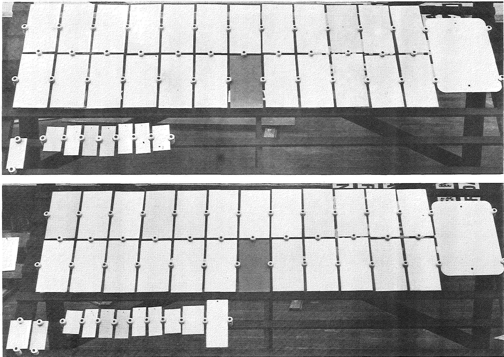
▲ FIGURE 2. (TOP) WEATHER RESISTANCE EXPOSURES. INITIAL CONDITION, MARCH 27, 1956. (BOTTOM) WEATHER RESISTANCE EXPOSURES. DETERIORATION, SEPTEMBER 1, 1956
