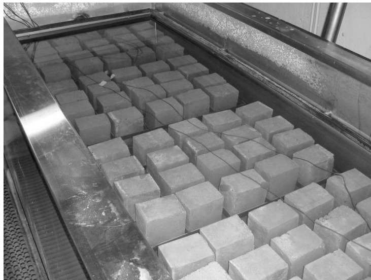
Figure 3-13: MTU 80-specimen Freeze-Thaw Chamber (Procedure B)
