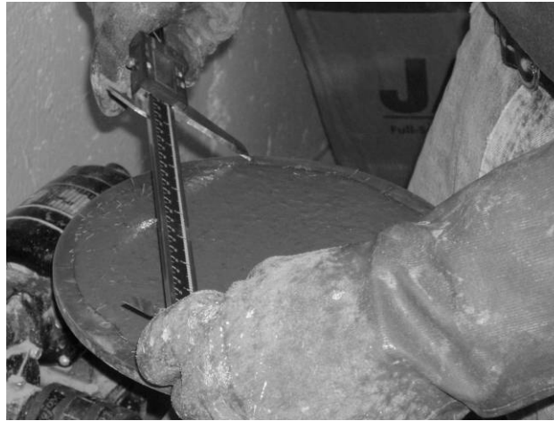
Figure 3-3: Impact Table Measurement of UHPC's Flow
