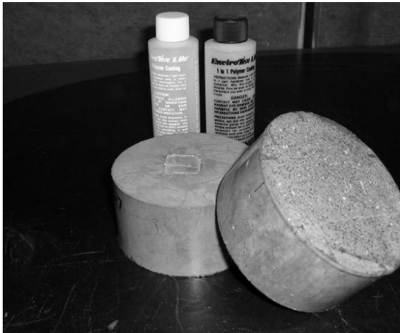
Figure 3-10: Epoxy-coated UHPC Specimens for RCPT
