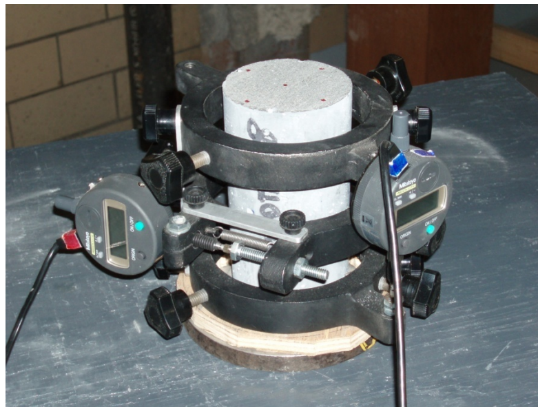
Figure 3-8: Compressometer and Extensometer
