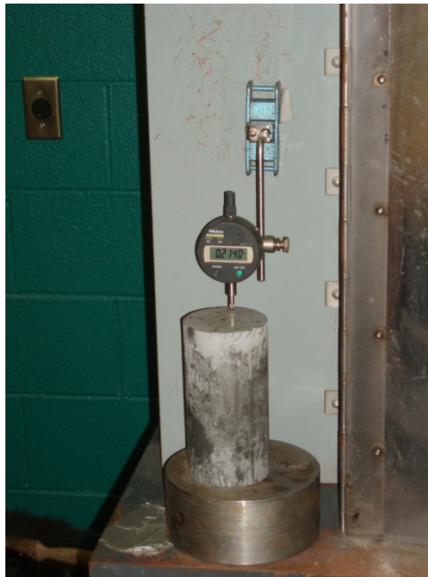
Figure 3-6: End Perpendicularity Set-up
