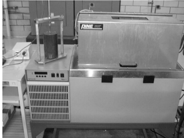
Figure 3-17: Pine CTE Specimen Test Frame and Water Bath
