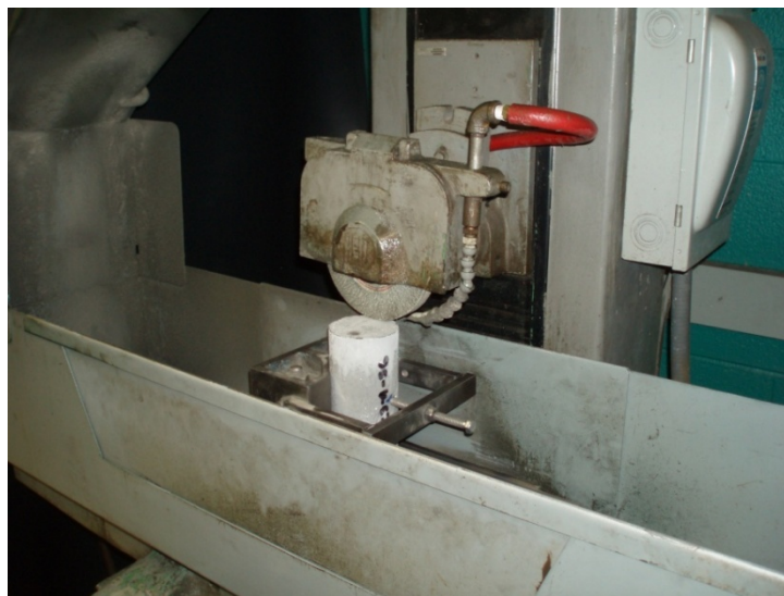
Figure 3-5: Reid Surface Grinder
