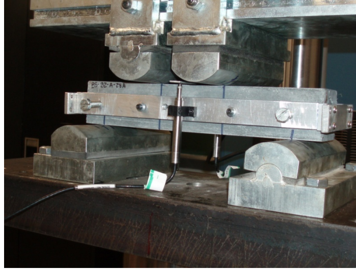
Figure 3-9: ASTM 1018 Loading Configuration
