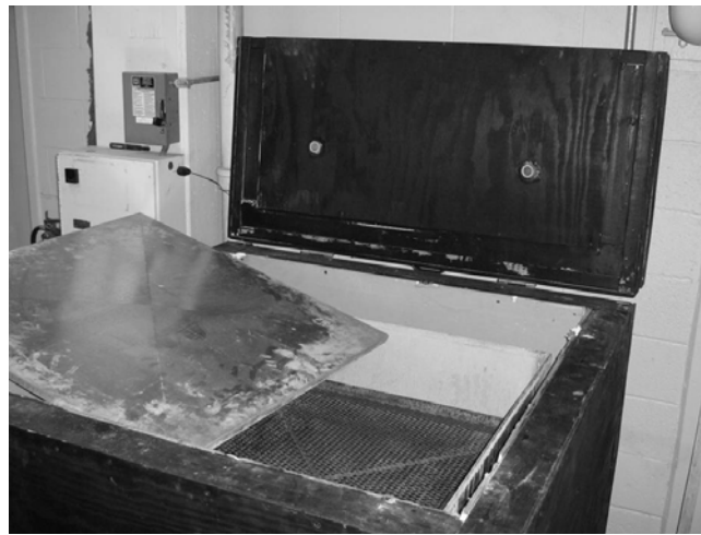
Figure 3-4: Michigan Tech’s UHPC Thermal Treatment Cure Chamber
