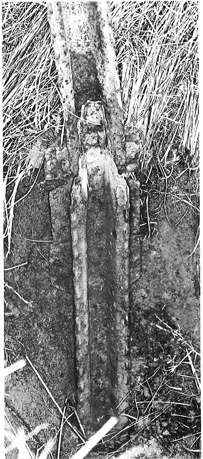
Figure 21. Age: 28 years. North side of US 16 about 4 miles east of Hogback Road and 1 mile west of M 59 intersection. Clay soil with some loam. Corroded completely through at ground line with severe corrosion above ground. Yellow paint still present below ground level. Three or four spots where paint has come off show shiny black metallic surface. Some corrosion under ground.
