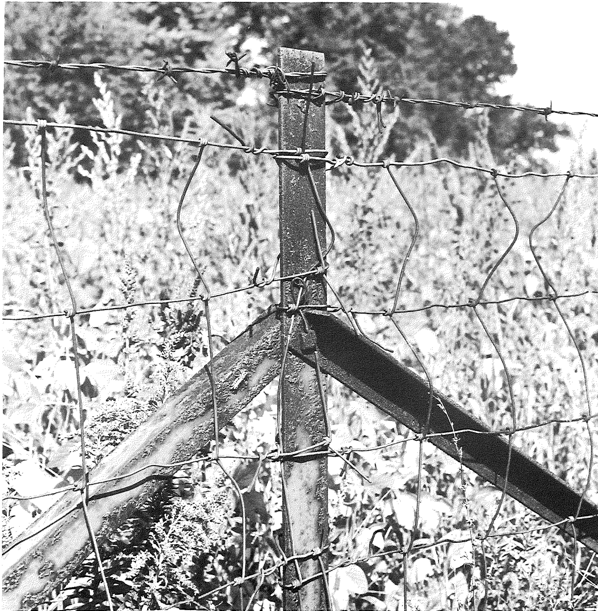
Figure 6. Age: 5 years. West side of I 75 at Station 1357+00 south of Vreeland Road between Detroit and Monroe. Two views of severe corrosion of intermediate braced post with several instances of galvanic corrosion of fencing wire.
